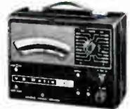
Has same automatic scale features as VTVM. No multiplying, no false readings. Features burn-out proof meter movement. Sensitivity is 20,000 ohms/V,DC; 5,000 ohms/V,AC. Ranges from 0 to 6000 Volts plus supplemental ranges. Complete with batteries and test leads.
