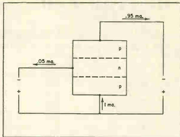
Fig. 8: Circuit current gain  $\alpha/(1-\alpha)$
