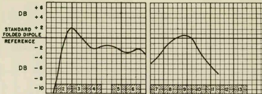
Fig. 2: Gain of a simple dipole (90" long) and reflector over the 12 channels, compare to "standard" cut for each frequency. Compare this broad-band, low-gain antenna with the narrow-band, high gain Yagi shown in fig. 3. Illustration courtesy American Phenolic Corp.
