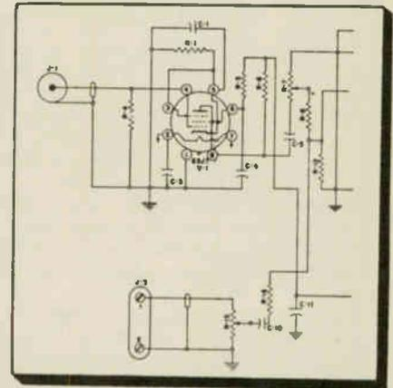
Fig. 2: Stromberg Corison amplifier AU29 uses a 6SJ7 for mike input (J-1). J-3, the phono input, feeds the second stage. Circuit components are chosen for slightly lower element voltages on the tube and consequently slightly lower gain than the stage in fig. 1, which must handle the extremely low output tape head.
