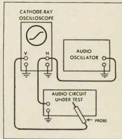
Fig. 3: Arrangement for estimating both frequency and amplitude distortion at a glance, making it easy to monitor oscillator output for uniform input to the device under test.
