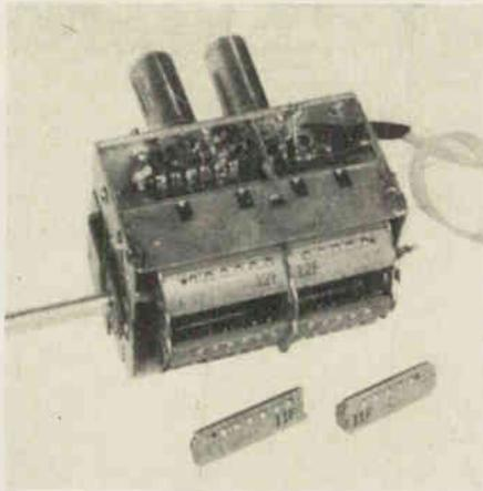
CAPEHART-FARNSWORTH—Using a regular Capehart CX-33 receiver chassis, four miles from the Bridgeport transmitter ultra-high-frequency conversion was accomplished by inserting UHF channel strips in Standard Coil tuner already a part of instrument. Complete Capehart line uses same chassis.
