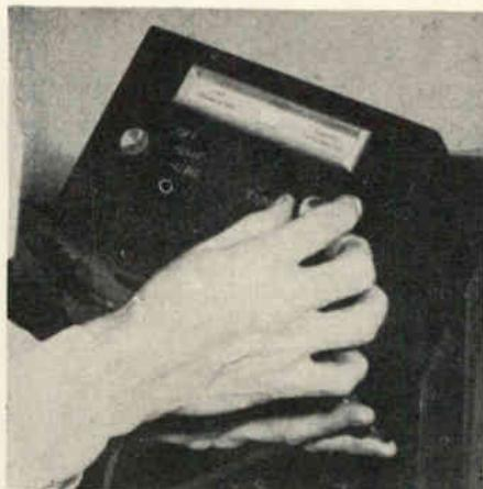
**TARZIAN**—Full-band UT-1 tuning unit for ultra-high-frequency telecasts is adaptable to any set now in use; does not interfere with VHF channels. Self-contained power supply. No electrical changes are necessary in present television sets. Unit may be placed on top of the set or installed inside.
