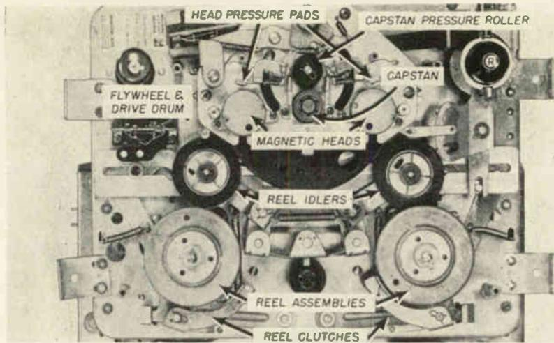
Fig. 3. Instantaneous dual track design of Webcor recorder uses symmetrical setup of reel assemblies, drive idlers and heads, which function both in play-record and erase.
