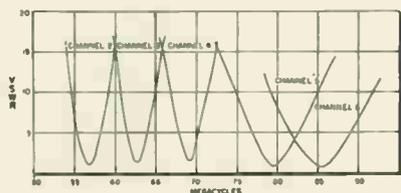
Fig. 5: SWR for low VHF band positions
