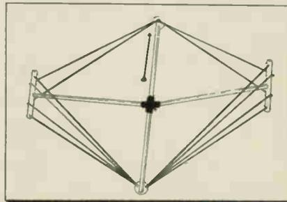
Fig. 6—An unusual rhombic in which the long axis is broadside to the station. Extra elements on the back are designed to improve pickup on the low band. By increasing the diameter of the elements, it is said to be possible to utilize shorter legs.—Courtesy Roger Phillips Research Labs.
