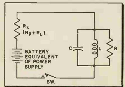
Fig. 4—Ringing circuit with shunt resistance.
