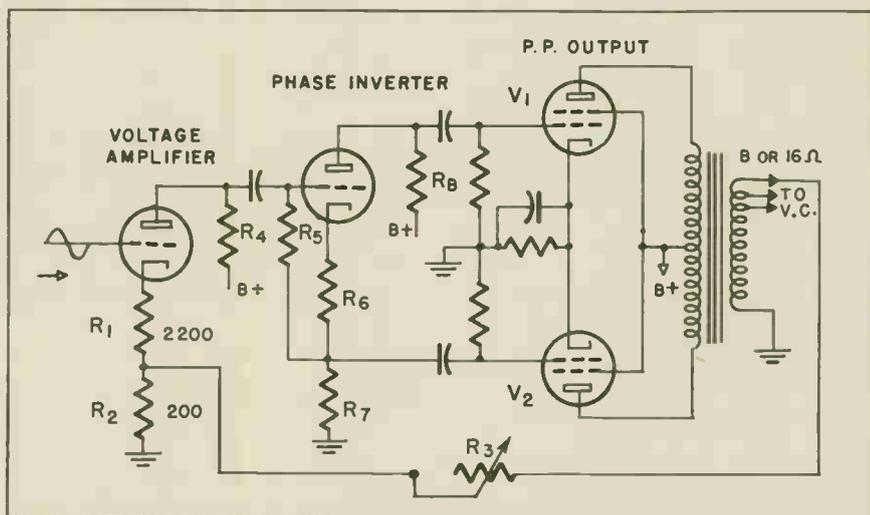
Fig. 1. In adjusting inverse feedback  $R_3$  is a variable potentiometer.  $R_1$  and  $R_2$  may vary. Some designers recommend omitting  $R_2$  and connecting  $R_3$  to cathode.  $R_7$  equals  $R_6$ .
