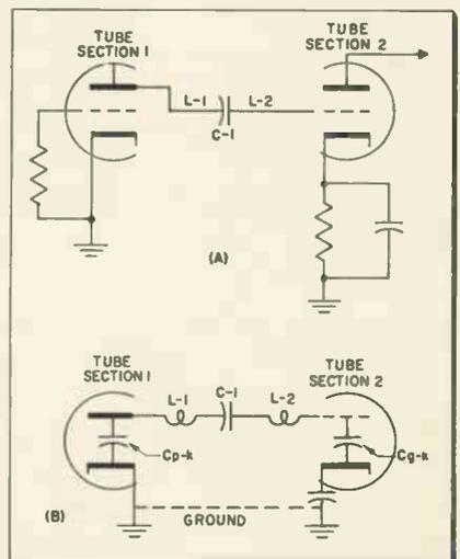
Fig. 5A—Section of sync circuit. B—Parasitic circuit of (A).  $C_{p-k}$  and  $C_{g-k}$  are the plate-cathode and grid-cathode capacitances.
