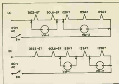
Fig. 2A—Connection of 2 ac voltmeters across tube filaments for first fading check. B—Voltmeter connections for the second fading check.
