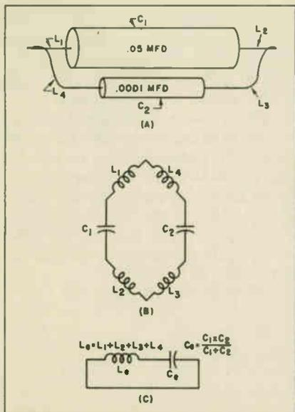
Fig. 1A—Capacitors in parallel, together with their lead inductance, may make up a parasitic resonant circuit. B—Elements of the parasitic circuit, schematically shown. C—Simplified, equivalent L-C series resonant circuit. Effective inductance is represented by  $L_c$ ; effective capacitance is represented by  $C_c$ .
