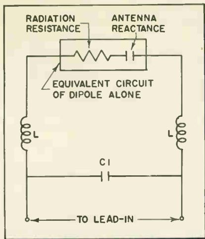
Fig. 3: Simplified circuit of matching network
