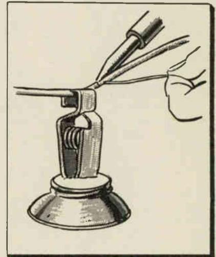
letting the lead (or solder) solidify while the end of the battery clamp is held in it. This "third hand" is a good item to carry along in the tool kit for those outside calls, too. M. Quisenberry, Bucks Radio & Appliance Co., Lexington, Va.
