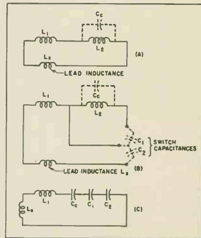
Fig. 4A—Coil inductance ( $L_1$ ) in series with parasitic capacitance ( $C_c$ ) of a 2nd coil ( $L_2$ ) and the lead inductance ( $L_2$ ). B—Basic circuit of (A), in series with, and completed by, capacitance introduced by switch contacts. C—Equivalent of one of the parasitic circuits in (B). Several others are possible.
