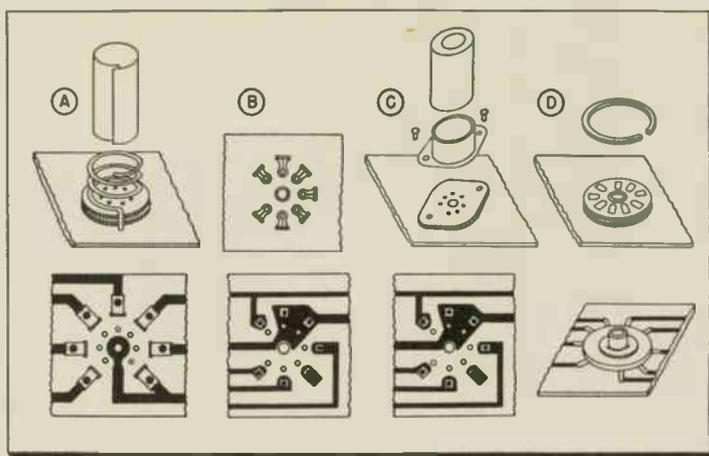
Fig. 2: (L) Pasteboard models for visual study of various shapes. Fig. 3: (R) Design sketches of dip-soldered assemblies incorporating tube sockets
