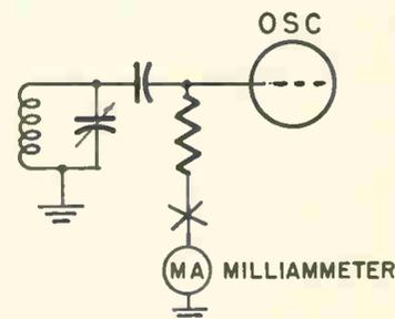
Fig. 4—Measuring grid voltage of oscillator with milliammeter. The circuit is opened at the ground side of the resistor (X), and the meter inserted as shown.
