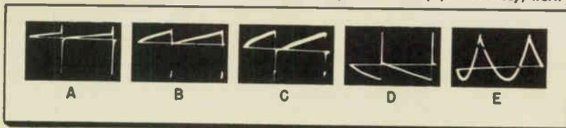
Fig. 4—Waveforms and their amplitudes in the circuit of Fig. 2 (preceding page). Numbers under the waveforms refer to the circuit points in Fig. 2 at which the waveforms were obtained.
