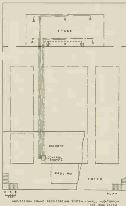
Fig. 1: Auditorium sound reinforcing system with 2 speakers and 4 mikes on stage.—Courtesy RCA.
