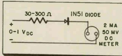
Fig. 9: Where meter protection from high reverse voltages is desired, a diode may be connected so the reverse current is limited to 3 ma with negative 30 v applied in place of the normal positive 0-1 v. The 30-300 ohm resistor is adjusted to calibrate the meter to 1 v full scale. The normal uniformly divided scale of the meter will be changed by the addition of the diode to one with the divisions contracted near the zero and approximately shown below:
