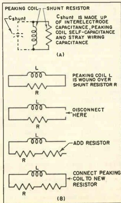
value—do not excessively over-damp one coil circuit alone, in order to get by with only one resistor.
