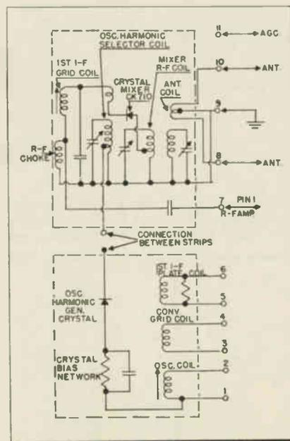
Fig. 2—A UHF strip circuit. (see text)
