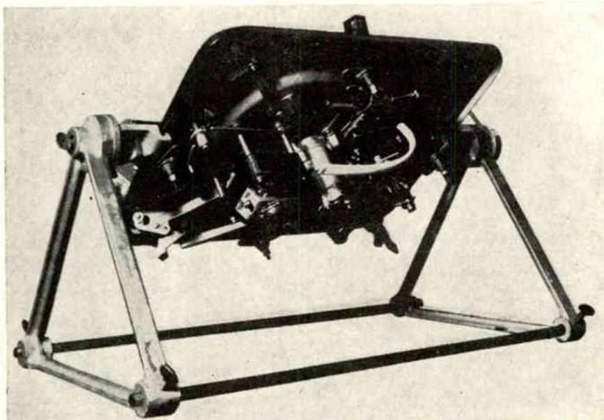
Mounted on adjustable changer rack for easier, faster repair is a Garrard 3 speed changer.
