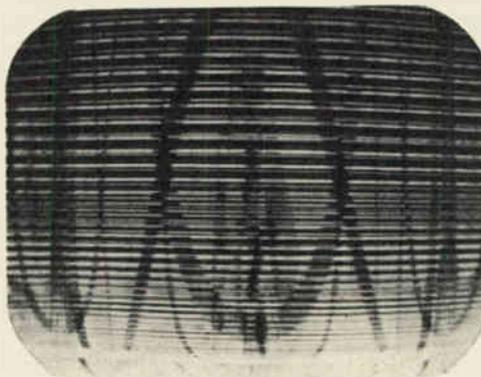
Fig. 6—Excessive height. Sweep is so great that the horizontal scanning lines are pulled apart. Severe leakage in the coupling condenser between vertical oscillator and amplifier may cause this.
