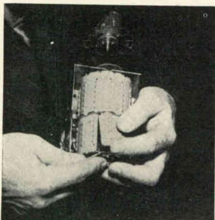
**STANDARD COIL**—Simple transfer of strips in tuner, readies any set so equipped, for reception of uhf signals within a few minutes. The two-section strips in effect turn TV set into a double conversion circuit. CK 710 diode is used as converter. Fingers shown belong to Edwin Thias, engineering VP.
