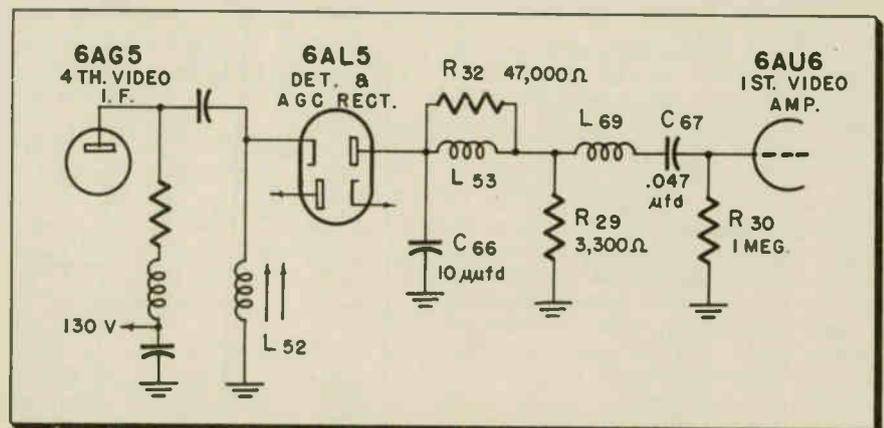
Fig. 1—Video detector circuit used in Philco 50-T1443. Filament circuit is not shown.
