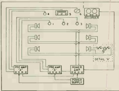
Fig. 2: Wiring diagram for auditorium reinforcement system similar to fig. 1. Placement of mikes and speakers is described in text.
