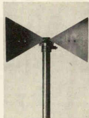
Fig. 4: Fan dipole
