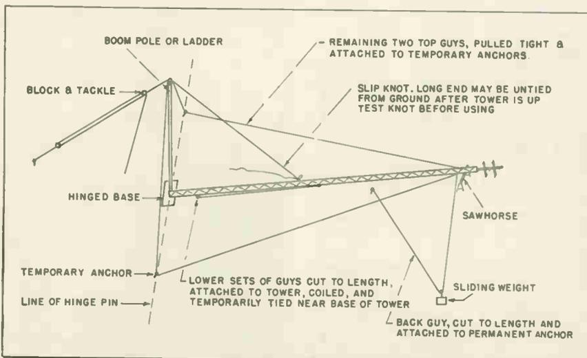
Fig. 5: The complete installation. A separate conductor should be run to a good ground for lightning protection. Grounding a guy wire endangers the mast, should that guy wire be damaged by lightning.
