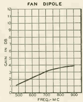
Fig. 5: Fan dipole gain
