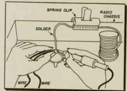
The drawing shows how I use a spring clip as a third hand to hold the solder in exactly the right position.—J. Amorose, Amorose Radio, Route 4, Hungary Rd., Richmond, Va.
