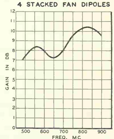
Figs. 7-10: (Left) Physical appearance of two-stacked (left) and four stacked fan dipoles. (Above) Gain vs frequency for the two types
