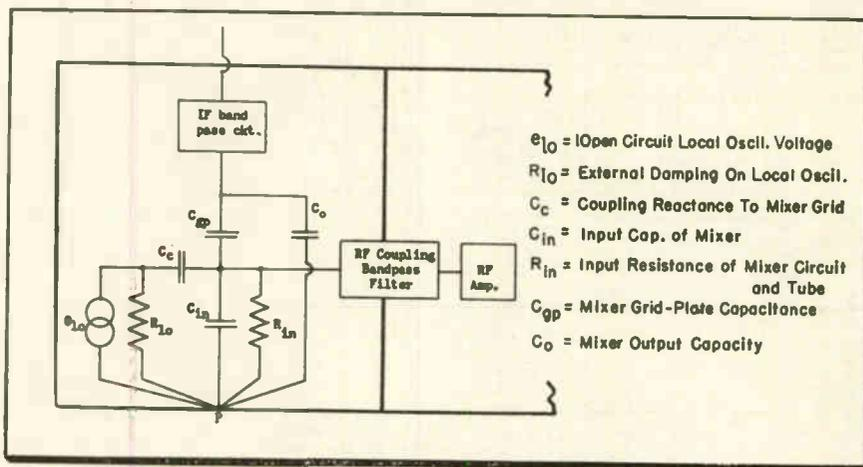
Fig. 1: Shielded local oscillator equivalent circuit. R-F and i-f bandpass filters introduce sufficient attenuation at local oscillator frequencies to make their ground returns relatively unimportant
