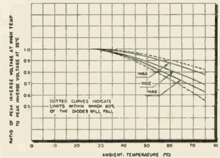
Fig. 19: Typical peak inverse voltage-temperature ratio characteristics with respect to 25°C.
