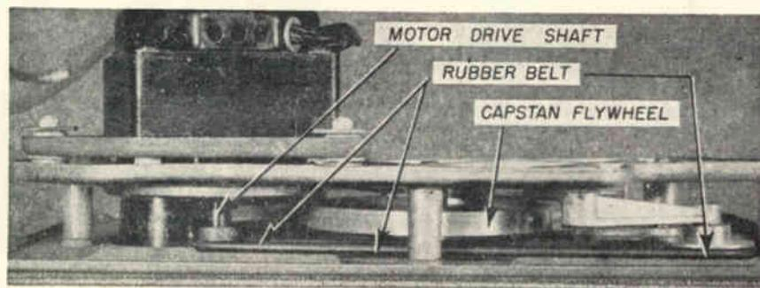
Fig. 2. In the Eicor mechanism above is shown the rubber belt which transmits motor force to takeup reel and capstan. Maintenance of proper belt tension and friction is important.
