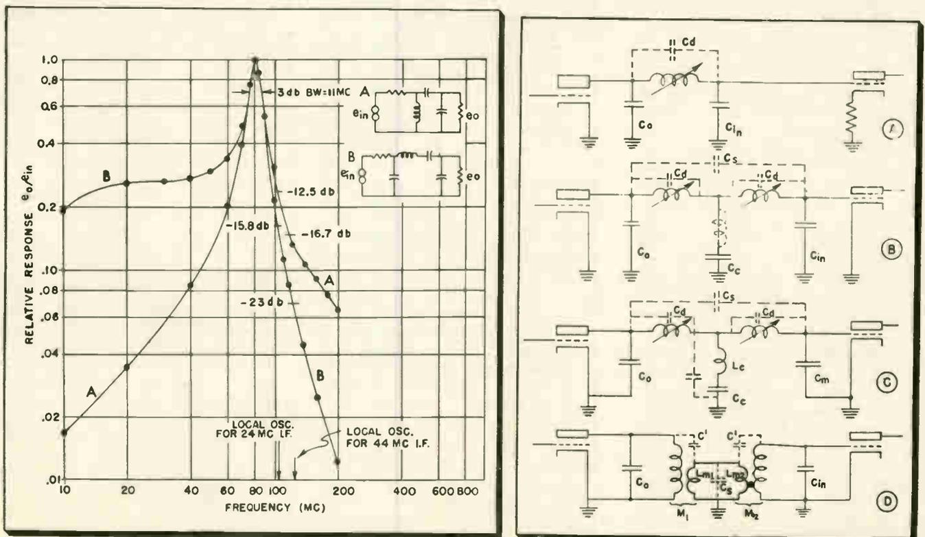
Fig. 8: (L) Comparison of selectivity of anti-resonant circuit (A) with high selectivity input (B) shows greater attenuation of (B) prevents reverse transmission of LO frequencies through r-f stage. Fig. 9: Mixer bandpass couplings circuits, stray reactances dotted.
