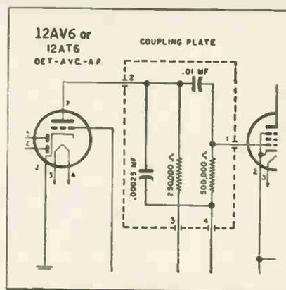
next stage, it will be seen that ordinarily *eleven* various points and *five* components would have to be connected together with *eight* or more soldering and twisting operations. With the printed circuit unit this is reduced to five soldering points, and *one* component.
