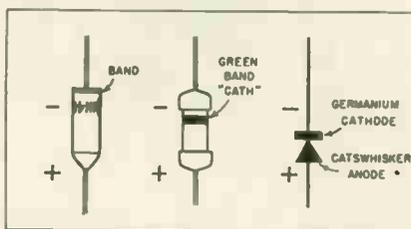
Fig. 3: Proper polarity indications for germanium diodes.
