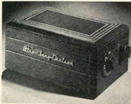
**STROMBERG-CARLSON'S** converter, styled in green leatherette and measuring only 8x4x6 in., uses a 6F4 as a local oscillator, a 6BQ7 as a cascode r-f preamplifier, and a 1N72 germanium crystal mixer. Unit has a 12MC bandwidth and balanced output feeds VHF-TV channels 5 or 6.
