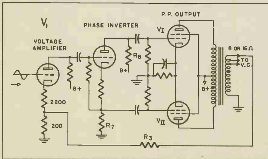
set, so an additional triode stage must be added to compensate for the loss.
