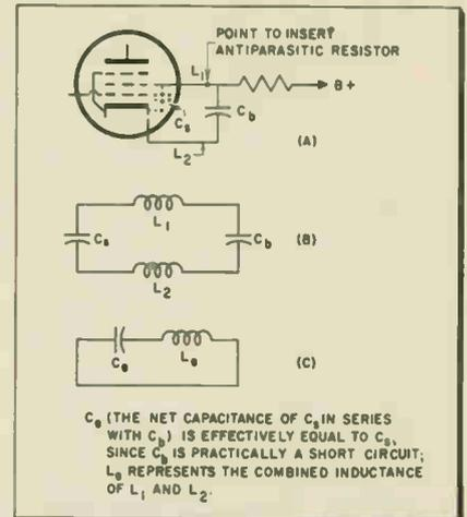
Fig. 2A—Partial schematic of a stage, showing location of bypass ( $C_b$ ) and interelectrode ( $C_a$ ) capacitances; also stray inductances ( $L_1$  and  $L_2$ ). B—Parasitic elements of circuit shown in (A). C—Simplification of circuit shown in (B).  $C_c$  and  $L_c$  are the effective net capacitance and inductance, respectively.
