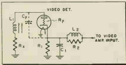
Fig. 3—Basic video detector circuit. C<sub>p</sub> is the plate-to-cathode capacitance. R<sub>x</sub> is the DC resistance of coil L-1. It is not actually a separate resistor, although it is represented as one.
