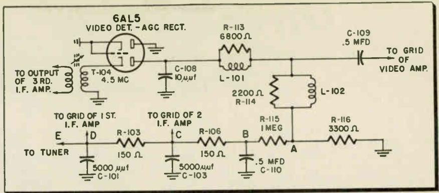
Fig. 1—Simple AGC circuit, in which video detection and AGC rectification are performed by the same diode. Elements of the unused diode are grounded out. The circuit shown is from the schematic of Hollicrafters Models 810A, 815, 822, 870, 871 and 880.
