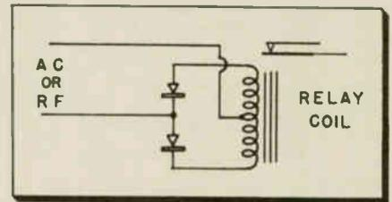
Fig. 11: Good 400-800 cycle relay operation has been obtained using a center tap brought from the relay coil with three wires connected to the diodes as shown. In this circuit the flux is held constant over both halves of the ac cycle. Greater freedom from chattering and increased sensitivity result from this arrangement.
