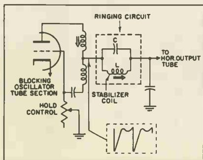
Localization of, and remedies for, this type of fault have been considered in a previous article. Barkhausen-Kurtz oscillations may also produce similar symptoms. A magnet moved about the horizontal output tube will eliminate, and thus serve as a check for, this source of trouble.
