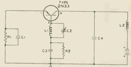
Fig. 3—50 MC oscillator circuit using a point-contact transistor.
