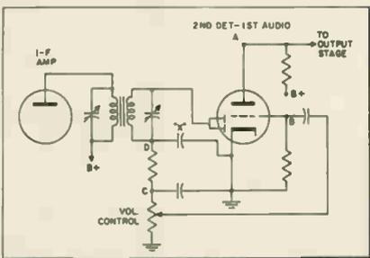
Fig. 1—i-f and second-detector circuit of 5-tube ac-dc receiver. Intermittent open-circuiting of condenser "X" resulted in fading.
