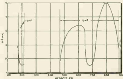
Fig. 6: SWR for high band VHF and UHF
