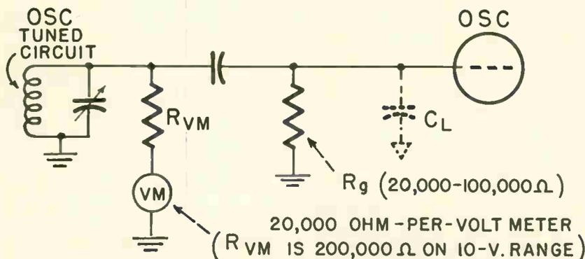
Fig. 2—Using a voltmeter with a relatively low input resistance will load down the tank circuit. If  $R_g$  is 100,000, and  $R_{vm}$ , the internal resistance of the meter, is 200,000, the effective value of  $R_g$  becomes about 67,000 ohms.
