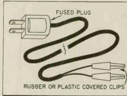
grips to protect the technician from shock and to keep the clips separated when they are used on terminals which are close to each other. This sort of cord can be used as a universal test cord for TV sets, particularly in the case of older sets such as GE, Philco, Emerson, which for some years had an AC interlock receptacle differing from what has now become standard for the industry.—Arthur Bertram, 247 West 15th St., New York, N. Y.
