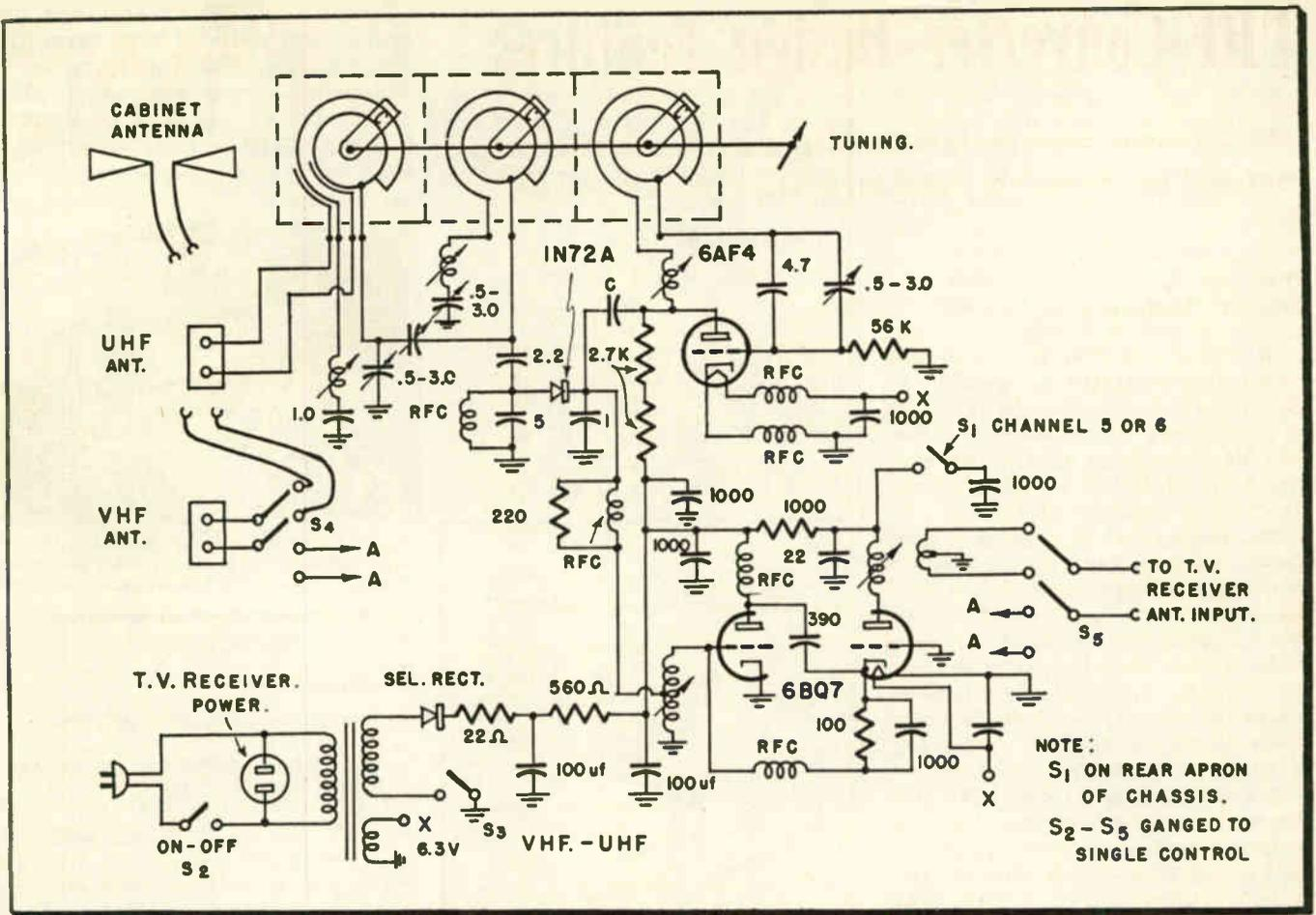
Fig. 5: Schematic diagram of the Stromberg-Carlson UHF-Converter
