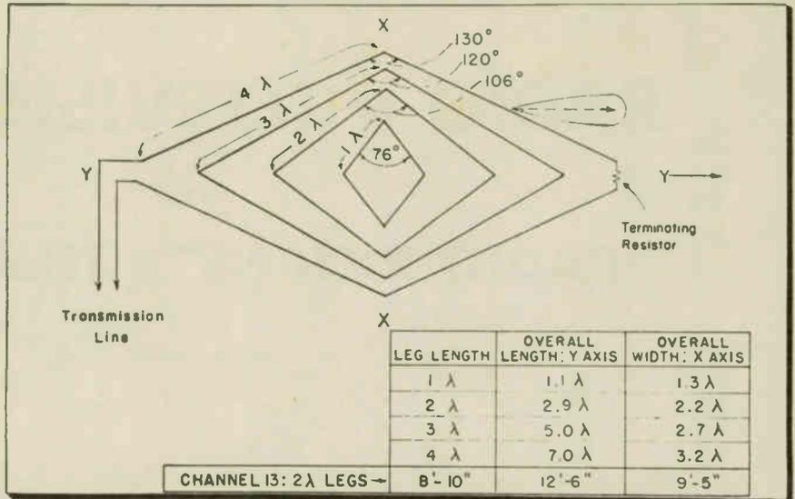
Fig. 2—Typical rhombic designs based on interior angles which complement those shown in fig. 3. When the legs or sides are larger multiples of a wave length at the operating frequency, the antenna gets longer and narrower as does the beam, and the gain goes up. Similarly, when the size remains the same but the frequency goes up: a leg which is  $2\lambda$  long at 100 MC is  $4\lambda$  at 200 MC.
