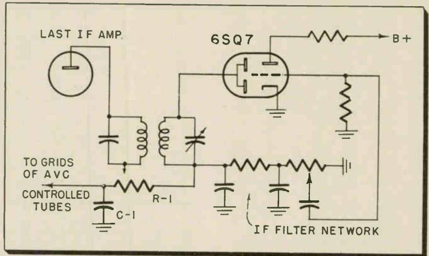
Fig. 2—Typical AVC circuit used in broadcast AM receivers.
