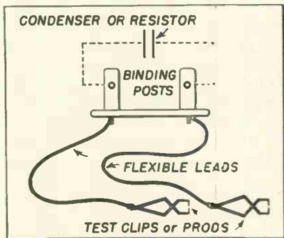
or resistor in a circuit momentarily to test the part in question. The usual method is to hold the substitute in your hand, or tack it in with a soldering iron. The test fixture shown enables the servicer to insert a condenser or resistor between two bind-
