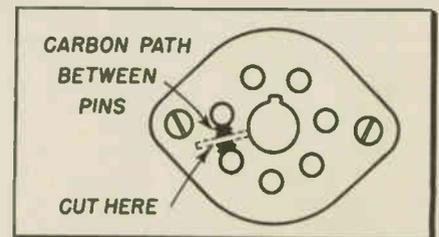
can be devised. So I used a key-hole hack saw to cut a slot from the center key of the socket to the space between the pins.
