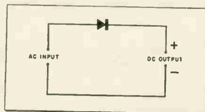
Fig. 4: Output taken from cathode (minus) end of diode.
