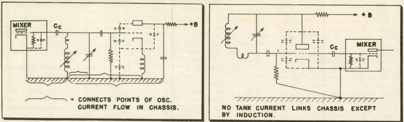
Fig. 5A: (L) Poor oscillator design causes conduction currents in chassis. Fig. 5B: (R) Good oscillator design reduces chassis currents
