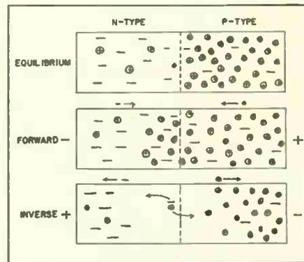
Fig. 4: Rectification by a P-N Junction
