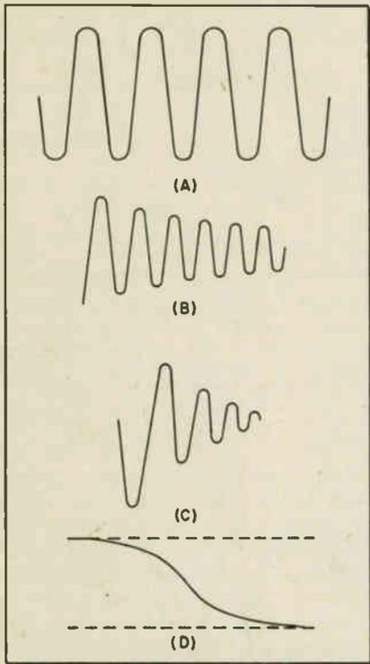
Fig. 3—Waveform of a ringing circuit when the latter is (A) undamped, (B) slightly damped, (C) heavily damped, (D) over-damped.
