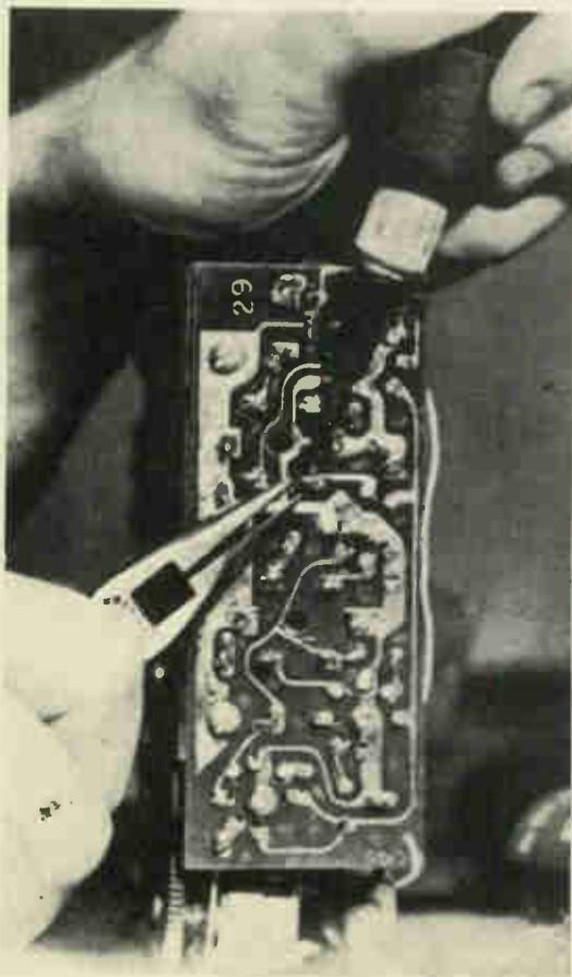
Several types of etched-metal, embossed-circuit and printed-circuit sets exist. In the true printed-circuit receiver, the wiring is electroplated on a layer of conductive (metallized) ink, printed on a sheet of phenolic plastic material, and deposited by a printing or silk-screening process. The bond between the chassis and wiring is very delicate, and special care is therefore necessary during servicing.
