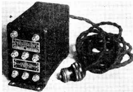
Fig. 9.—A typical filament heating transformer suitable for heating the filaments of the tubes in the conventional type of electric set. The two binding posts at the top give 1\frac{1}{2} volts. The middle row, 2\frac{1}{2} volts with a center tap and the lower row, 5 volts with a center tap. The size can be judged by comparing it with the electric plug beside it.
