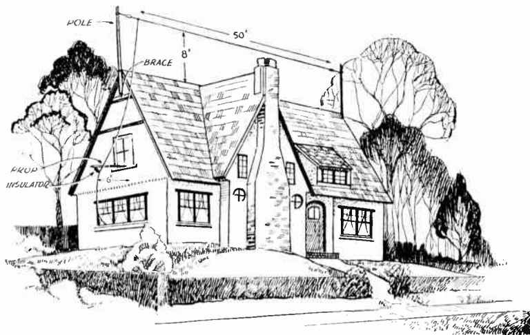
Fig. 20—How to install an aerial for the suburban home which will not be considered detrimental in point of appearance.
