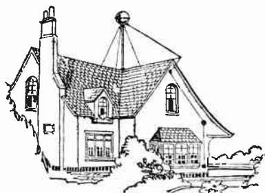
Fig. 6—Ball antenna installed on suburban home.
