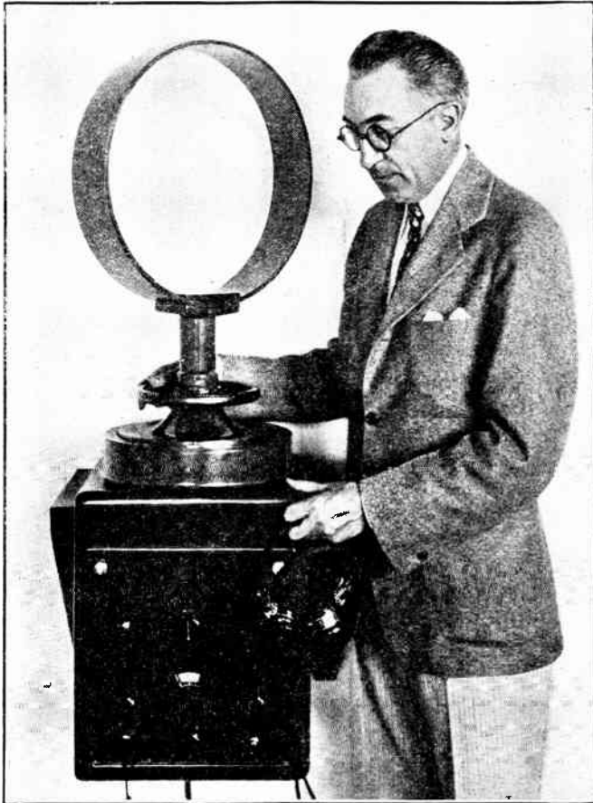
Fig. 16-A—Dr. F. A. Kolster, Inventor, Inspecting an Installation of a Small Radio Compass on a Sea Skiff.
