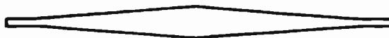
Fig. 14—A type of diaphragm made of a non-magnetic material, the thickness at the center being greater than at its edges.
