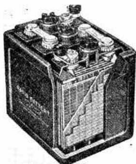
Fig. 16—Cross-section of Lead plate Storage Battery.
