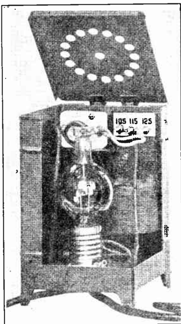
Fig. 6—General Appearance of a Commercial One Tube Rectifier with Two Sides and Top Removed.
