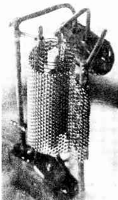
Fig. 5.—A photomicrograph of the electrodes of the type 227 A. C. heater tube (three times full size) taken through the glass of the tube. Note the wire screen plate, the spiral grid wire, the white, porcelain-like cathode insulator, at the top of which you can see the heater filament where it passes from one hole in the insulating tube to the other one.
