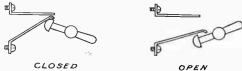
Fig. 5.—Sketch Illustrating Action of Filament Switch.
