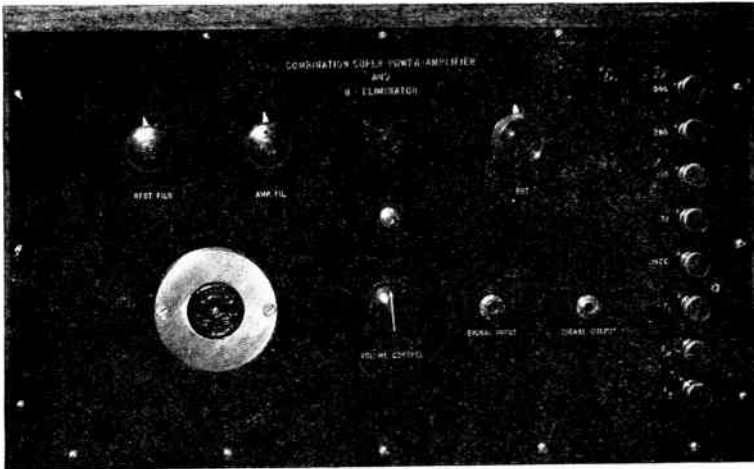
Fig. 10—Panel of Super-Power-Amplifier, Showing the Various Controls and Binding Posts.
