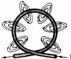
Fig. 4—Magnetic field about a single loop carrying current.
