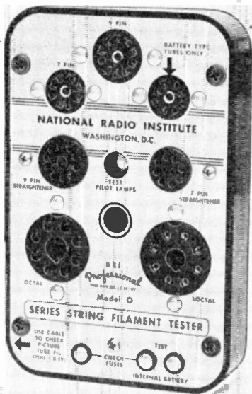
FIG. 11. The NRI Professional filament checker shown above can be used to quickly locate a tube with an open filament in a series filament string.
