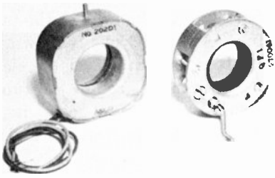
FIG. 16. A typical focus coil is shown at the left, and a permanent-magnet focusing device at the right.
