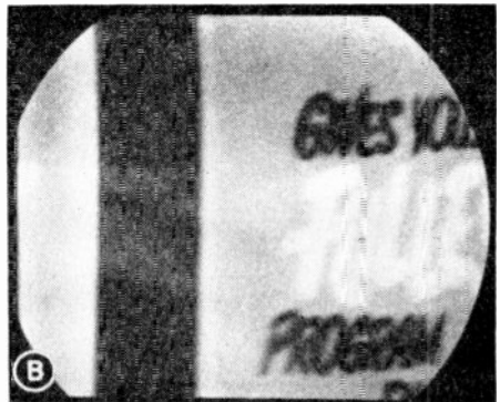
FIG. 9. Two forms of horizontally unsynchronized picture: (A) horizontal frequency off; (B) out of phase.
