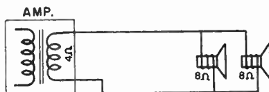
FIG. 32. Matching impedances of parallel voice coils.
