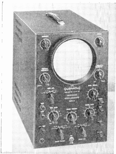
FIG. 5. Serviceman's oscilloscope designed specifically for TV Service.
