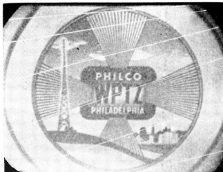
FIG. 27. When the pedestal voltage is above the cut-off point, vertical retrace lines become visible.
