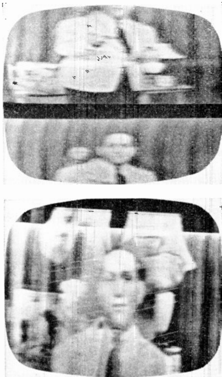
FIG. 26. Above: Vertical oscillator operating at half the correct frequency. Below: Vertical Oscillator operating at too high a frequency.
