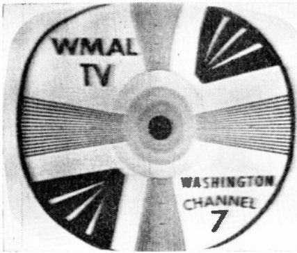
FIG. 17. Poor high frequency response. Note that only fine detail on vertical lines is lost.
