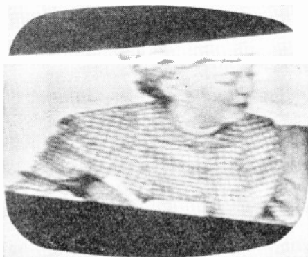
FIG. 33. Trapezoidal sweep resulting from a short across one section of vertical deflection coil.
