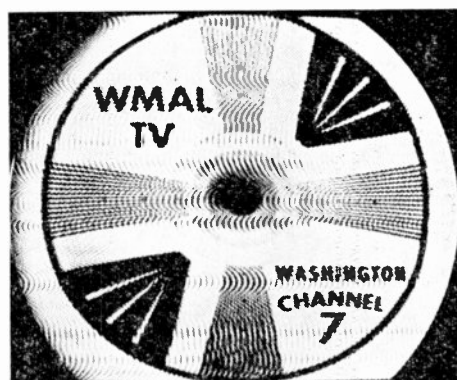
FIG. 27. Interference produced by the local oscillator of a nearby TV or FM set. The number and positions of the lines will change when the tuning of the interfering oscillator is changed. When the tuning operation stops, the pattern may change to that in Fig. 28.
