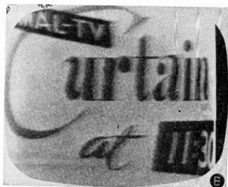
FIG. 37. Picture distortion due to open capacitor at output of linearity coil filter.
