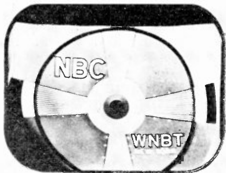
FIG. 31. The shadow at the bottom left of this picture is produced by an incorrect adjustment of the ion trap.
