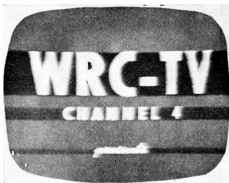
FIG. 5. Attenuation and phase shift caused by poor low-frequency response in the video amplifier.
