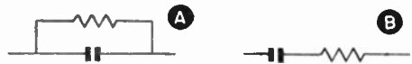
FIG. 38-1. Leakage in a capacitor has the effect of a resistor shunted across the capacitor as shown at A. Power loss has the effect of a resistor in series with the capacitor as at B.
