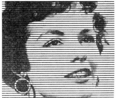
FIG. 6. Picture formed by light variations along each scanning line.
