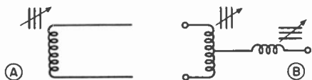
FIG. 18. Schematic drawings of (A) a ringing coil, and (B) a horizontal oscillator transformer.
