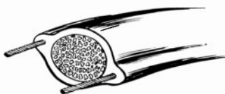
Tubular twin-lead with polystyrene center.
