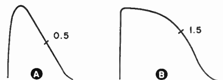
FIG. 9. Frequency response curves of Q and I demodulators. A, Q response; B, I response.
