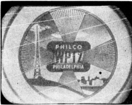
FIG. 36. Weak picture only—more characteristic of a video i-f defect.
