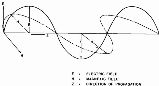
Figure 1-4. Electromagnetic Wave
