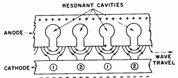
Figure 8-7. Electric Field in Linear Magnetron
