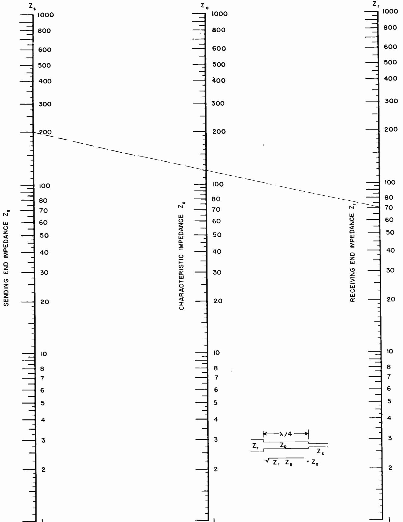
Nomogram G. Characteristic Impedance of a Quarter Wave Section Used as an Impedance Transformer
