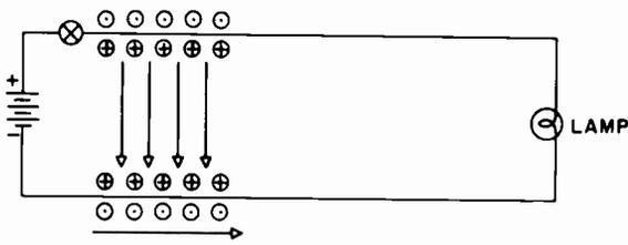
Figure 6-1. Field Created by Current Flow
