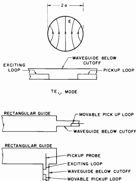
Figure 6-11. Cutoff Attenuators
