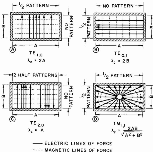
Figure 6-5. Rectangular Waveguide Modes
