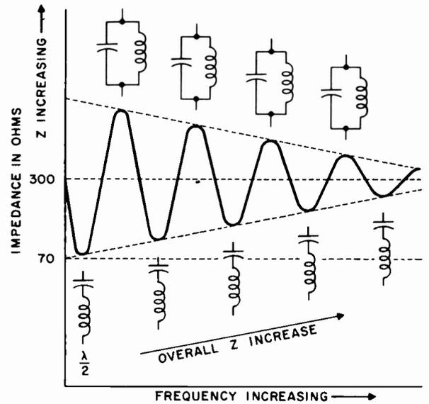
Figure 7-4. Dipole Impedance Excursions
