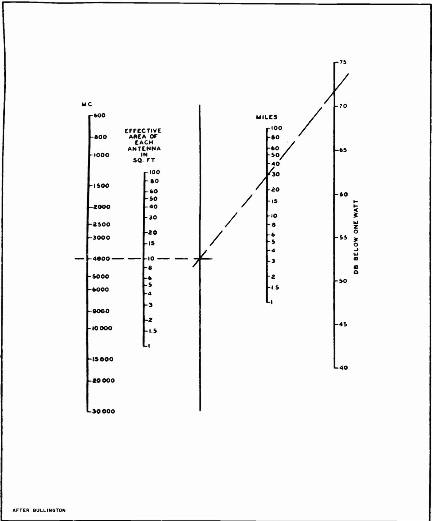
Figure 14-12. Received Power in Free Space between Two Antennas of Equal Effective Areas, 1 Watt Radiated
