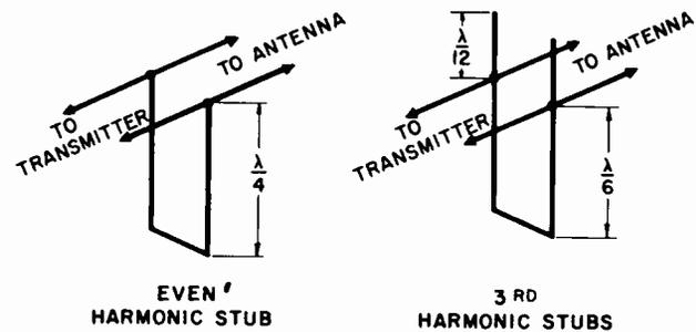
Figure 13-1. Harmonic Rejection Stubs
