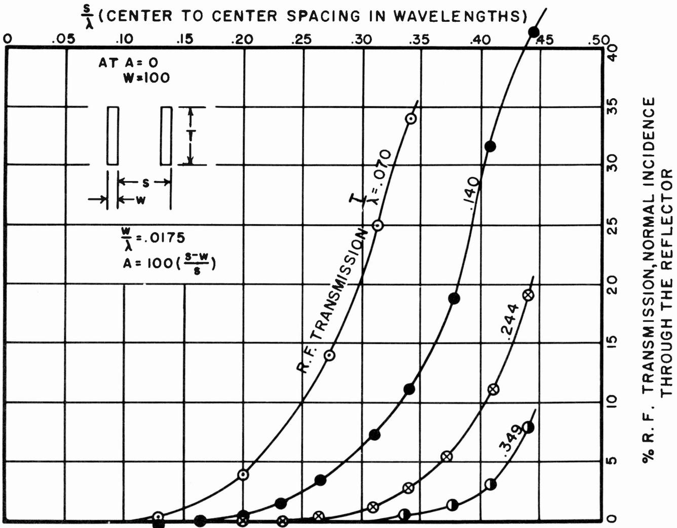
Figure 7-18. Reflector Power Loss
