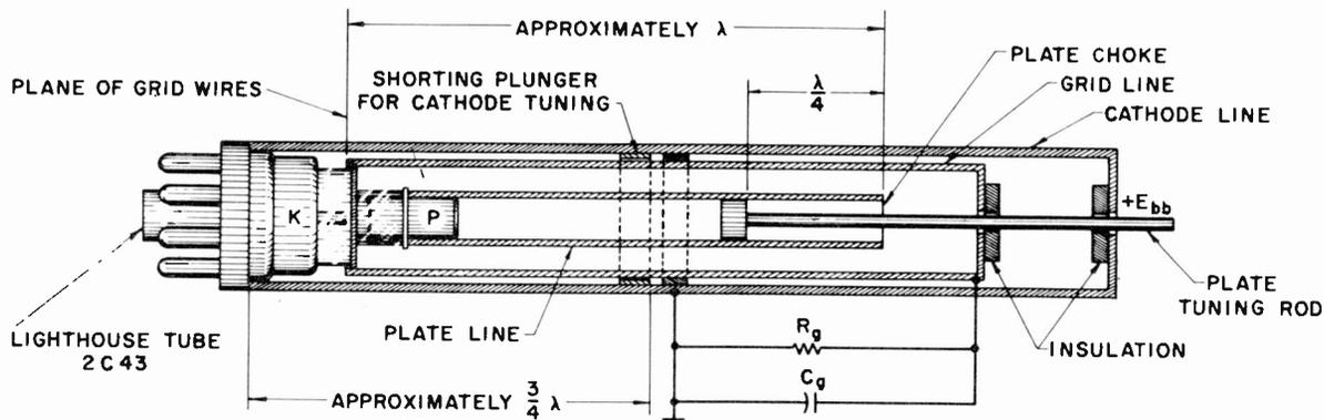
Figure 8-2. Lighthouse Tube Oscillator Circuit
