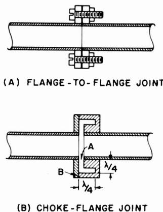
Figure 6-12. Waveguide Joints
