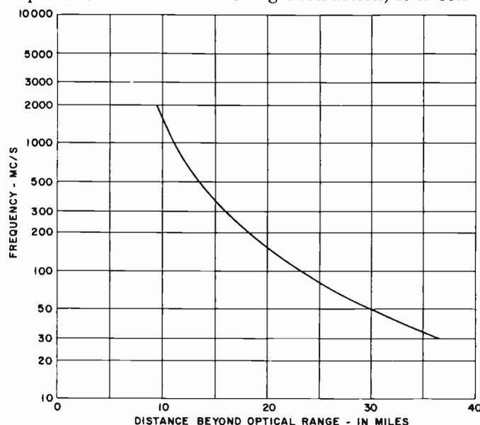
**Figure 14-4. Limitations of Bullington Nomograms Beyond the Radio Horizon**
