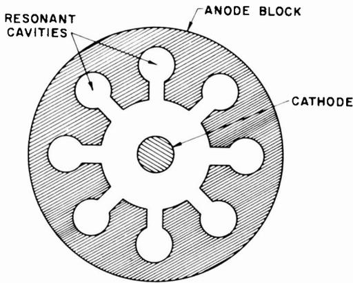
Figure 8-9. Cross-Section of Multicavity Magnetron
