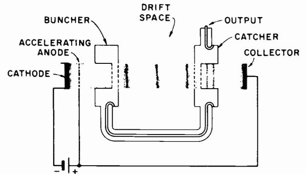
Figure 8-3. Two-Cavity Klystron Oscillator
