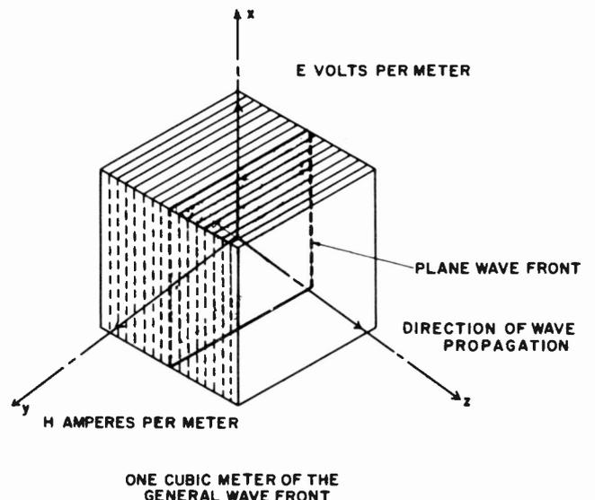
Figure 1-6. Electric & Magnetic Vectors
