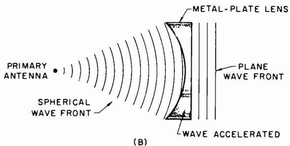
Figure 7-22. Lens Antenna Characteristics
