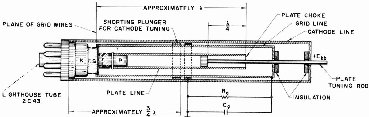
Figure 8-2. Lighthouse Tube Oscillator Circuit
