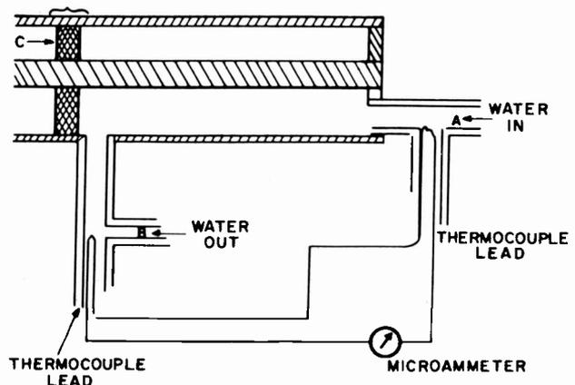
Figure 16-8. Coaxial Water Load
