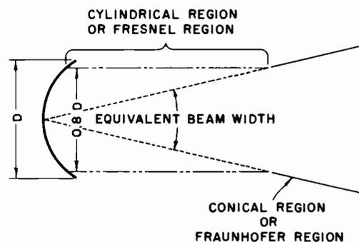
Figure 7-16. Parabolic Reflector Beaming Action
