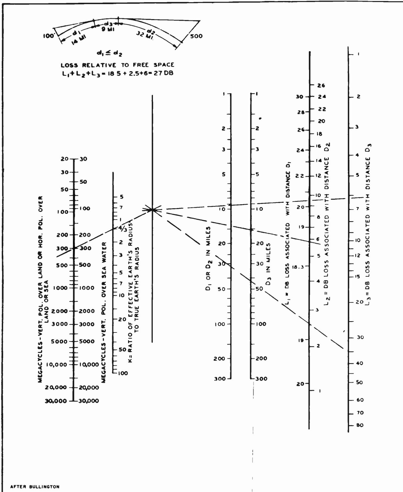
Figure 14-16. Db Loss Relative to Free Space Transmission at Points Beyond Line of Light over a Smooth Earth
