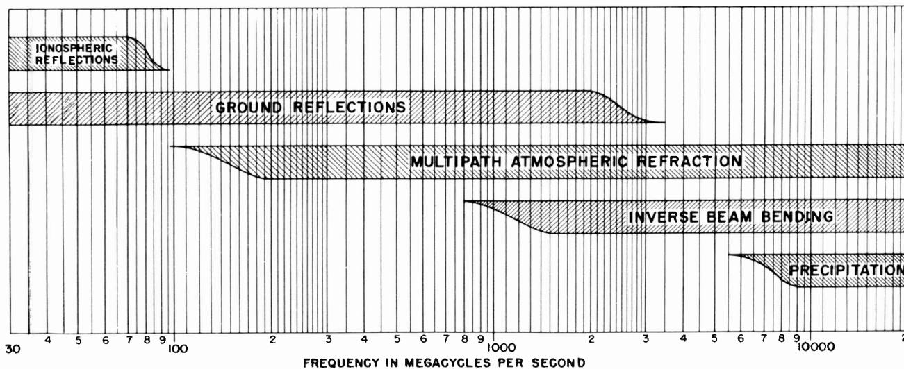
Figure 3-5. Fading Causes by Frequency
