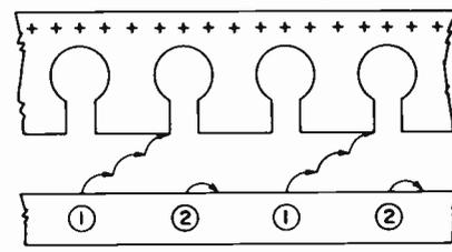
Figure 8-8. Electron Trajectories in Linear Magnetron
