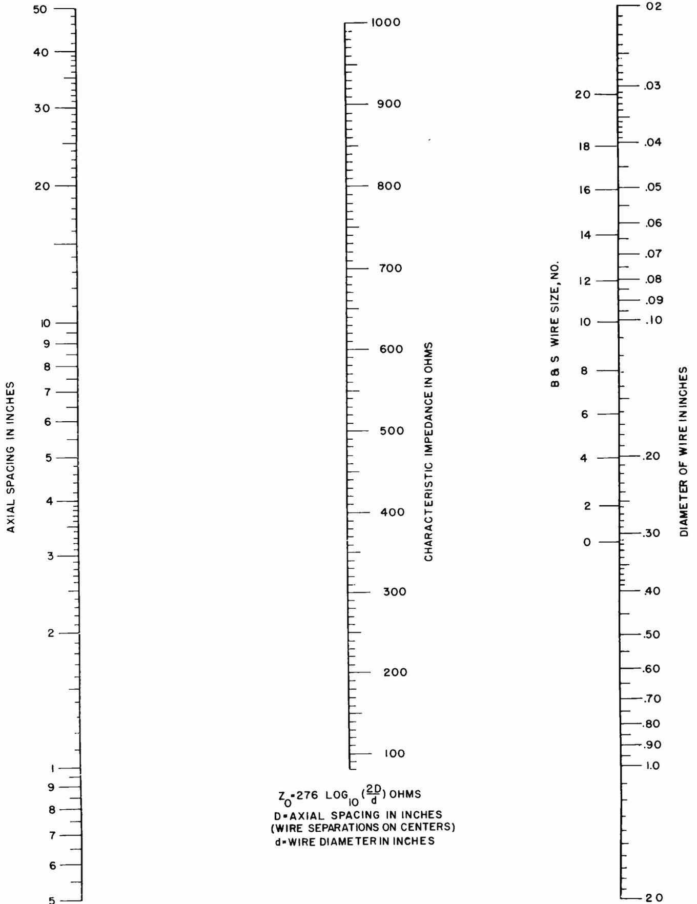
Nomogram D. Characteristic Impedance of Open Wire Lines
