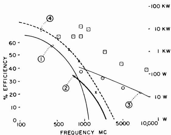
CURVE ①: EFFICIENCY VERSUS FREQUENCY FOR TYPICAL UHF TETRODE - 4X150G. (PLATE DISSIPATION 150 WATTS.)
