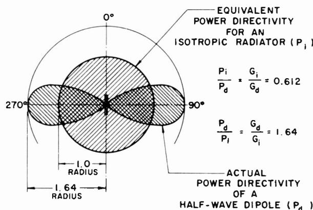
Figure 2-2. Relative Antenna Gain
