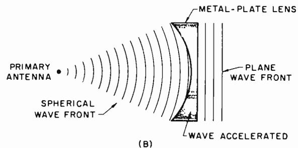
Figure 7-22. Lens Antenna Characteristics
