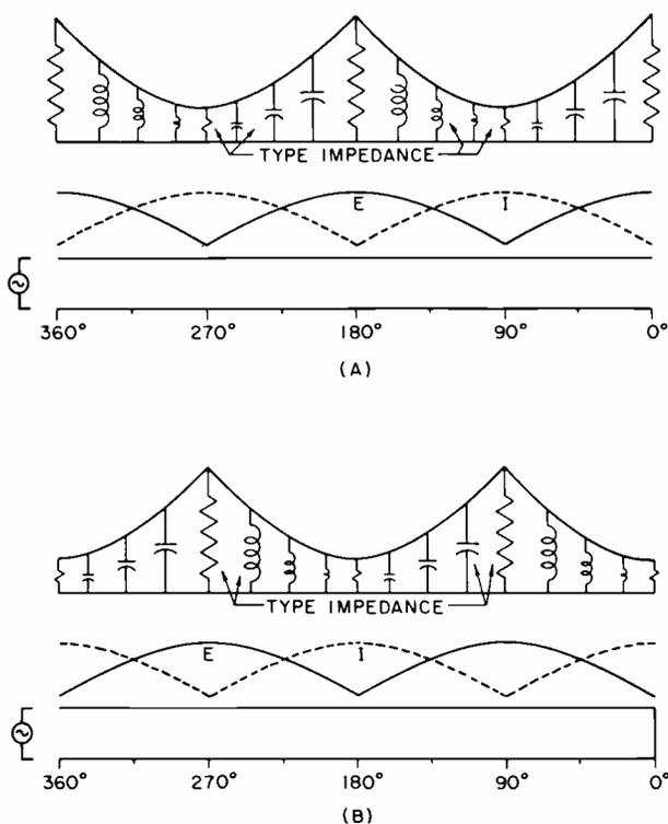
Figure 6-3. Open and Shorted Transmission Lines
