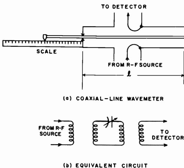
Figure 16-1. Coaxial Line Wavemeter
