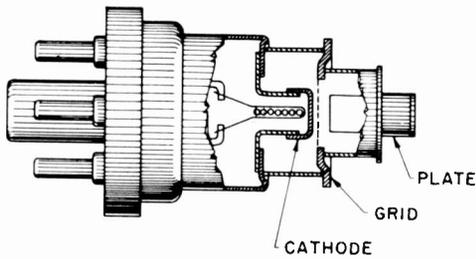
Figure 8-1. Lighthouse Tube (Cross-Section)
