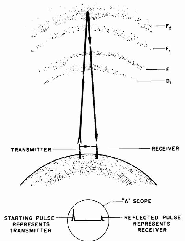
Figure 15-2. RF Sounding of Ionosphere
