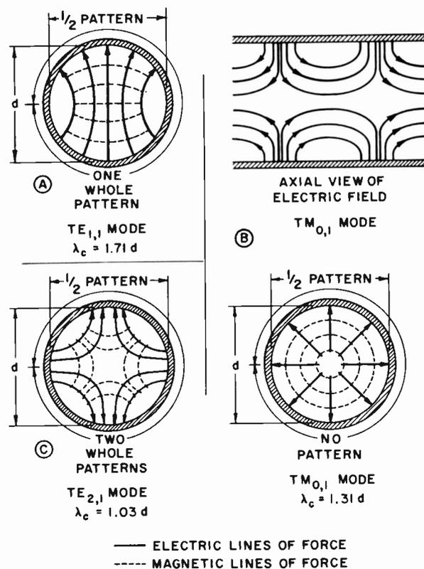
Figure 6-6. Circular Waveguide Modes
