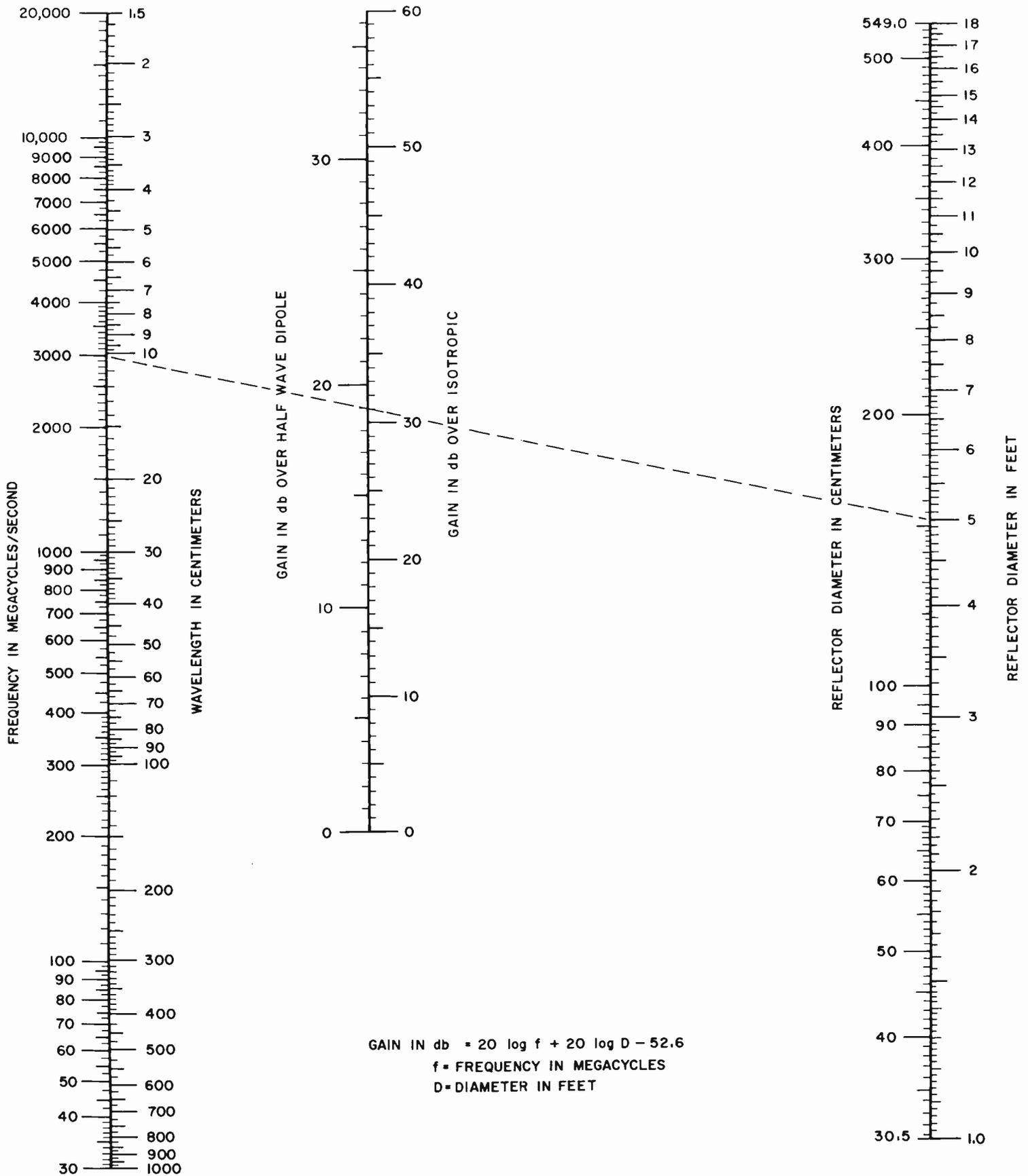
Nomogram K. Gain of Parabolic Antennas
