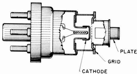
Figure 8-1. Lighthouse Tube (Cross-Section)
