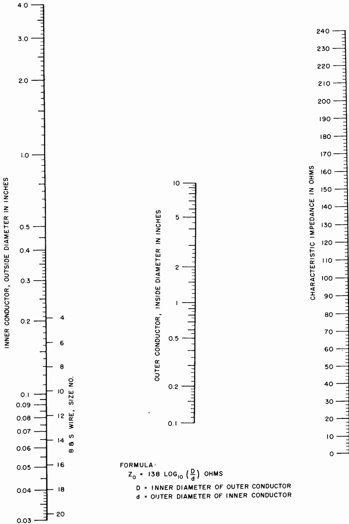
Nomogram E. Characteristic Impedance of Air-Filled Coaxial Lines
