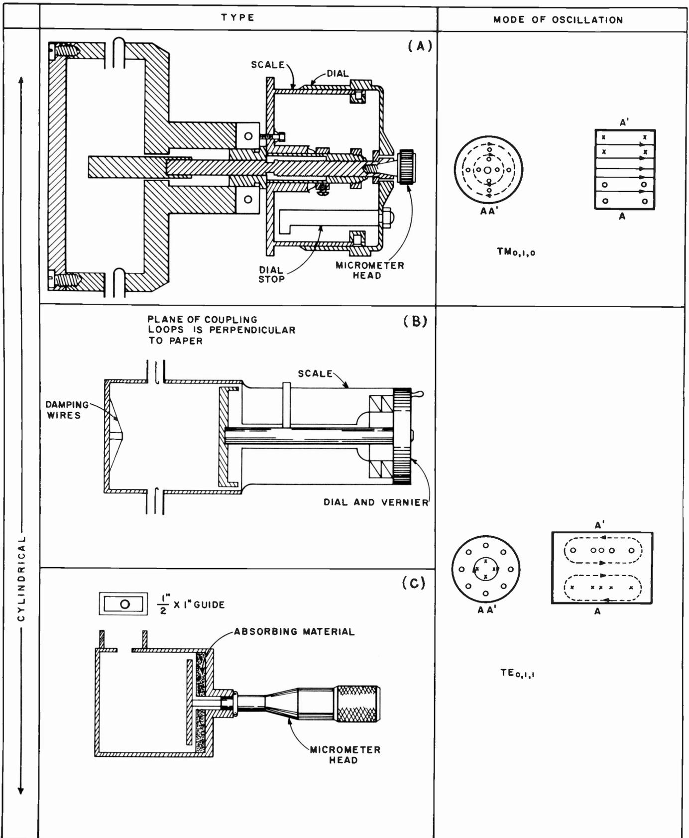
Figure 16-3. Cylindrical Wavemeters
