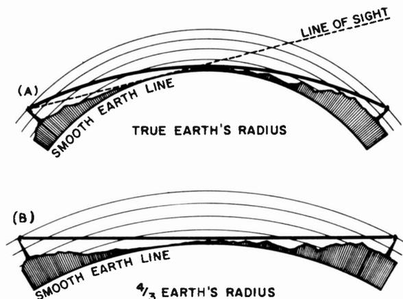
Figure 1-15. Refraction through Standard Atmosphere
