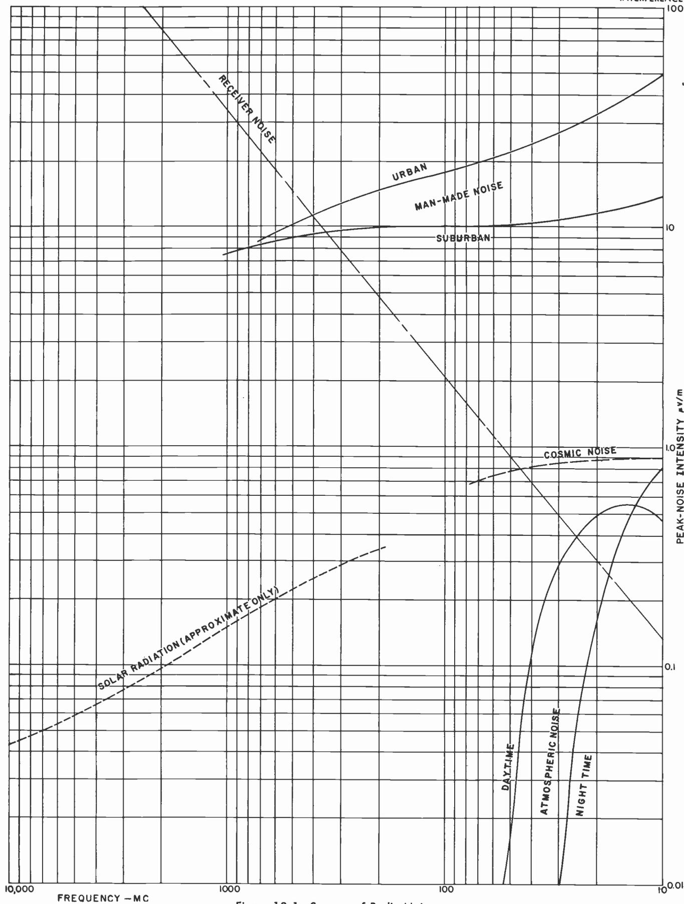
Figure 12-1. Sources of Radio Noise
