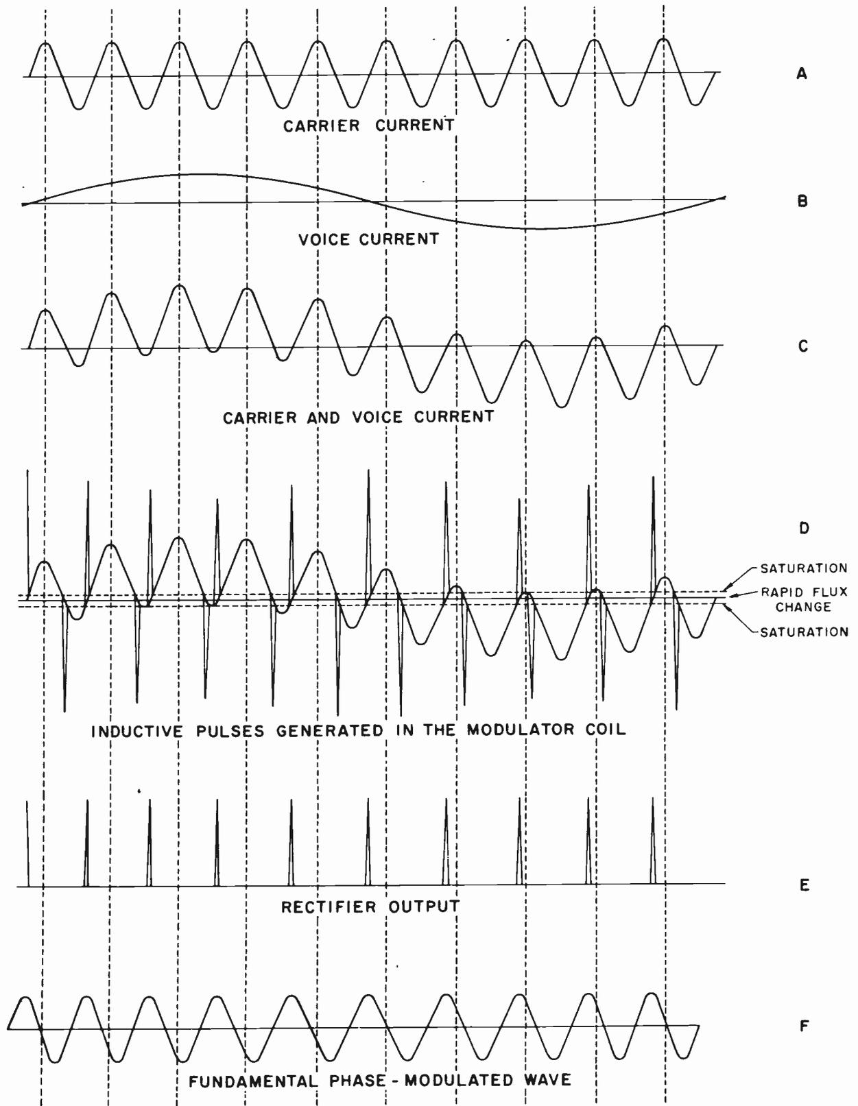
Figure 8-12. Waveforms Developed in Nonlinear Coil Modulator
