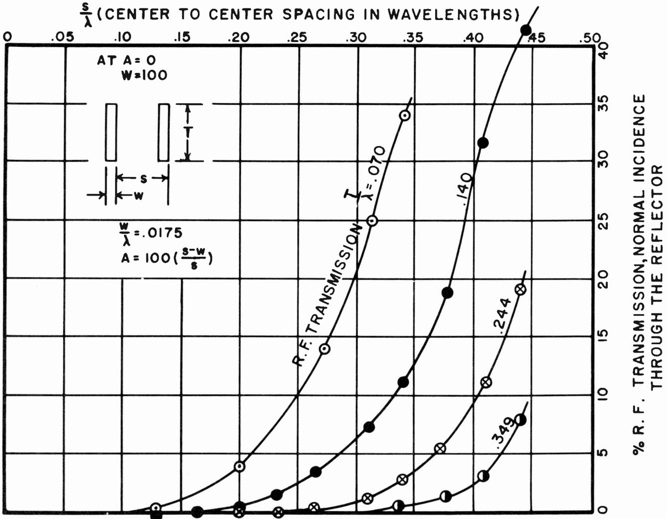
Figure 7-18. Reflector Power Loss
