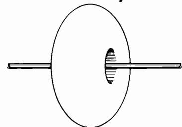
Figure 7-7. Dipole Field Pattern
