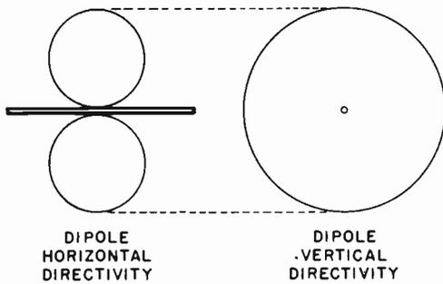
Figure 7-8. Horizontal and Vertical Directivity Pattern
