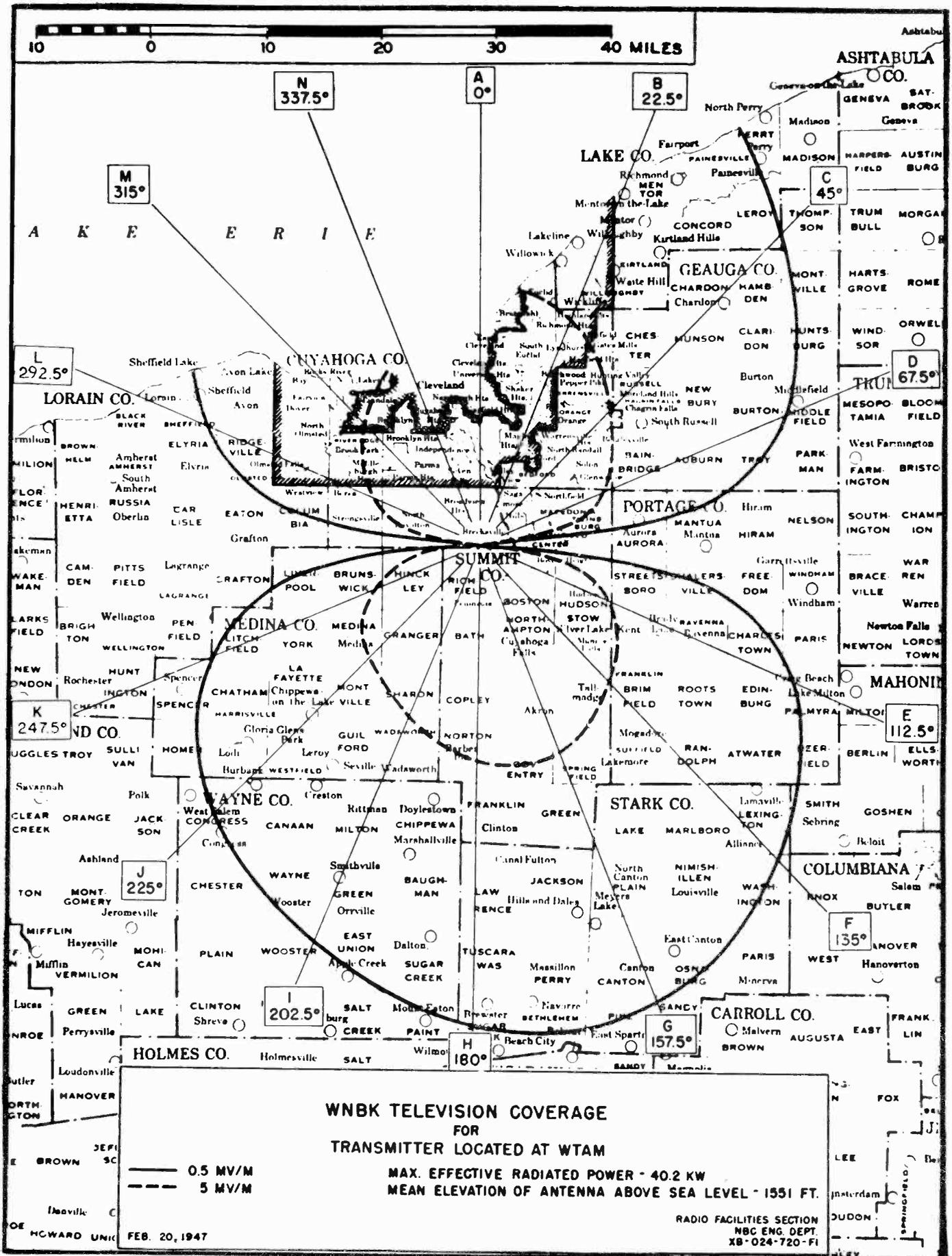
Figure 2-3. Polar Diagram of Field Strength
