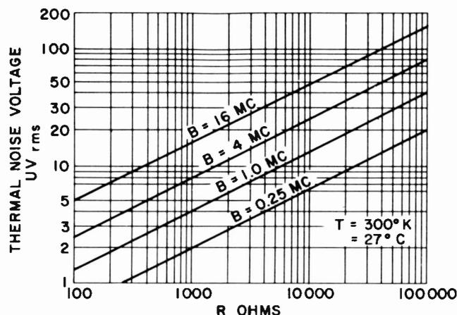
Figure 12-2. Thermal Agitation Noise
