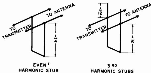
Figure 13-1. Harmonic Rejection Stubs
