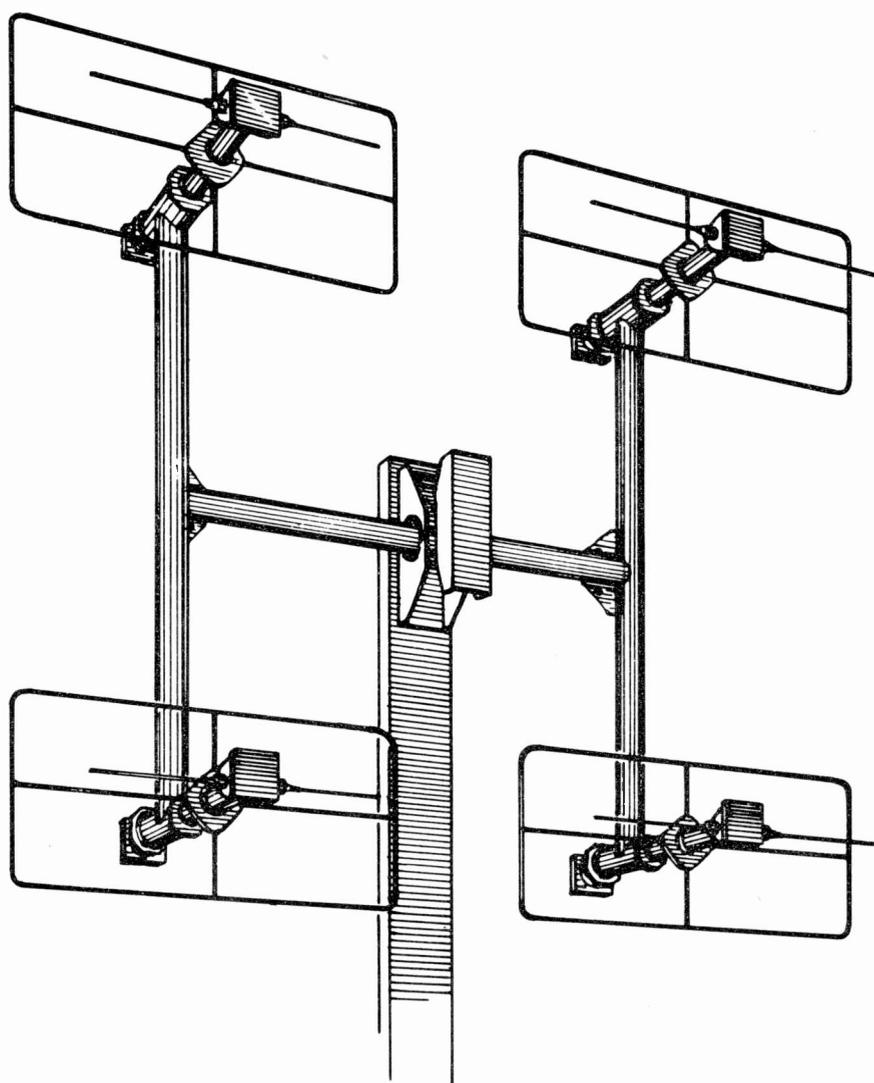
Figure 7-13. Four Element Broadside Array
