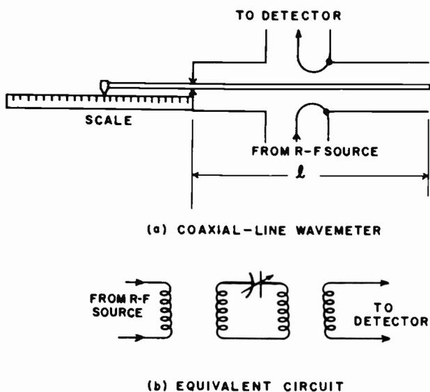
Figure 16-1. Coaxial Line Wavemeter
