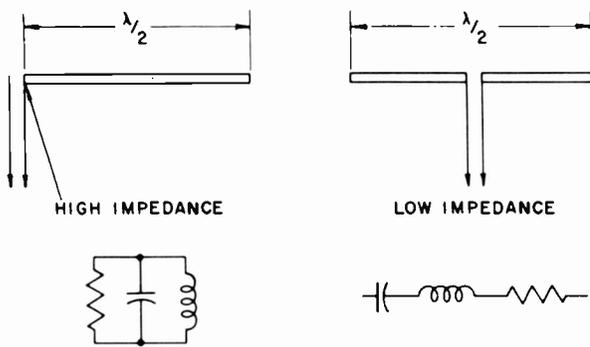
Figure 7-1. Antenna Feed Systems
