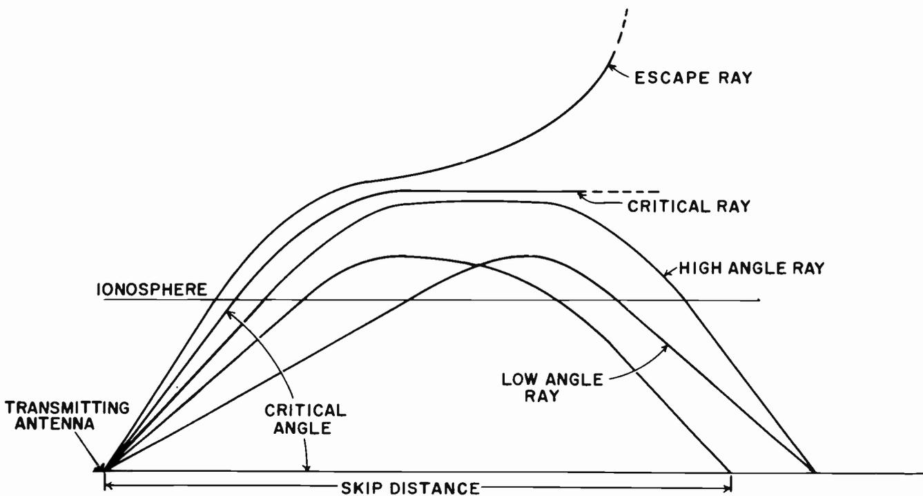
Figure 15-3. Ionospheric Dispersion
