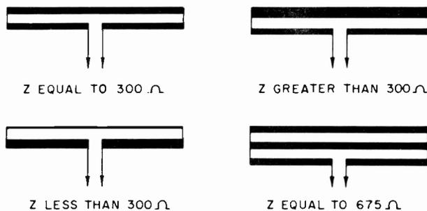
Figure 7-11. Folded Dipole Impedances
