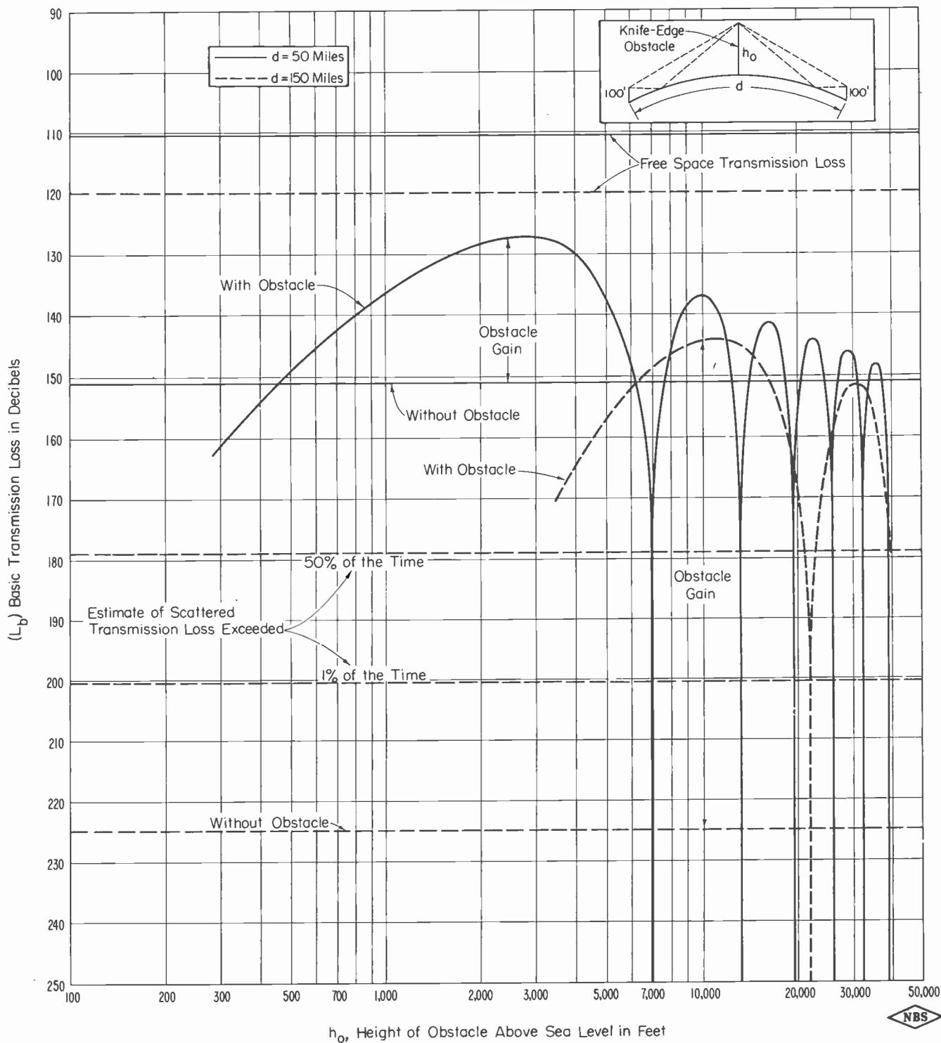
Figure 2-5. Attenuation with Obstacle
