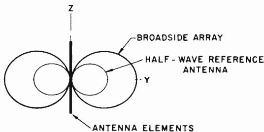
Figure 7-12. Vertical Directivity of Broadside Array
