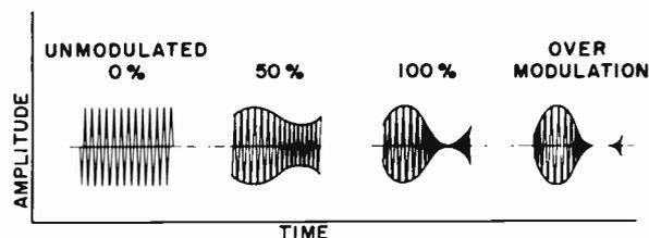
Figure 8-11. Amplitude Modulation Waveforms
