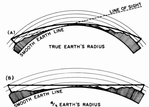
Figure 1-15. Refraction through Standard Atmosphere
