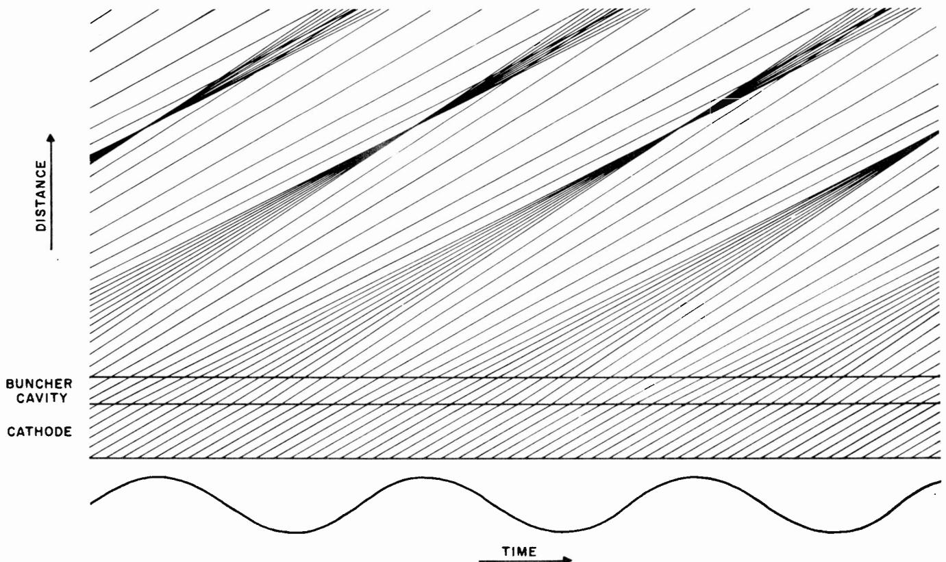
Figure 8-4. Bunching in Two-Cavity Klystron
