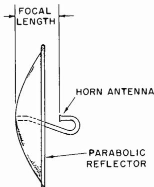
Figure 7-21. Horn Fed Parabola
