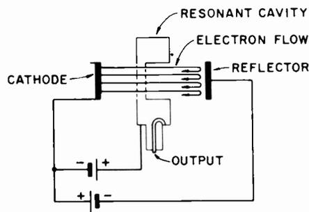
Figure 8-5. Reflex Klystron Oscillator
