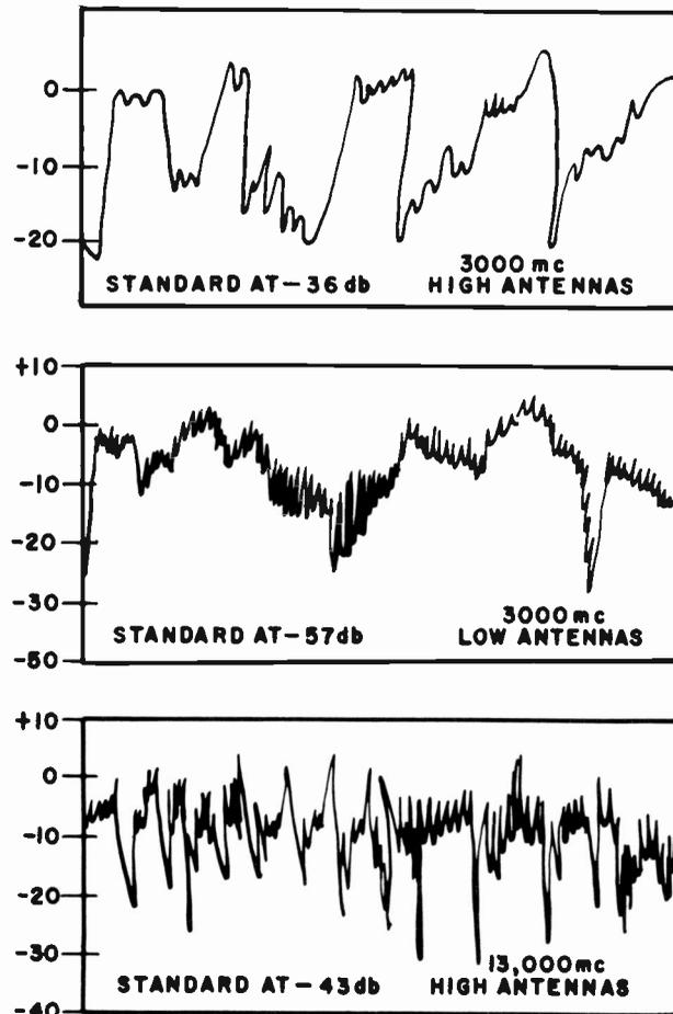
Figure 3-4. Fading Comparison
