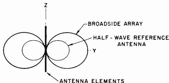
Figure 7-12. Vertical Directivity of Broadside Array
