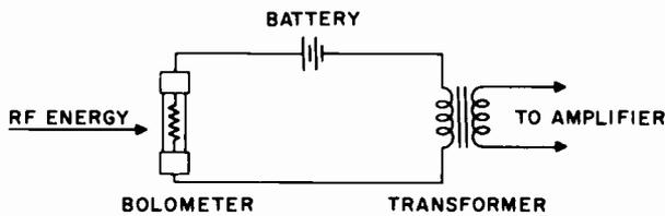
Figure 16-7. Bolometer Bias Circuit
