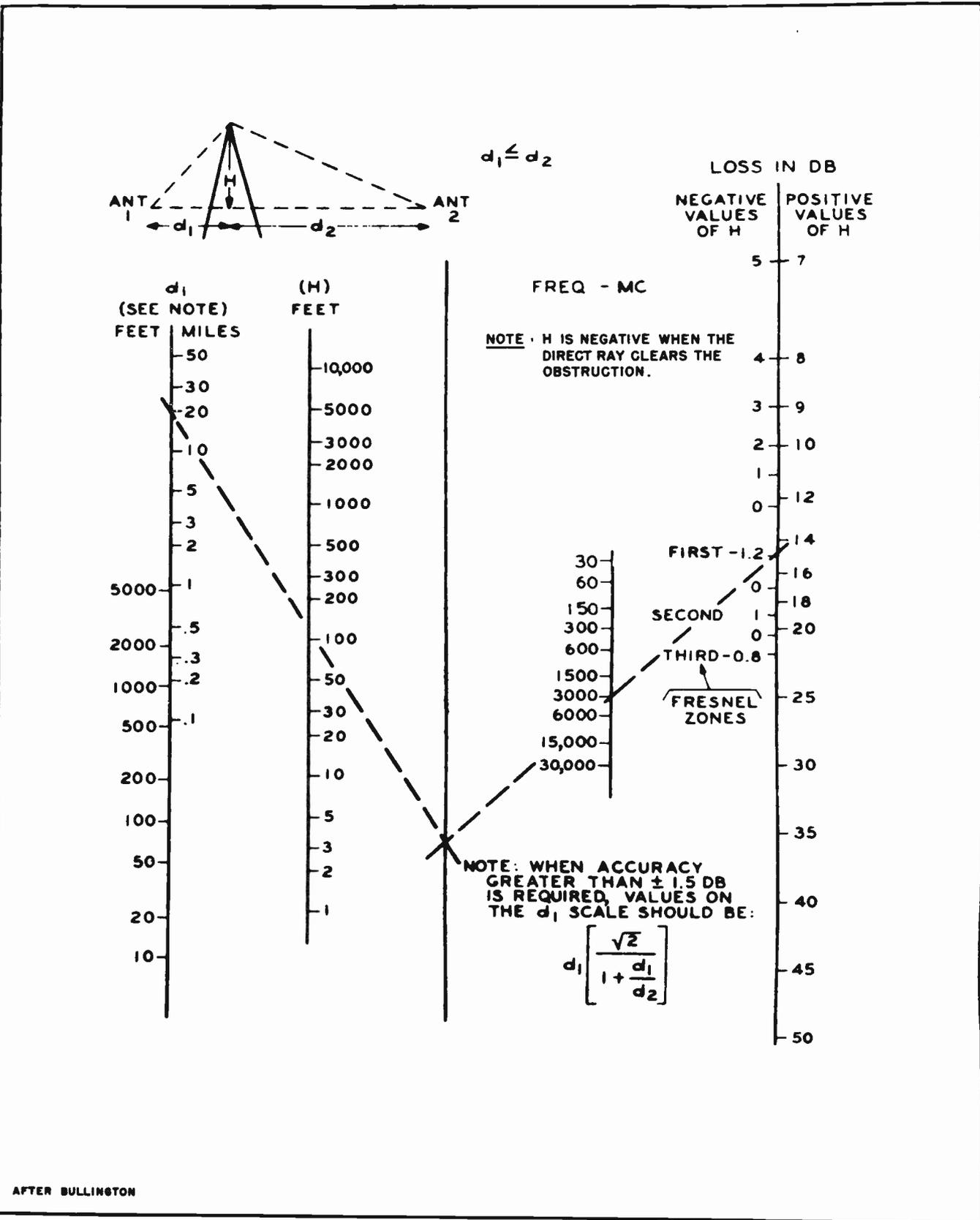
Figure 14-18. Shadow Loss Relative to Free Space
