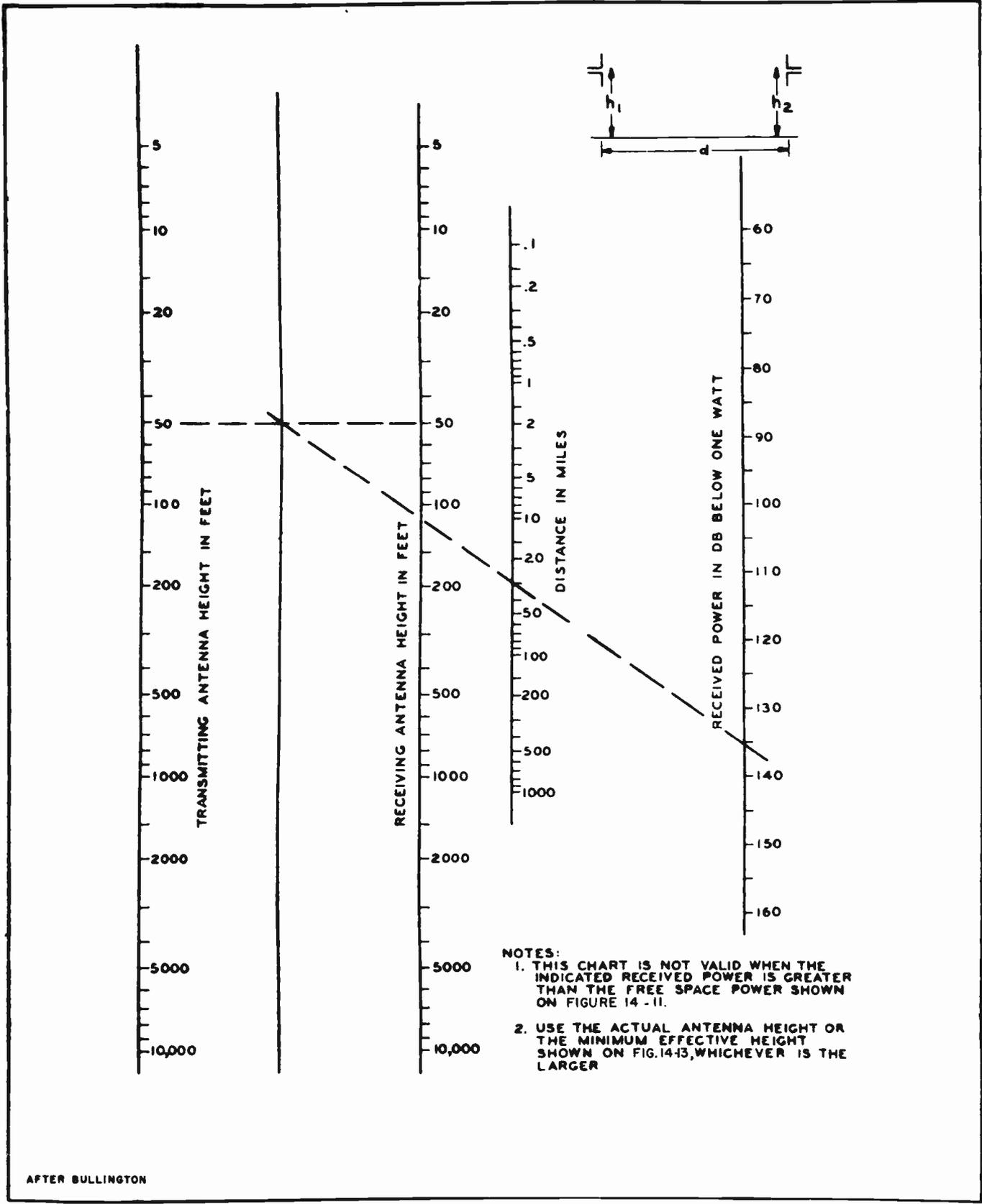
Figure 14-14. Received Power over Plane Earth Between Half-Wave Dipoles, 1 Watt Radiated
