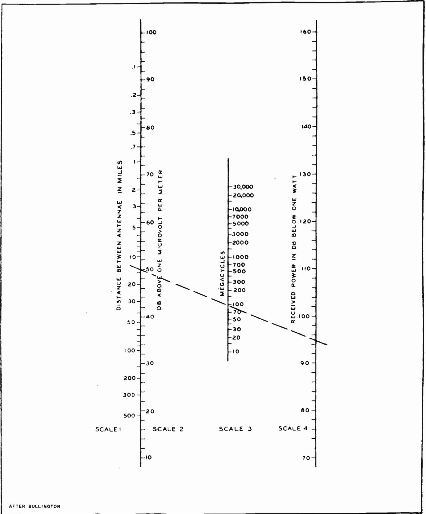
Figure 14-11. Free Space Field Intensity and Received Power between Half Wave Dipoles, 1 Watt Radiated
