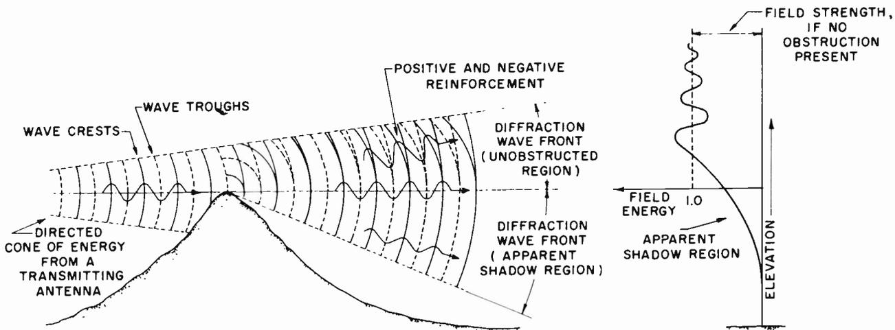
Figure 1-9. Diffraction
