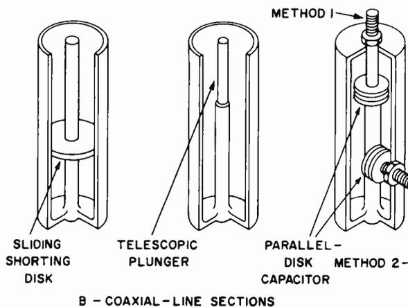
Figure 6-7. Common Tuning Methods
