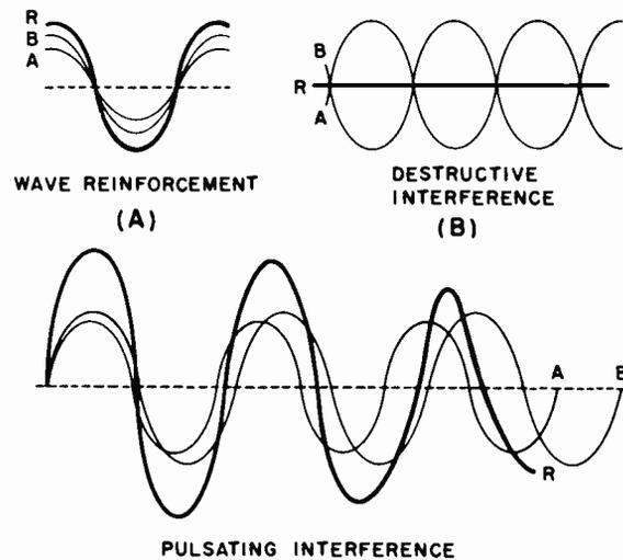
Figure 1-2. Interference of Waves
