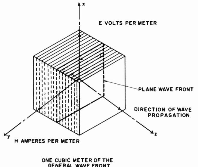
Figure 1-6. Electric & Magnetic Vectors
