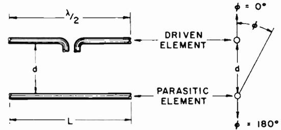
Figure 7-10. Antenna Array with One Parasitic Element
