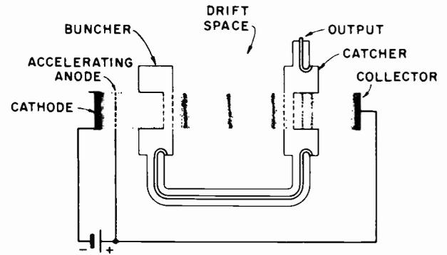
Figure 8-3. Two-Cavity Klystron Oscillator
