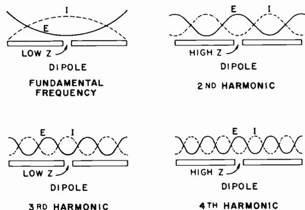
Figure 7-2. Dipole Current and Voltage Distribution
