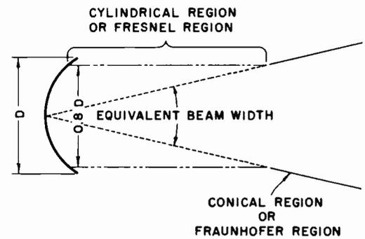
Figure 7-16. Parabolic Reflector Beaming Action
