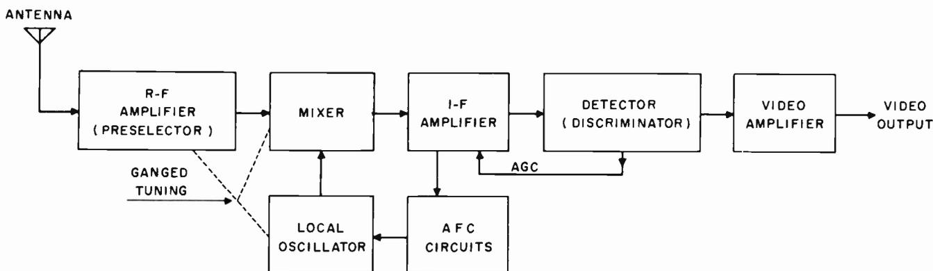
Figure 9-1. Block Diagram of Superheterodyne Receiver
