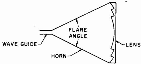
Figure 7-23. Lens-in-Horn Antenna
