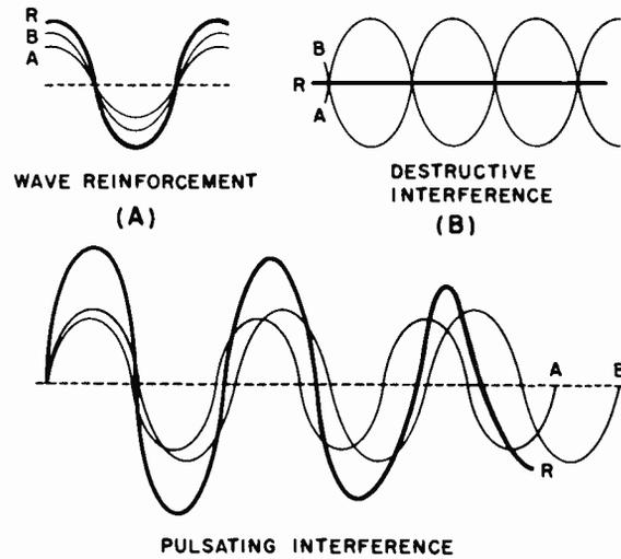
Figure 1-2. Interference of Waves
