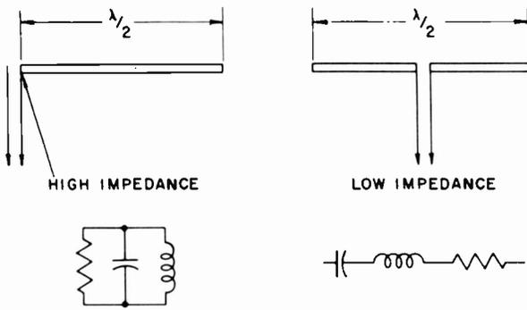
Figure 7-1. Antenna Feed Systems
