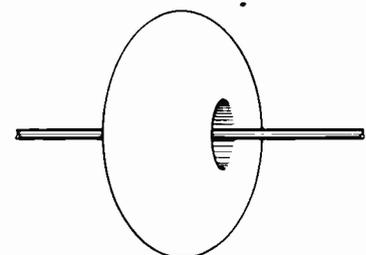
Figure 7-7. Dipole Field Pattern
