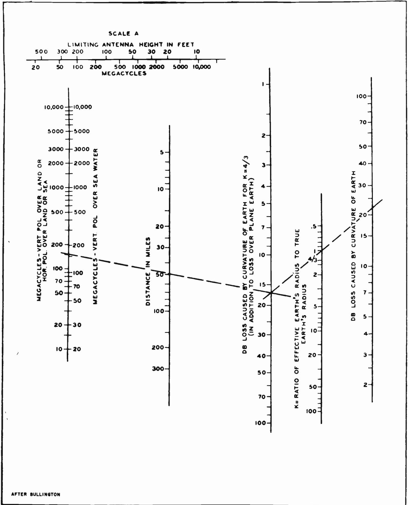
Figure 14-15. Diffraction Loss Caused by Curvature of the Earth Assuming Neither Antenna Height is Higher than Shown on Scale A
