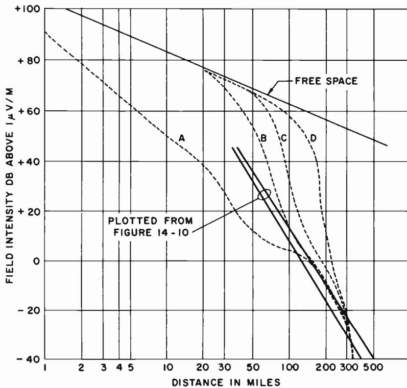
CURVES A, B, C AND D, SHOW MEDIAN VALUES OF FIELD STRENGTH FOR VARIOUS RECEIVING ANTENNA HEIGHTS. FREQUENCY 410 MC/S. EFFECTIVE RADIATED POWER 1 KW. TRANSMITTING ANTENNA HEIGHT 40 FEET.
