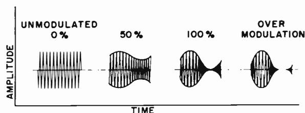
Figure 8-11. Amplitude Modulation Waveforms
