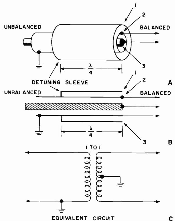
Figure 6-9. Bazooka Line Balance Converter
