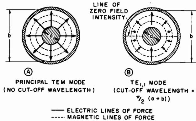
Figure 6-4. Coaxial Modes of Operation
