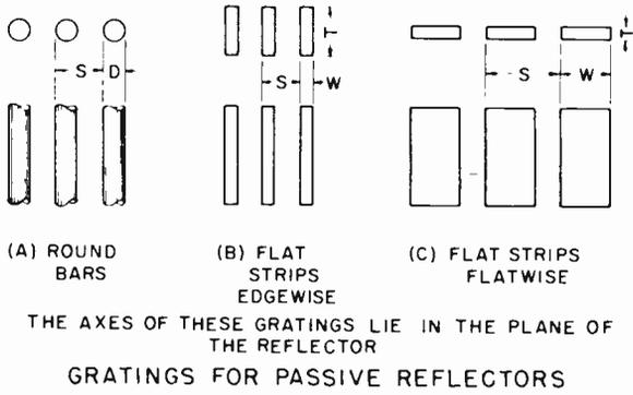
Figure 7-17. Gratings for Passive Reflectors
