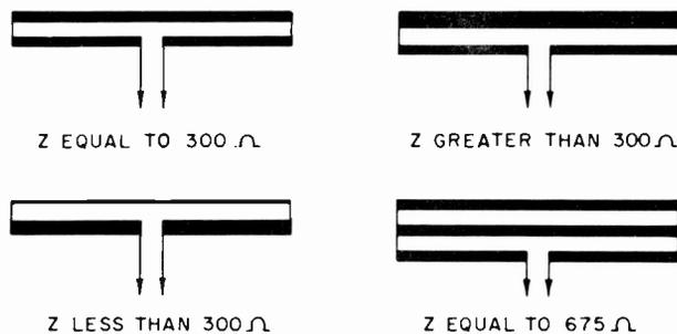
Figure 7-11. Folded Dipole Impedances
