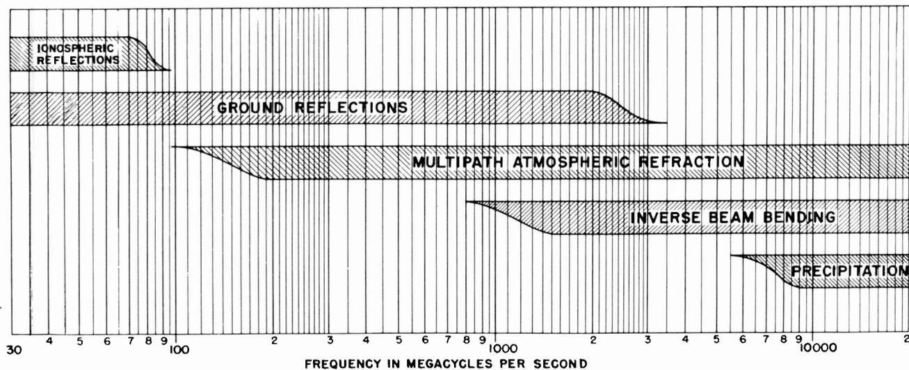
Figure 3-5. Fading Causes by Frequency
