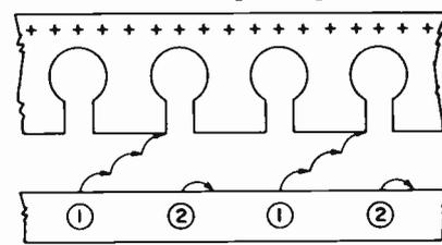
Figure 8-8. Electron Trajectories in Linear Magnetron
