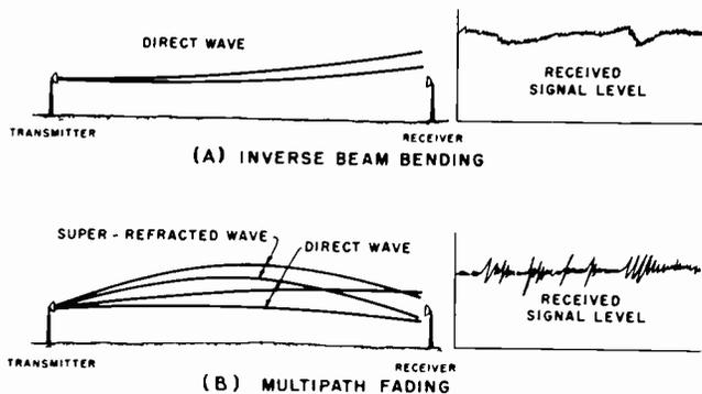
Figure 3-1. Single & Multipath Fading
