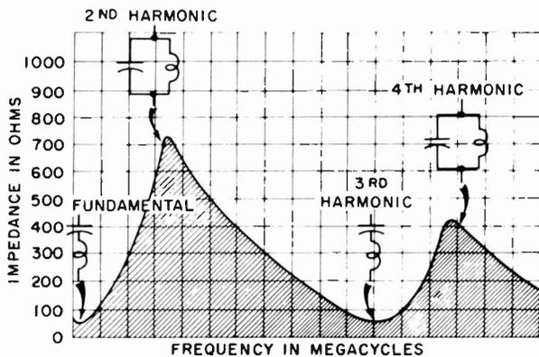
Figure 7-5. Dipole Impedance Variation
