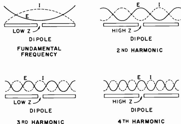
Figure 7-2. Dipole Current and Voltage Distribution
