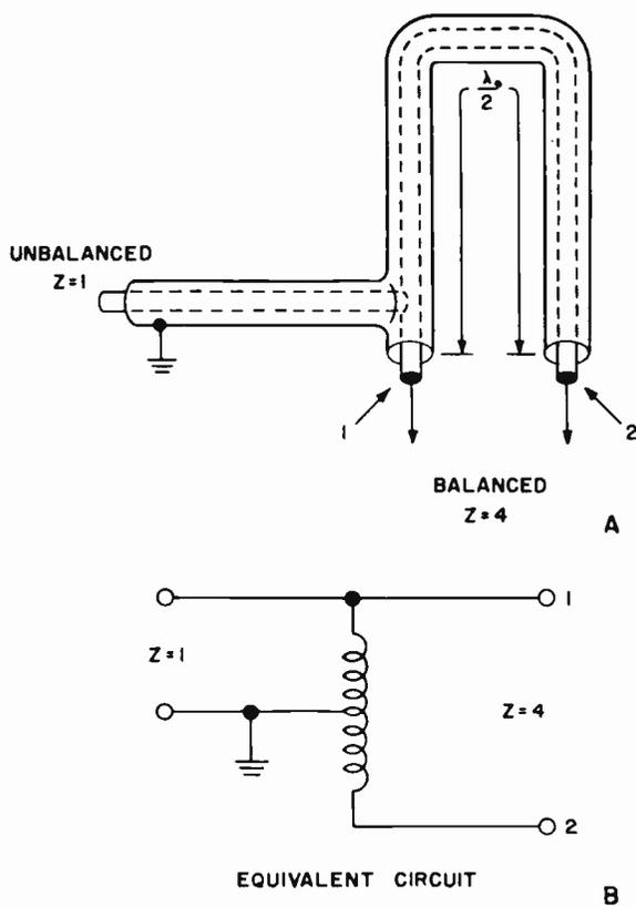
Figure 6-10. Phase Inverter as Line Balance Converter
