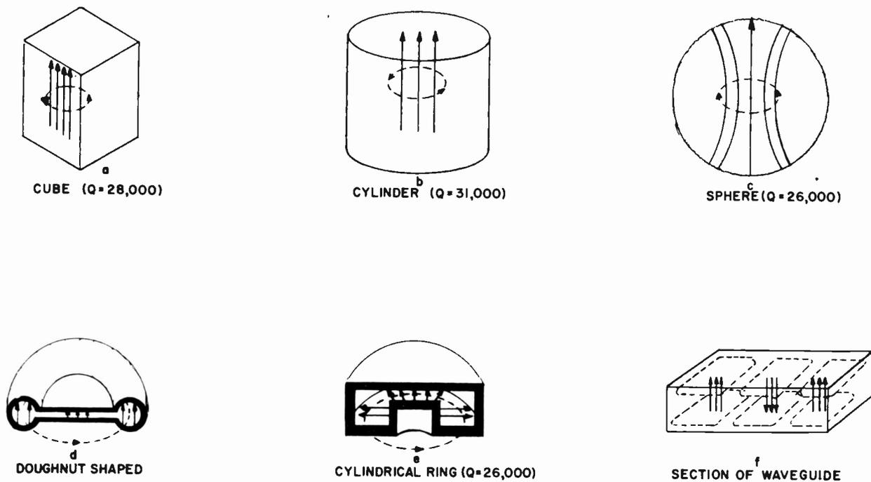
Figure 6-8. Types of Cavities
