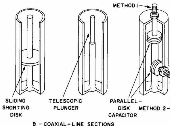
Figure 6-7. Common Tuning Methods
