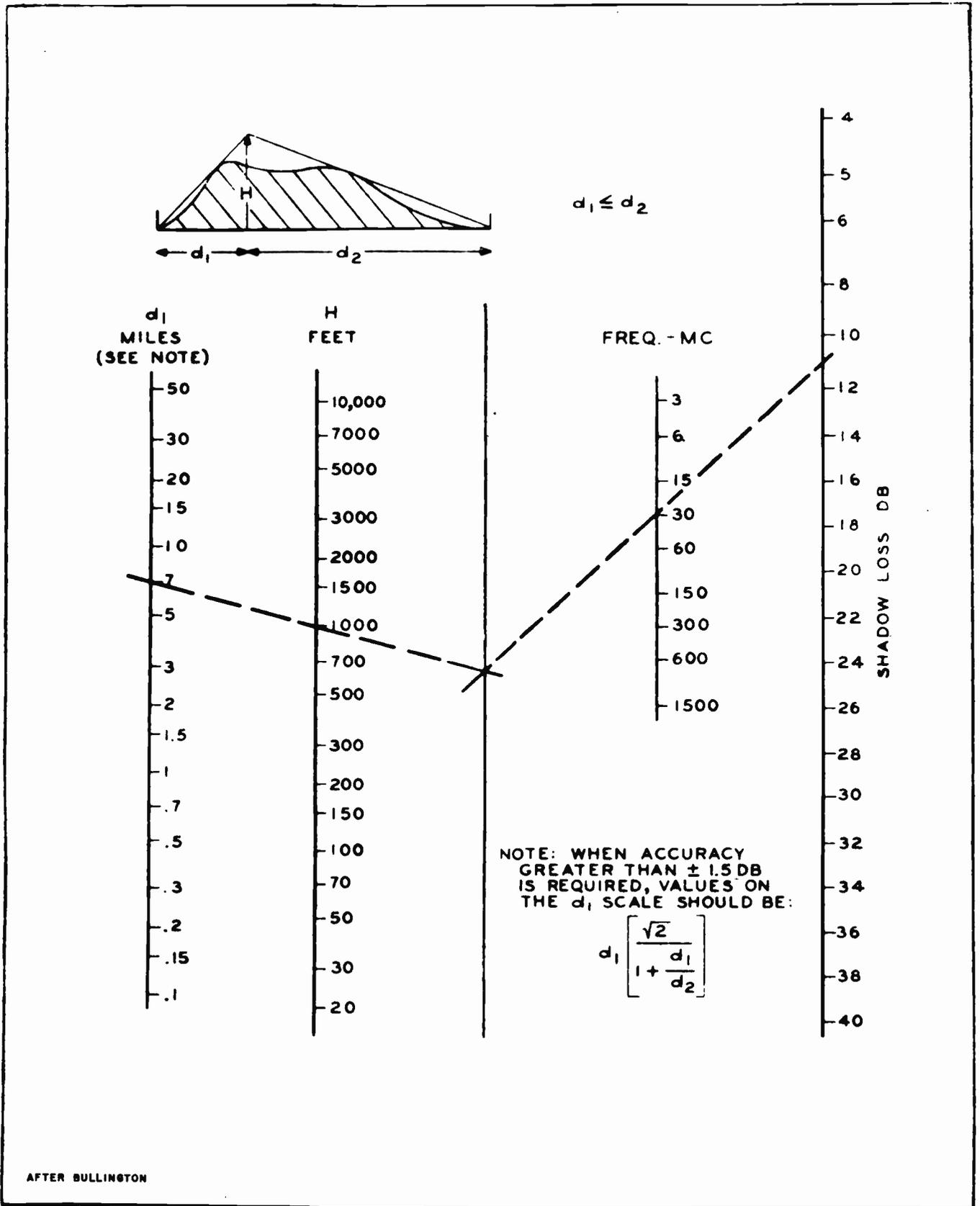
Figure 14-19. Shadow Loss Relative to Smooth Earth
