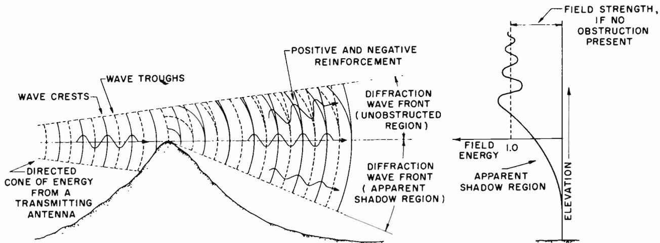
Figure 1-9. Diffraction
