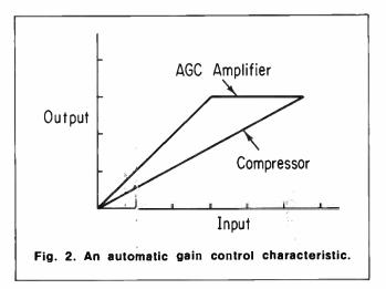
†AGC should not be confused with AVC (automatic volume control), which is a technique for maintaining carrier levels in a receiver.
