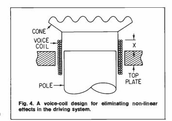
will be a constant if the amplitude of excursion is always less than x of fig. 4. The reduction in distortion by employing the expedient of fig. 4 is shown by the curve **B** of fig. 3.
