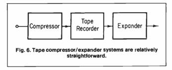
The compressed signal is recorded on the tape which contributes additional noise. During playback, the apparent noise is minimized by the expander action which reduces gain in the presence of low-level signals. In one current application of this principal, the Dolby system, the audio spectrum is divided into several regions, each with its own pair of control elements.
