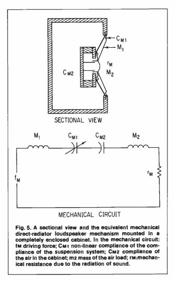
is the controlling compliance as shown in fig. 5. The mechanical circuit of fig. 5 depicts the method for reducing the deleterious effects of a non-linear suspension. The non-linear distortion is reduced to curve C by the use of the low-frequency-resonant loudspeaker mechanisms housed in a completely enclosed cabinet of fig. 5 and the voice-coildesign of fig. 4.
