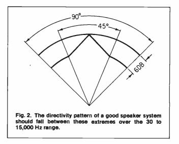
shown for an angle of at least 45%. For really high quality, the polar curves should fall within the amplitude limits shown for an angle of 90%.
