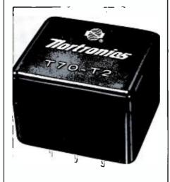
The T70-T2 bias oscillator features convenient plug-in dip-solder terminals and has the same efficient ferrite E-core construction and electrical characteristics as the popular Nortronics T60-T2 transformer. This unit will furnish up to 110 kHz of bias and erase power to full-track heads or to both channels of a stereo recorder.
