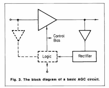
output signal is rectified and fed back as control bias to this variable gain stage. Since the circuit arrangement constitutes a negative feedback loop, it tends to be selfregulating. A high level audio signal produces enough control bias to lower the gain to the point where the output level no longer produces excessive control bias. When low-level signals are encountered, the reverse action takes place and the gain is increased. In this way the output tends to be maintained at a constant level.
