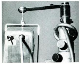
Figure 5. The leaf-spring suspension employed on the C-4 microphone. Ribbon mics are insensitive to shock in a plane parallel to the ribbon, a fact teken into account in this simple design.
