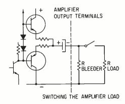
Figure 1. Switching the amplifier load.
