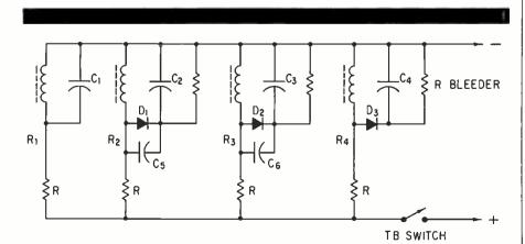
Figure 4. A relay-operating capacitive-delay circuit. In the circuit, R is the same in all cases, C1 is the smallest and C4 is the largest. The turn-on sequence is R1, R2, R3, R4. D1, D2, and D3 prevent discharge through the coils of R2, R3, and R4, but C5 and C6 delay turn-off enough to reverse the sequence with the same time constants:  $C_1 < C_2 < C_3 < C_4$   $C_5 < C_6$ .
