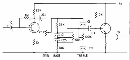
Figure 3. The final circuit that overcame the difficulties.
