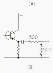
Figure 6. Different ways of achieving output internal impedance: (A) using voltage and/or current feedback, applied over the active device (shown here as a transistor); (B) using an actual internal series resistor from a stage (shown here as emitter follower) that is essentially constant voltage, or zero impedance.
