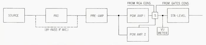
Figure 1. A block diagram of the Langevin console. The VU meter bridges (through a Langevin bridging card) the program line after the output selector switch (s) thereby tracking any source feeding the transmitter.
