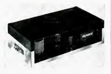
• Low cost reliability is claimed for this solid-state stereo amplifier rated at 40 watts continuous per channel. T.h.d. is rated at under 0.5 per cent at rated output, and i.m. is under 0.1 at rated output. Built-in current limiting circuitry eliminates the need for protective fusing, and permits placement of the amplifier in relatively inaccessible locations. Kit and factoryassembled versions are available. *Mfr.: Dynaco Div.*
