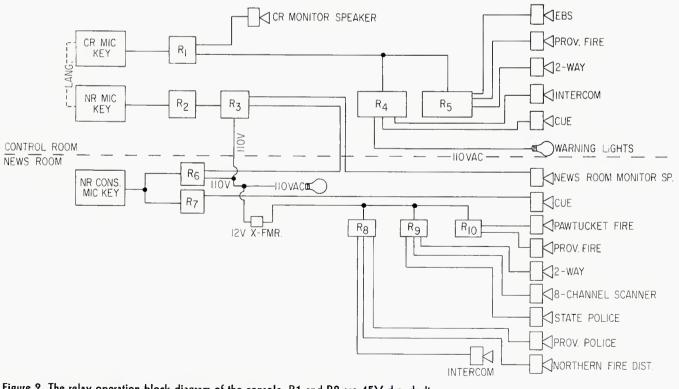
Figure 2. The relay operation block diagram of the console. R1 and R2 are 45V d.c. dpdt; R3, R4, R5 are 12V a.c. 3pdt; R6 and R7 are 24V d.c. supplied with the RCA console, R8, R9, R10 are 12V a.c. 3pdt. Load reisstors are substituted for all speakers when microphone keys are opened. R1 and R2 are used to switch 12V a.c. located physically outside the console. Note that the CR and NR mic keys are ganged on the Langevin console.
