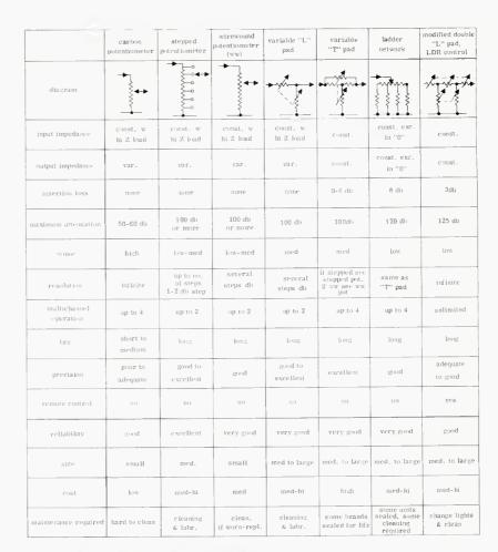
Figure 1. A comparison of various attenuator types.
