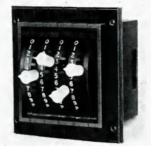
• A total of 250,000 operations are promised from this random-access unit which will switch from any one position to any of ten others without making contact with intermediate switch points. It has modular, expandable construction which allows any practical number of units to be stacked side-by-side. Contacts will carry 3 amps static, 250 mA during switching and have a resistance of 75 milliohms maximum. The switch is designed for p.c. board mounting.
