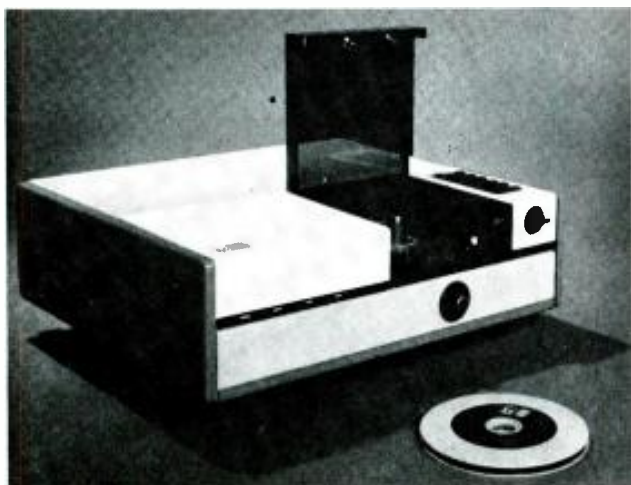
Figure 2. The EVR player and cartridge. The player is being manufactured by Motorola in an exclusive arrangement with CBS.
