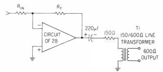
Figure 9. Alternate 600-ohm output connection for +23 dBm. You should change R11 to provide sufficient current output, and heat sinking of both the IC and Q1 is recommended. The amplifier should be labeled - - circuit of Figure 4.
