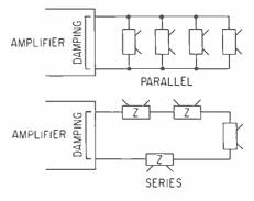
Figure 1. A comparison between parallel and series connection of speakers at an amplifier output to show the reason, based on damping, usually expressed for preferring parallel connection.
