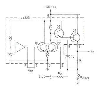
Figure 3. A #A723 connected as an audio amplifier.
