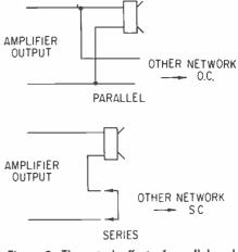
Figure 3. The actual effect of parallel and series networks does not make much difference to the coupling of damping factor to each speaker unit within its own frequency range.
