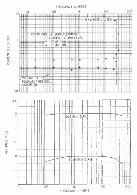
Figure 5. Total harmonic distortion at 10 dB and 20 dB gains
