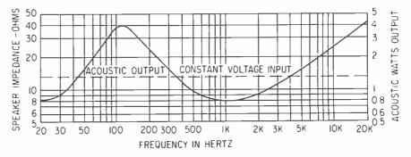
Figure 2. The effect of damping factor on frequency response. The solid curve represents a typical impedance curve. The dashed line is an ideal constant-voltage frequency response (it may not be this good). The solid curve also represents the frequency response when fed constant-current, or from an amplifier with a low damping factor.
