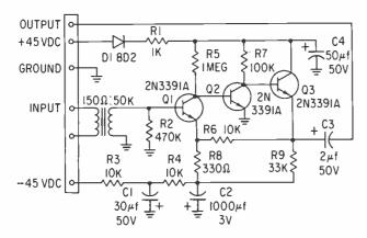
Figure 1. A mic preamp constructed with discrete components.
