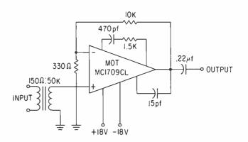
Figure 3. An integrated circuit mic preamp.
