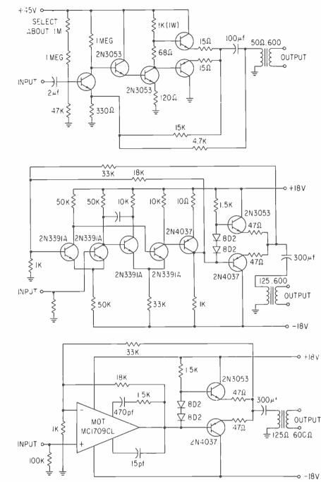
Figure 4. A line amp using discrete components.
