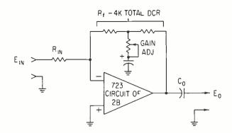
Figure 10. A configuration for adjustable gain.
