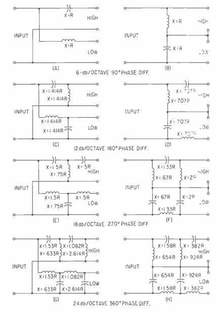
Figure 4. These are possible circuits, using from one to four reactance elements in each section to give constant resistance performance. Reactances are given in terms of terminating resistances at the crossover frequency.
