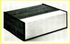
• This new line of enclosures is highly styled and constructed of aluminum wrap-around and molded ABS end panels to provide rigidity, accessibility, and light weight. Two finishes, grey with black or white with wood grain, are available. The two basic sizes available from stock are  $2\frac{1}{2}$ -in, high by  $5\frac{1}{2}$ -in, deep and can be had 4 to 10-in, wide — or  $4\frac{1}{4}$  by  $6\frac{1}{4}$  and 5 to 12-in, wide. Special finishes and punched holes can be provided.
