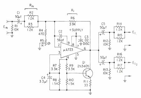
Figure 4. The complete schematic of a line amplifier using a  $\mu A723$ .
