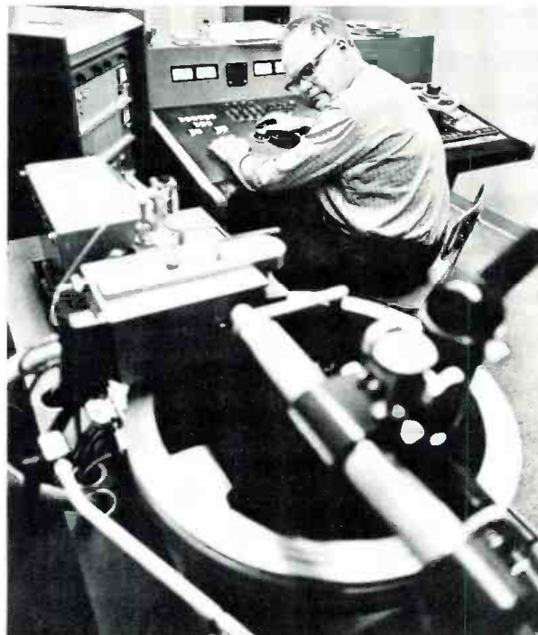
Record mastering is done on a computer controlled Neumann lathe. Robert Berglund is in charge.
