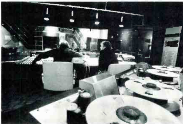
Two sixteen-track machines are interlocked during a 30 track session. The ZPE synchronization system of Sound 80's is used.
