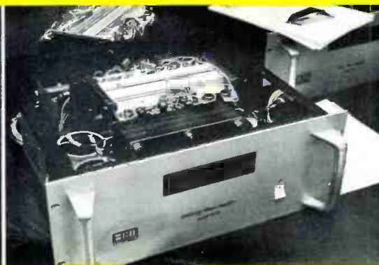
BGW's massive power amplifier has 275 watts across 8 ohms, 550 across 4 ohms, 1500 across 1 ohm. Circle 85 on Reader Service Cards.
