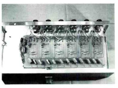
The finished circuit board is installed in the chassis and hard wired to the previously installed pots—finishing the unit.
