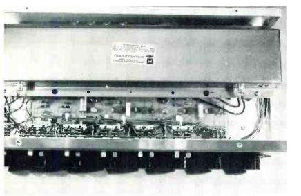
This view from the top of the completed unit shows one channel's output reverb in place and the connectors that join it to the circuits.
