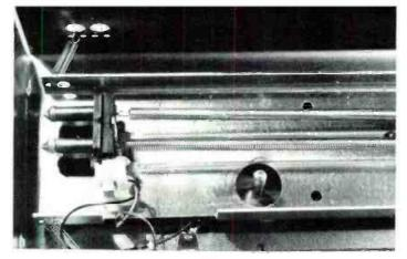
In this closeup the input transformer and terminal of the spring system is shown. This spring system is just for one channel of output.
