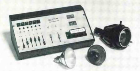
Lightmaster 601 provides a variety of automatically synthesized and manually controlled lighting effects. Six individual channel faders plus two master faders. Plug in modules for sound-to-light, sequence flashing, and random flashing. 117 or 220 VAC, up to 6 KVA power handling capacity...\$595.00.
