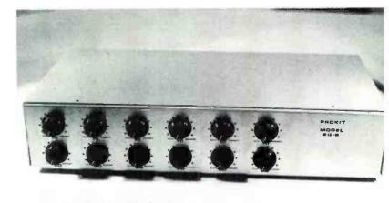
The finished EQ-6 unit. Each vertical pair is one low- and one high-frequency control for the respective channels of the separate mixer.
