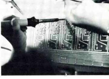
A small pencil iron of low wattage is recommended. A big and hot iron will tend to lift the foil from the glass board.
