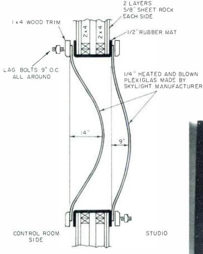
Figure 2. The construction drawing side view. From the front, the window specified is 6-feet, 4-inches across, and 5 feet, 4-inches top to bottom. The window has good dispersion and high rigidity:weight ratio. The windows cost \$85 each and total cost including construction was \$200.
