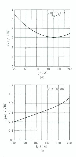
Figure 1. At (A) wideband equivalent input noise voltage versus collector current is shown. At (B) it is current that is shown.
