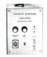
• Almost any oscilloscope may be converted into a real time audio analyzer with the ARA-412 audio response analyzer. Although it is not an impulse analyzer, it can be used to analyze all types of sound which have a less significant time framework. The device covers the audio frequency range from 40 Hz to 16 kHz, with 27 parallel bandpass filters. It has an input impedance of 100,000 ohms high level and 250 ohms microphone level.
