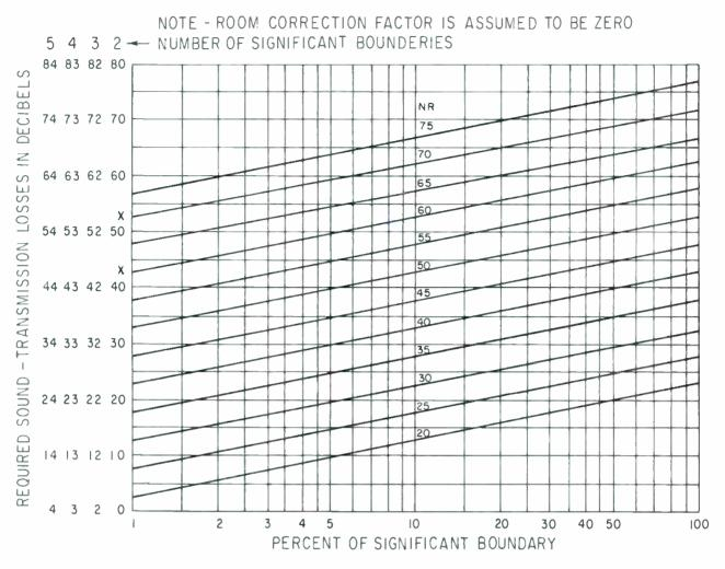
Figure 3. This graph provides quick determination of the required sound transmission losses of elements in a composite barrier to provide various noise-reductions. The abscissa refers to the per cent area of an individual element.
