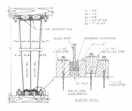
Figure 1. Details of construction of triple-pane sound-retardant window used in monitoring room. The values for the glass thicknesses shown on the figure refer to a large (8 feet x 16 feet) window in a Hollywood motion picture scoring stage.
