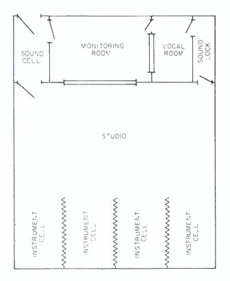
Figure 2. This illustration shows sound-locks, or vestibules, for noise control, and folding partitions for the quick establishment of instrument cells.
