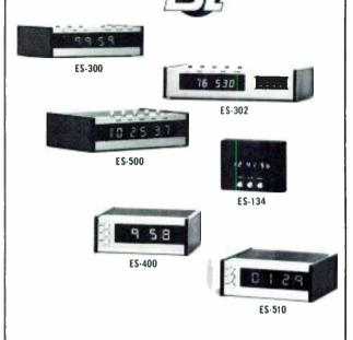
ES-300: A 100 minute up/down timer with incandescent digital display & momentary pushbulton controls on top of an etched aluminum case DIMENSIONS 234" high is 8" wide x 536" deep ELECTRICAL 117 VAC 60 Hz 10W max OPTIONS B.D.G.H.J.K.P.Q.R.S.T.W.Y
