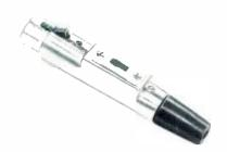
• A momentary "pause" switch on the Q-G (Quick-Ground) f.m. cord plug enables entertainers and broadcasters to interrupt a broadcast for a brief time. The raised knob on the switch permits instant control of the microphone circuit without having to look at the microphone. The subminiature slide switch is built into the connector shell, made secure by a wedging insert screw. The cord plug has a flexible neoprene strain relief, accepts cables up to 0.25 inch diameter.
