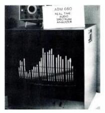
Audio Designs was demonstrating their real time spectrum analyzer that uses a t.v.-type crt tube.
