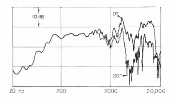
Axial and off-axis (20 degrees) response of an inexpensive (\$15) domestic speaker in a 0.3 cu. ft. cabinet.
