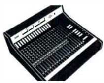
• Flexible BC-5 series production consoles are expandable through the choice of modular plug-in components (770 input and 873 series output modules). The console contains four outputs with individual vus and monitors, cue, foldback and equalizers. It is flexible up to 16 low-level inputs or 28 high-level inputs. There is echo send on all inputs and echo return on all masters.
