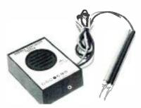
• An audible pitch, varying in tone according to the amount of resistance (0 to 50 ohms) issues from ACT-1 tester while monitoring electrical wiring and electronic circuits. The manufacturer claims complete safety for delicate components, sensitive circuits and semiconductors. Probes produce 2.5V when circuit is open, and 6mA when shorted. Powered by a 9 Vdc battery, the unit measures 23/4 x 1-3/16 x 334 inches. It comes complete with 30-inch probes, battery and alligator clips.
