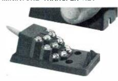
• Twelve-terminal, four-pole, double throw TK-12 transfer key is available in fifteen instrument coordinated colors. The arrangement of the terminal pads in a multi-level design provides positive separation. Contacts are available in gold or silver. The manufacturer also makes similar 6- and 9-terminal keys.
