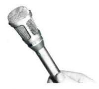
• Designed primarily for sports broadcasts and news remotes, SM82 line-level unidirectional microphone contains its own line-level amplifier, peak limiter, and 9.8V battery. Its balanced line-level output can drive telephone lines or other line-level inputs. Up to a mile of unshielded cable can be used between the mic and the broadcast equipment without equalization. Frequency response is 40-15,000 Hz. Supplied with the unit are a windscreen and a locking swivel adapter.
