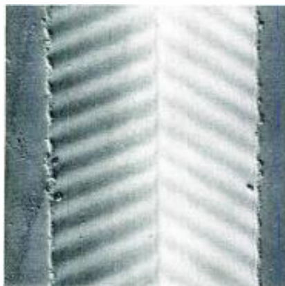
High magnification of a single groove revealing faint parallel lines, probably resulting from imperfections of the original cutting tool. The two rows of debris visible on the "land" at the top of the groove walls are also of interest. (X1000)
