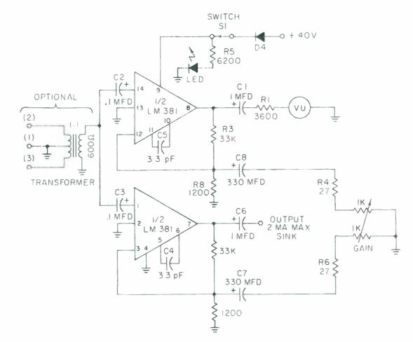
Figure 3. Microphone preamp schematic.
