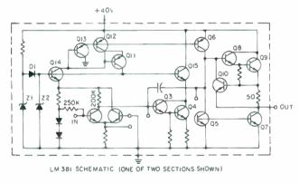
Figure 1. LM381 schematic (one of two sections shown)
