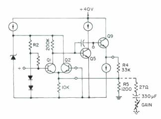
Figure 2. A.C. equivalent circuit.
