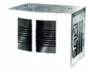
• Exact replacement heads for Gauss (Cetec) type high speed tape duplicating systems are made of hot-pressed glass-bonded ferrite construction. They are designed to replace the original metal 4-track cassette and 8-track cartridge heads in the systems, and are fully compatible with existing Gauss electronics. The manufacturer claims that the new heads will outwear the original metal heads by ten to twenty times.
