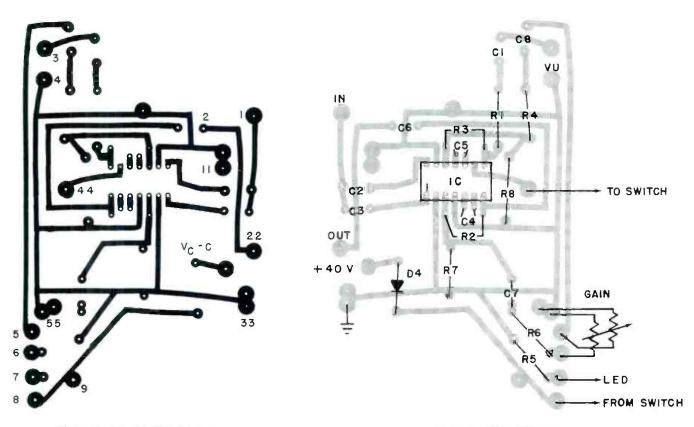
Figure 5. Printed wiring mask.
