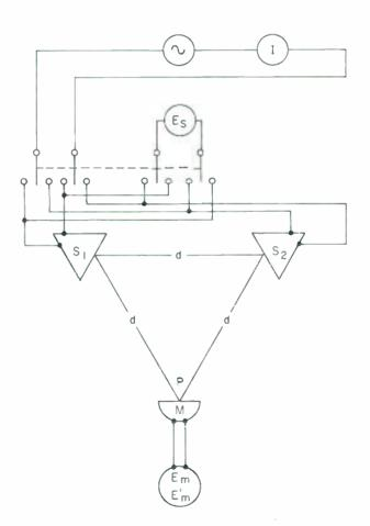
Figure 1. Schematic diagram of the free-field measurement system.
