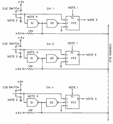
Figure 1. Channel select/control logic.
