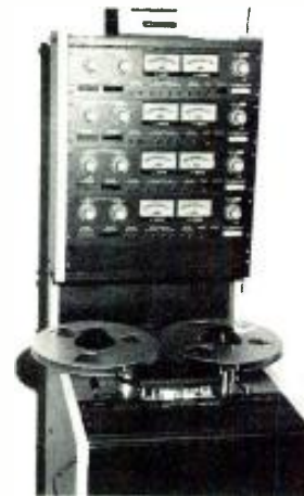
Otari has come up with the MX-5050-8, an 8-track deck using half-inch tape.
