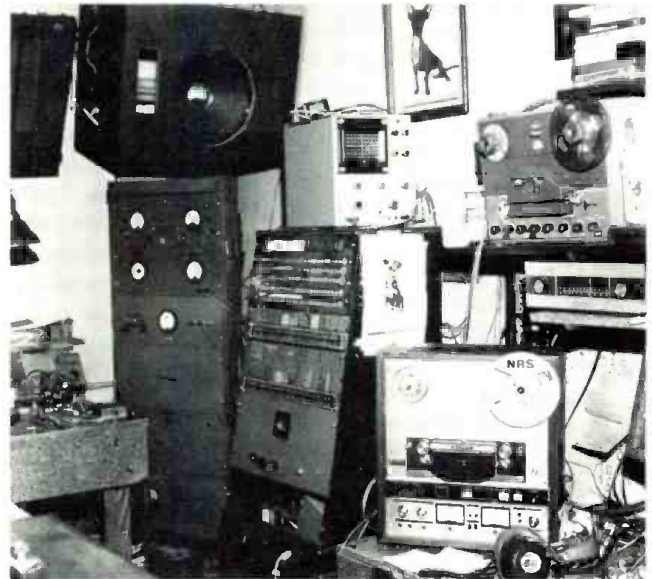
Far left, disc lathe; in the equipment rack top, four meters with hot stylus control; center meter, a.c. control; bottom panels, four power amps. Above the rack, a monitor speaker; below the patchbay, the home-brew compressor. Also, 'scope for positioning, Sony two-track, G.E. am/fm tuner, Newcomb tape deck.
