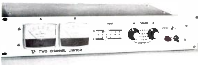
The two channel limiter with variable release time. Stereo coupling is accomplished by a dpst switch which connects the C and F tie points of the two limiters.
