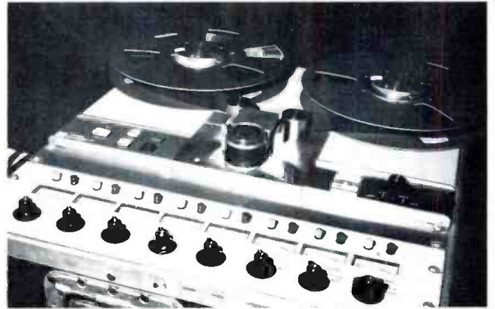
Stephens also produces an isolated multitrack machine, this one featuring eight tracks on one-inch tape.
