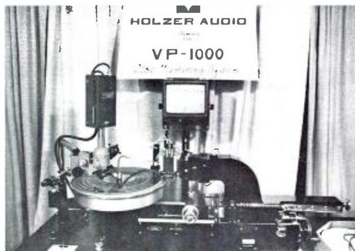
One of the more interesting uses of t.v. is Haeco's hookup to a lathe microscope so everyone can see the cut.
