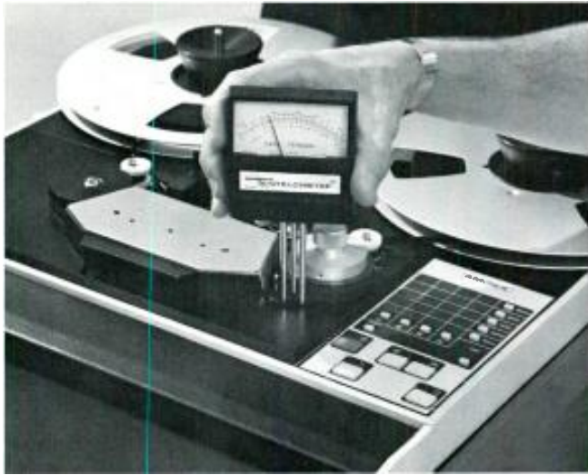
Figure 2. The Tentelometer, manufactured by the author's company, Tentel, is a simple device for the actual measurement of dynamic tension as the tape moves on a transport. By using such a device several times during depletion of the supply reel (as illustrated), tension on a constant torque or constant tension machine can be determined.
