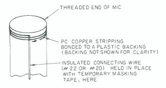
Figure 1. PC copper stripping applied to the microphone shell
