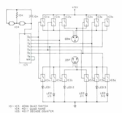
Figure 1. Schematic diagram for the microphone cable tester.
