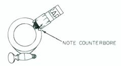
Figure 9. Installation of a screw-mount transducer.
