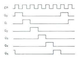
Figure 2. IC5 waveforms.
