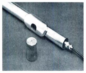
Figure 6. The Type W flute transducer.
