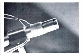
Figure 2. A condenser microphone outfitted with heater.
