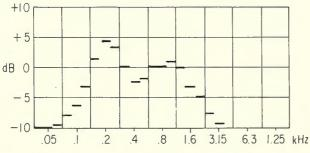
Figure (A). Response of a loudspeaker in a theatre before house equalization.
