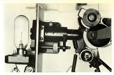
Figure 2. An optical sound head as found on a modern 35mm projector. See Figure 4 for a call-out of parts.
