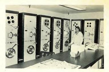
Batteries of magnetic-film recorders and reproducers occupy the machine room at Goldwyn Studios, all locked in sync with the projector and with each other. Photography by R. A. Peterson; Dolbylabs photos.
