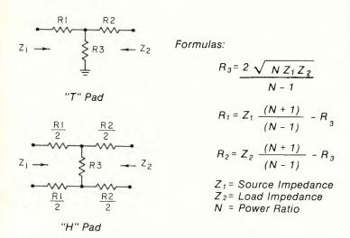
Figure 1. The "T" and the "H" pads. The "H" is the same as the "T", but arranged for balanced circuits.
