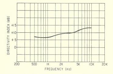
Figure 8. The directivity index for the JBL model 2350 radial horn.
