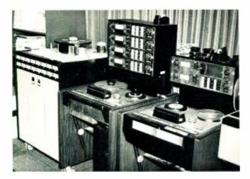
Ampex 2-, 4-, and 16-track tape machines are used in Opryland Productions' television studio operation.
