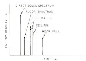
Figure 6A. How ETC data is interpreted. In this example we have marked out the direct sound plus the floor, ceiling, and rear wall reflections.
