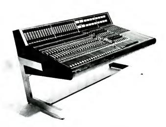
The Trident TSM Series console featuring 24-inputs with fully removable modular patchbay.
