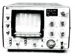
The Hewlett-Packard 3580A spectrum analyzer.
