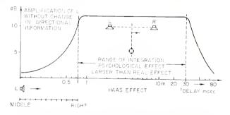
If a person sitting symmetrically between two identical noise sources L and R receive exactly the same sound impulse from both sources, it appears to him that there is only one sound source midway between L and R.
