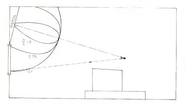
Figure 1. Directional radiation characteristics of a circular piston in an infinite baffle for various ratios of piston diameter to wavelength of generated sound.
