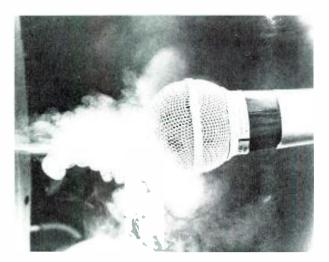
feet-per-second. By comparison, a 100 Hz sound wave with a sound pressure level of 100 dB attains a peak particle velocity of only 0.03 feet-per-second. Wind is also a moving mass of turbulent air and affects the microphone much like pop, except over a broader frequency range, and over a greater area.
