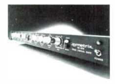
• A new audio processing device designated the SG-200 dual signal gate, was recently unveiled. The SG-200 contains two totally independent gates sharing a common power supply in one, 1¾-inch high, rack mount chassis. Operating controls for each gate include attack time, release time, range of attenuation, threshold, a totally silent in/out switch, and an internal/external gating command control.
