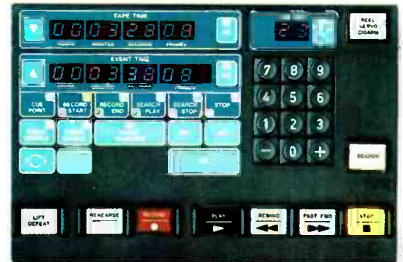
ATR-124's Multi-Point Search-To-Cue (MPSTC). Provides 100 cue locations.
