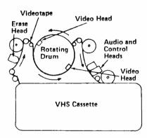
Although Beta and VHS Systems employ different tape loading systems, both use stationary audio recording and playback heads.
