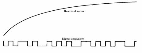
Figure 1. A baseband audio signal with its digital equivalent.
