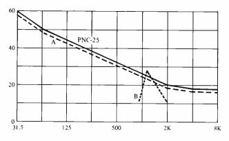
Figure 3. Noise A is rated less than PNC-25, and should be considered acceptable; yet it has an A-weighted sound level of 35 dB-A. "Non-acceptable" noise B exceeds PNC-25, but has an A-weighted sound level of only 26 dB-A.
