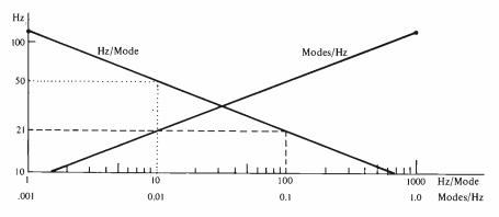
Figure 1. The average frequency space between modes (Hz/mode) for a control room of 5000 ft³ volume, as a function of frequency. For example, at 50 Hz, a frequency space of 10 Hz exists between modes (dotted line). At 21 Hz, the modes are 100 Hz apart (dashed line).
