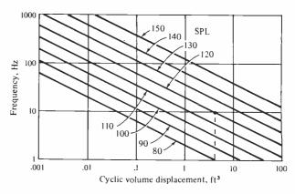
Figure 6. The cyclic volume displacement required for a baffled piston to generate the indicated sound pressure levels at a distance of 10 feet. For example, for a 10 Hz signal, a cyclic volume displacement of 4 ft³ is required to produce a SPL of 120 dB at a distance of 10 feet from the speaker.
