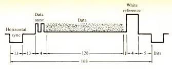
Figure 3. The complete contents of one horizontal line, including standard NTSC video sync components.
