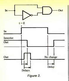
If we run the input from H to L, there will not be any response from the AND gate, since both its inputs are L for this instant. Since the AND gate has the same output when one or both inputs are L, the output does not show the same kind of temporary H output.
