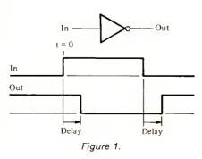
which all other sequential logic is built. It is not obvious from this definition, but the basic flip-flop itself can be built from combinatorial logic. To do so, we introduce the concept of time in our simple combinatorial logic, for it is not quite true that the output is determined *only* by the present input.
