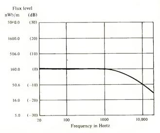
Figure 1. Short Circuit Flux Level versus Frequency for the NAB  $50/\infty$  microsecond Time Constant.
