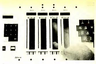
Figure 3. The fader computer recognizes only finger movement, and not where it is positioned in the infra-red field.
