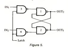
the circuit to a given state. When these inputs are both brought back to H, then the circuit can remember that state. This is a very primitive flip-flop, but it forms the basis of more complex circuits. FIGURE 5 shows a modification to the circuit, with the addition of two extra NAND gates (3, 4) to feed the R and S inputs (IN<sub>1</sub> and IN<sub>2</sub>) of the previous circuit.
