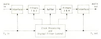
Figure 2. Block Diagram of the SFC-16. The real-time control signals for the operation of the sampling frequency converter are obtained by digital processing of the clock signals, and so it is not necessary to program the converter for any particular ratio of sampling frequencies.
