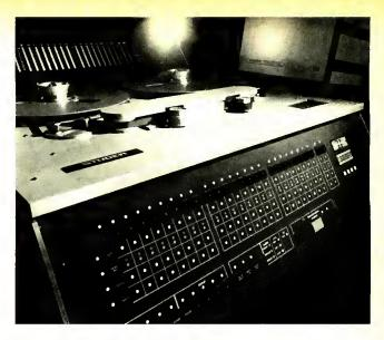
Figure 3. Studer's entry in the digital arena: 24 audio tracks on half-inch tape at 30 ips.
