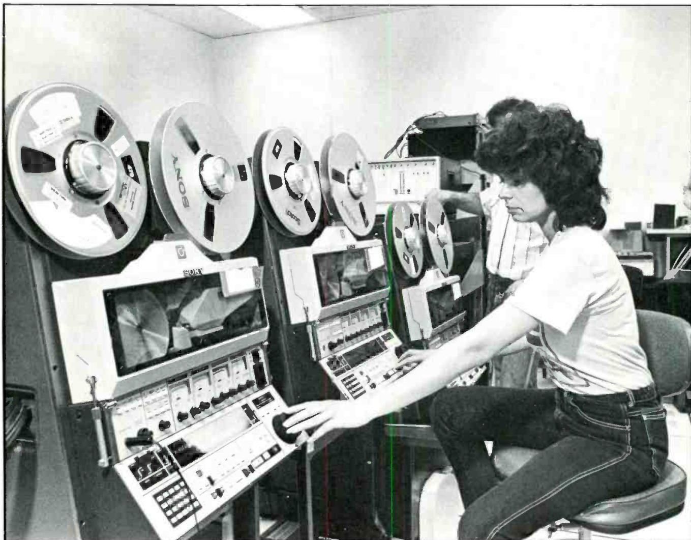
Showtime's video tape operator, Pat O'Grady, at the Sony BVH-2000 1-in. video tape machines.
