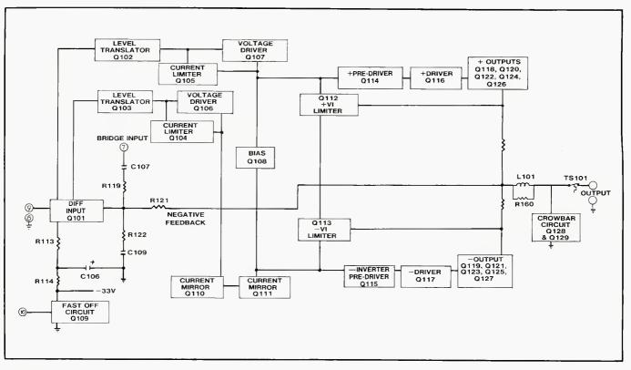
Block diagram for amplifier Model 8000.
