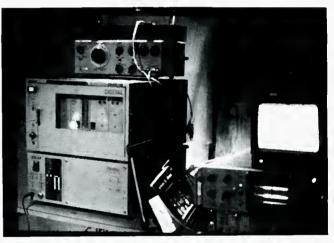
In this view of other transmission equipment we can make out the Sony 160 and 1630 units. The picture monitor and wave-form monitor is also seen.
