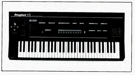
allow manipulation of filters, amplitude, and the relative mix of the 4oscillators per voice. Looping and repeat functions enhance the power of patch programming. Other features include real time control of stereo panning, voice oscillator mixing, stereo chorusing and instant access to 200 programs via ROM and RAM cartridges. The five-octave synthesizer is velocity and pressure sensitive and can
