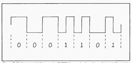
Figure 2. Bi-phase modulation used in SMPTE time code. A voltage change in the middle of a half-cycle (bit number) signifies a binary 1; no change signifies a binary 0.
