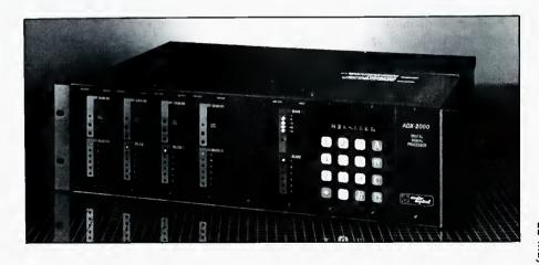
Delay settings range from 10 microseconds to 261 milliseconds (1048 milliseconds optional) in increments of one micro- or millisecond. Dynamic range is at least 100 dB (A-weighted, no companding); THD plus noise is better than 0.1%; and frequency response is 20 Hz-20 kHz. Additional modules which will further broaden the ADX-2000s capabilities are forthcoming. Mfr: Audio/Digital, Inc. Price: \$3,500.00 for standard configuration. Circle 55 on Reader Service Card
