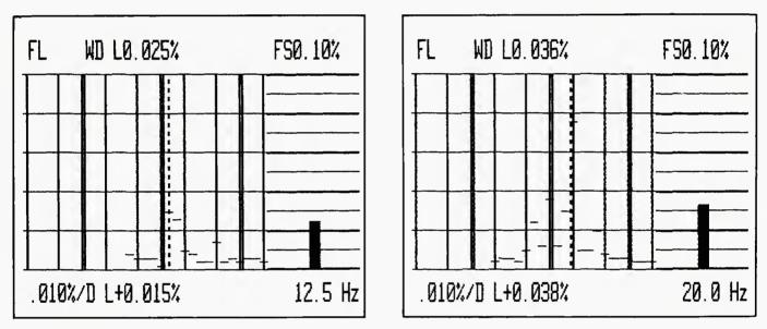
Figure 8. Wow-and-flutter at 3 3/4 ips (A) and at 1 7/8 ips (B).
