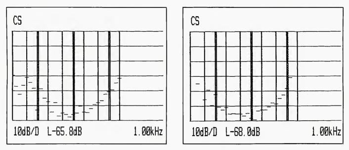
Figure 10. Channel separation vs. frequency at 3 3/4 ips (A) and at 1 7/8 ips (B).
