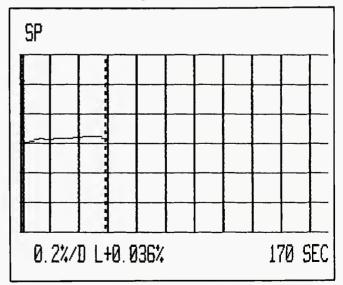
Figure 11. Tape speed accuracy, at 1 7/8 ips.
