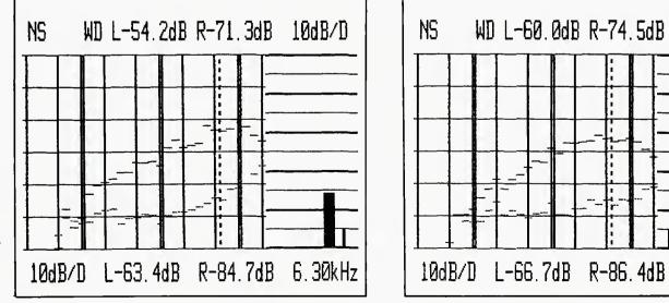
Figure 6. S/N analysis, without and with Dolby C, at 3 3/4 ips (A) and at 1 7/8 ips (B).
