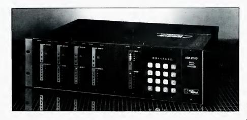
Delay settings range from 10 microseconds to 261 milliseconds (1048 milliseconds optional) in increments of one micro- or millisecond. Dynamic range is at least 100 dB (A-weighted, no companding); THD plus noise is better than 0.1%; and frequency response is 20 Hz-20 kHz. Additional modules which will further broaden the ADX-2000s capabilities are forthcoming. Mfr: Audio/Digital, Inc.
