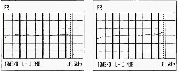
Figure 3. RECORD/PLAY frequency response with Dolby B N/R, at 3 3/4 ips (A) and at 1 7/8 ips (B).
