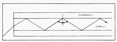
Figure 2. (top) Light entering from left into core with index  $n_1$  reflected at the boundary with the cladding having index  $n_2$ . [page 21 from AMP] (bottom) various paths for light ray in different types of fiber optic cables. The core size and refractive index determine the light propagation characteristics of the fiber. [page 23 from AMP].
