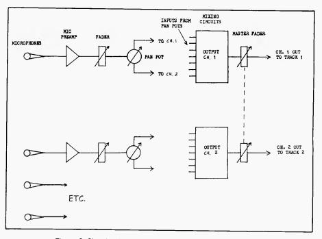
Figure 2. Signal paths in a typical 2-channel mixers.
