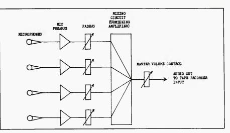
Figure 1. Signal paths in a typical mono mixer.
