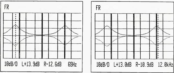
Figure 12. Response of system with low and high frequency EQ controls set to one extreme and EQ level controls next to
