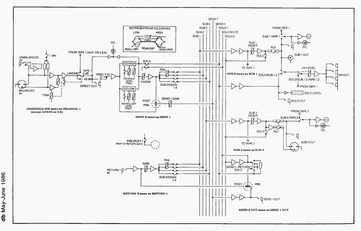
Figure 1. Block diagram of the mixer section.
