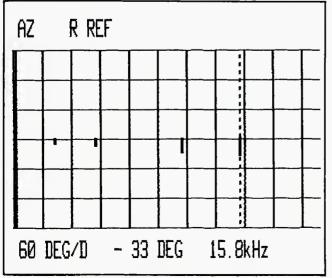
Figure 9. Azimuth alignment accuracy during playback of calibrated azimuth alignment tape at 1 7/8 ips.
