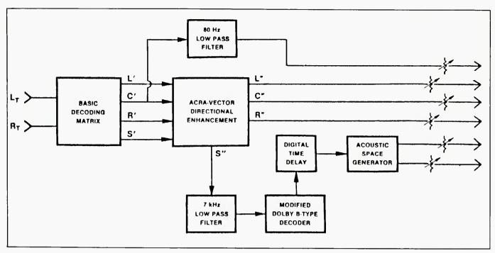
Figure 5. Block diagram of the HTS 5000 in the Dolby Surround mode
