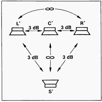
Figure 4. Interspeaker leakages of the Dolby Surround Matrix before directional enhancement.
