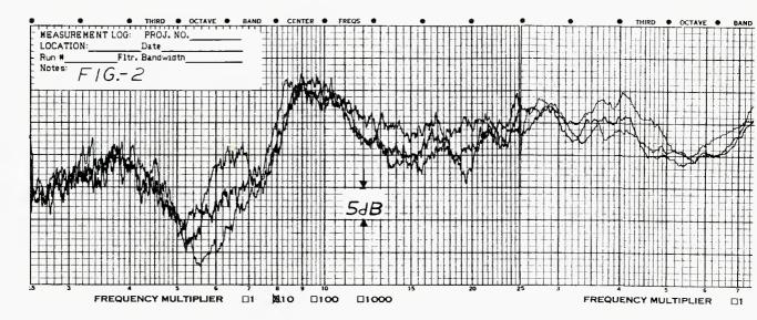
Figure 2. The monitor response measured in a control room in which reflected energy is returned in the
