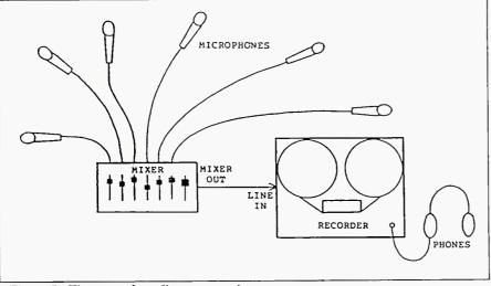
Figure 5. The setup for a live mono mix.
