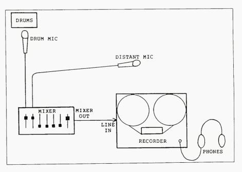
recording level. Play back the tape. Even though you recorded at a moderate level, you're likely to hear distortion caused by the microphone signal overloading the mic preamp in the tape recorder. Insert a pad in the microphone cable (such as a resistive voltage divider with 20 dB loss) and repeat the recording. The distortion should be eliminated.
