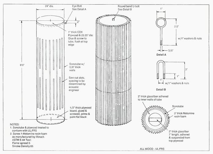
Figure 10. A detailed construction diagram of Helmholz tube-type resonators.
