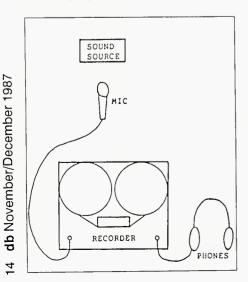
tortion and too-low levels make tape hiss audible. Note that percussive instruments require lower recording levels for undistorted recordings than do non-percussive instruments.
