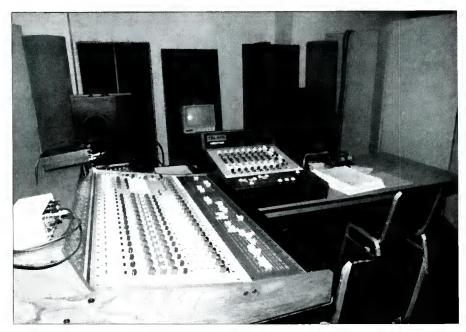
Figure 3. The Neotek console and monitoring equipment.
