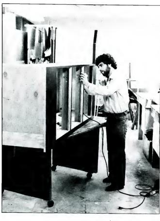
Figure 4. The author is seen finishing the front of the new rack. Steel reinforcement was added to withstand the weight load.
