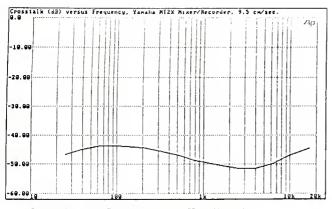
Crodestalk versus Frequency, Yamaha MTZX Multitrack Cassetta Recorder, at 9.5 cm/uac. (adjacent tracks Figure 11.
