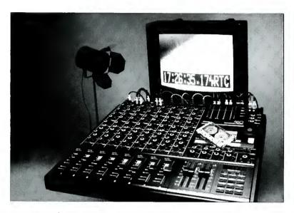
• The Fostex 460 is the company's top-of-the-line recorder/mixer. It includes a 4-track cassette recorder built into a complete 8-input mixer.
