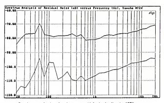
Spectrum analysis of noise, record/playback, Yamaha MT2X, Upper trace without dbx, lower trace with dbx ON, 9.5 cm/sec  $Figure\ 9(B).$
