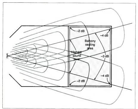
Figure 7. Overall coverage in the balcony from two horns.
