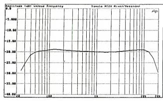
Frequency Response, record/play at 4.8 cm/sec, -20 dB record level. Yamaha MY2X Multitrack Cassette Recorder
