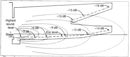
Figure 2. An overlay showing vertical dispersion for a typical horn application.
