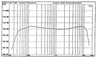
Frequency Response, record/play at 4.8 cm/sec, -20 dB record level, dbx ON, Yamaha HT2X Multitrack Cassette Recorde
