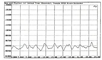
Wow and Flutter for a test period of 30 seconds, record/playback Yamaha MY2X Multitrack Cassette Recorder, 9.5 cm/sec.
