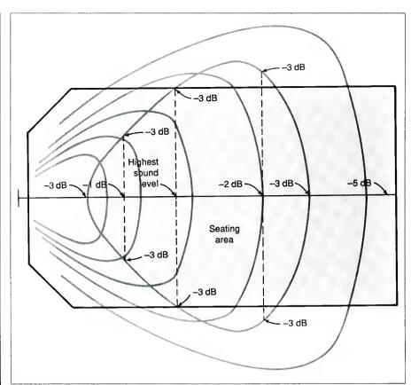
Figure 5. Horizontal dispersion and overall coverage contour.
