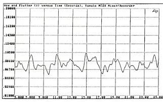
Wow and Flutter for a test period of 30 seconds, record/playback Yamaha MT2X Hultitrack Cassette Recorder, 4.8 cm/sec.
