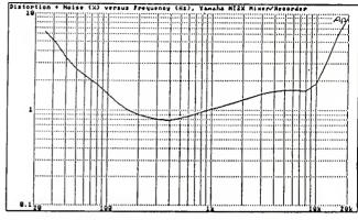
Distortion vs Frequency Yamaha HT2X Multitrack Cassette Recorder, at 9.5 cm/sec. dbx ON.
