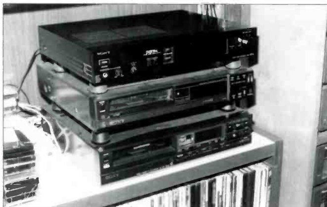
Figure 10. Sony F-1 equipment serves for the recording and the mastering.
