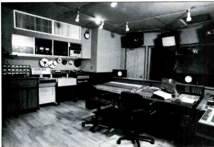
Figure 9. Studio 5 with its Harrison 4032 with Auto Set and a 3-machine lock up.
