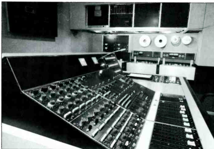
Figure 10. An 18-year-old Neve discrete console. It has been renovated with an extended patch bay and 4-track monitoring.
