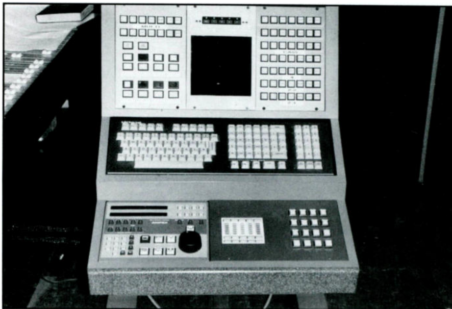
Figure 13. Master switching console.
