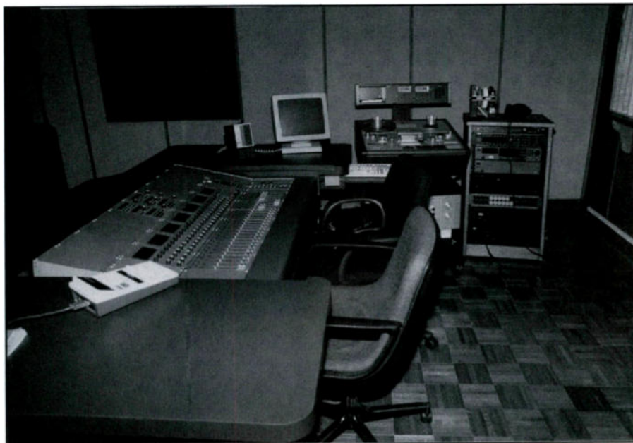
Figure 1. A Daniel Weiss Digital Console dominates this mix room at New York City's Sony Classical suites.
