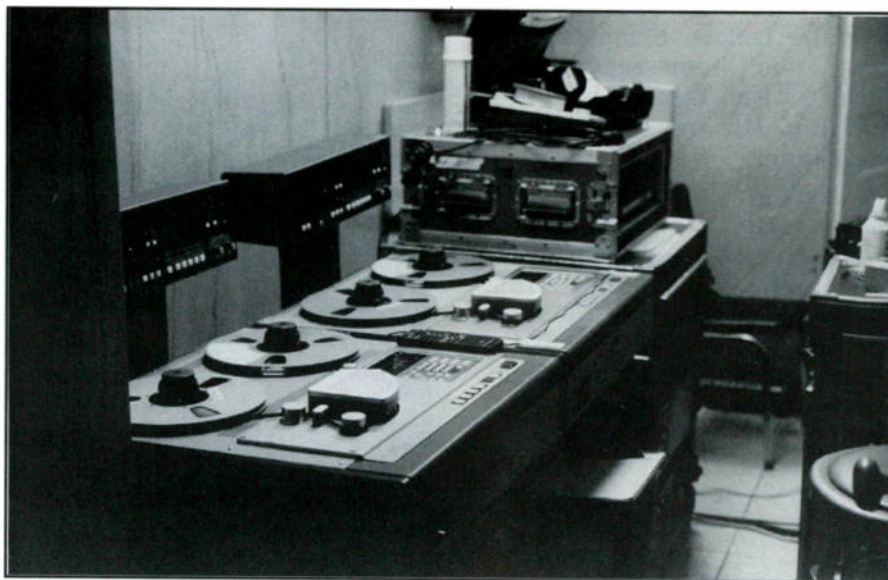
Figure 3. For a recent Emanuel AX recital of works by Beethoven and Brahms, stereo mixes being recorded on 20-bit two-track Sony PCM-3344 Twin-DASH recorders, with a greater than 105 dB dynamic range.
