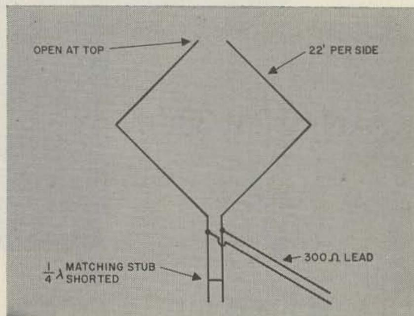
Fig. 1. Bi-square antenna for 15 meters. A horizontally polarized, broadside, bi-directional array with a gain of about 4 db. It is constructed with ordinary antenna wire and fed with twinlead. It requires only one 35 foot (or taller) pole for support.
