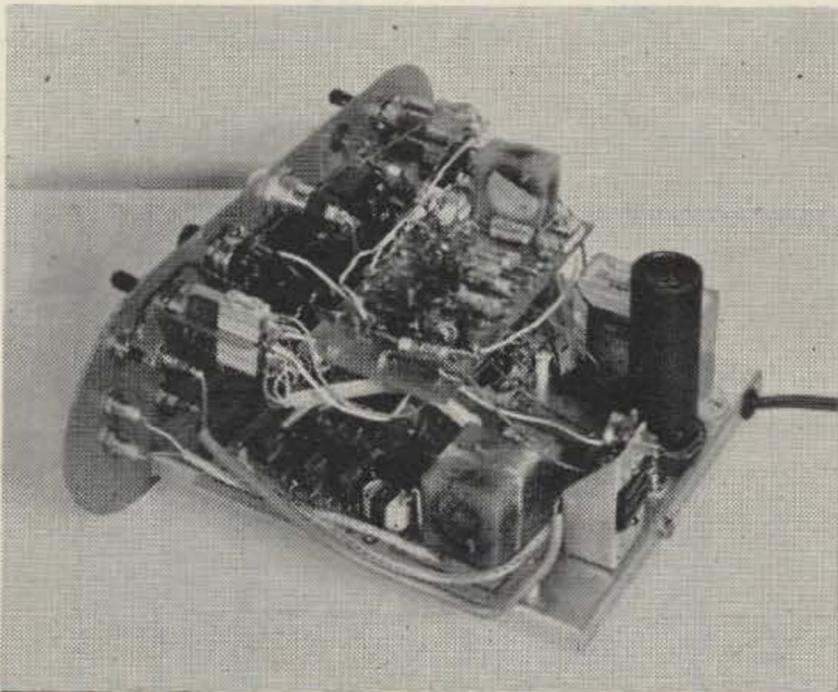
space filter is tuned to 2975 cps. This takes a total capacity of about 0.033 mfd, and about 0.068 mfd capacity for 2125 cps for the other toroid. We may note here that when tuning these two toroids they should be mounted on the board and in the circuit. An audio signal is applied to the input at the frequency each of the toroids is to be tuned to. Watch for a peak on a V.T.V.M. across the toroid being tuned. NOTE:
