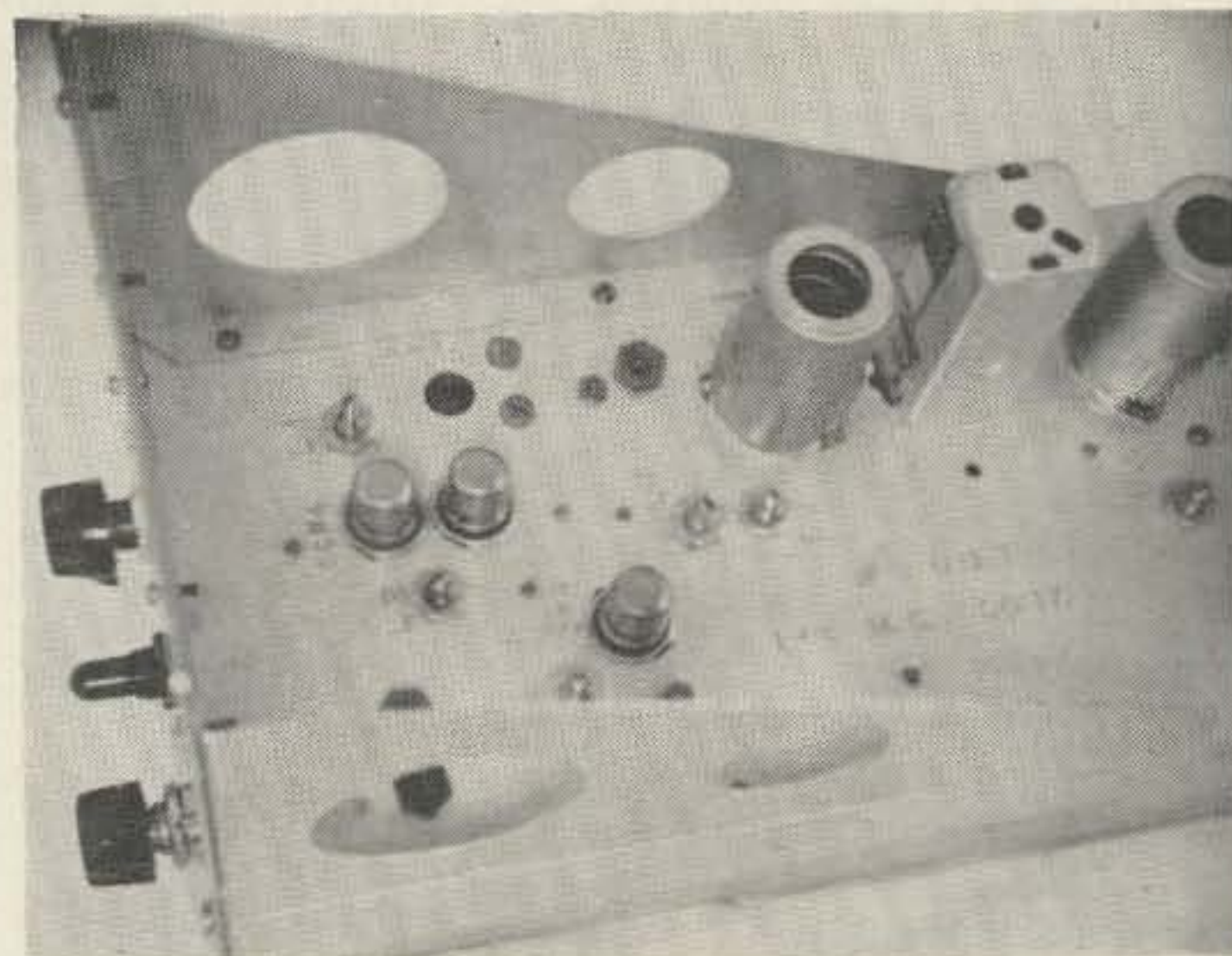
Enlarged top view of the front end showing the arrangement of nuvistor and coils. The first large tube in the upper right is the 6AK5 mixer.
