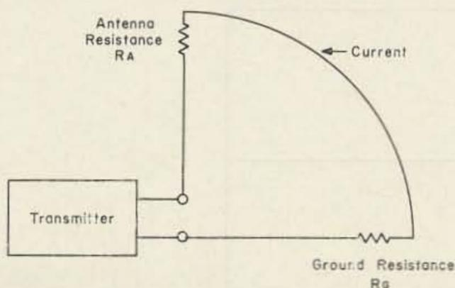
Transmitter Output is Dissipated Proportionately Between  $R_A$  &  $R_g$
