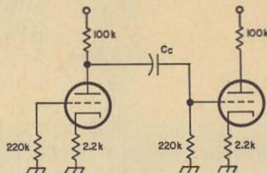
Fig. 1. Two stages of audio, resistance coupled.
