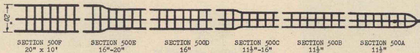
Fig. 2. Typical TV tower sections available.
