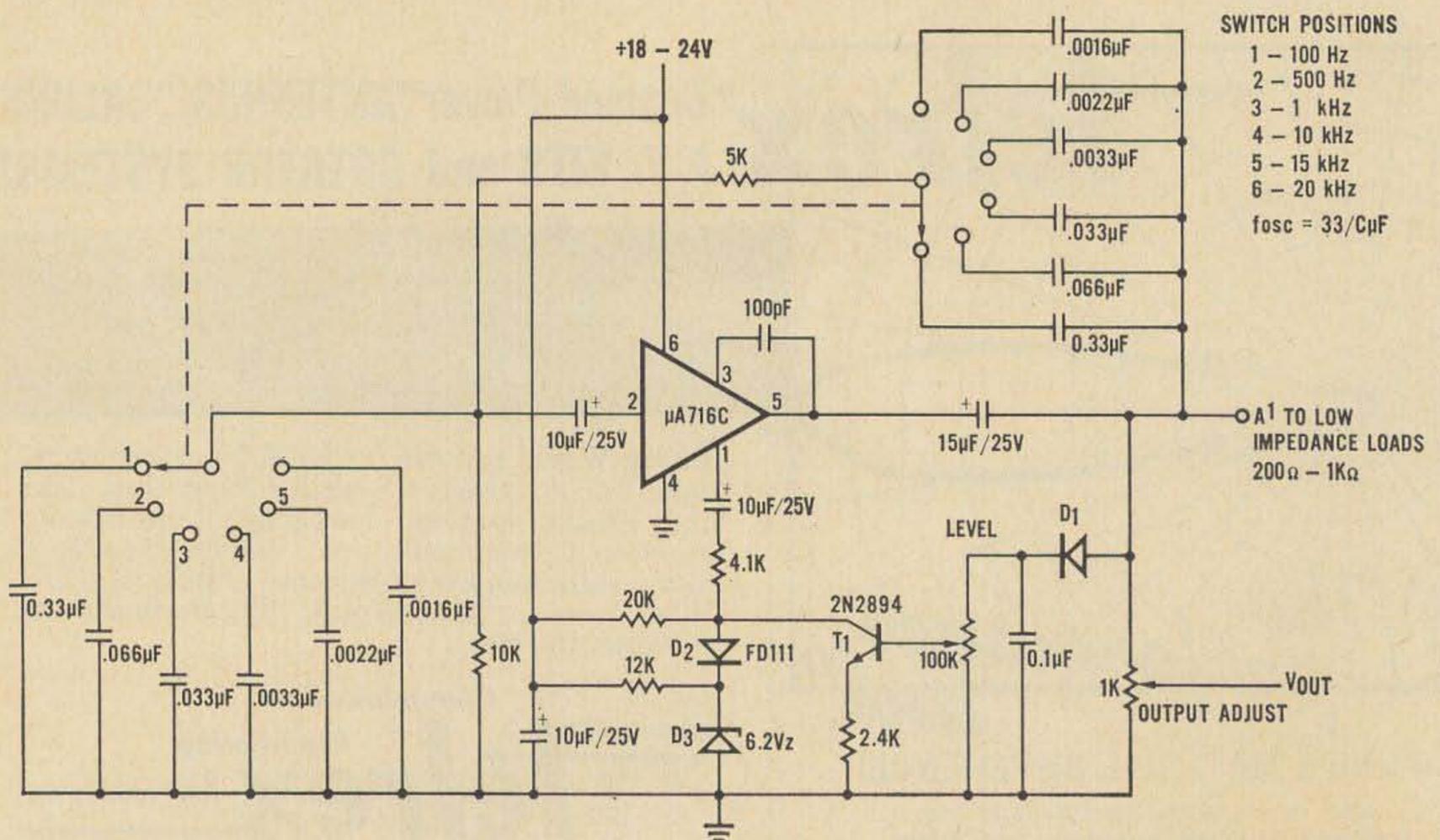
Fig. 1. The complete schematic of the oscillator.
