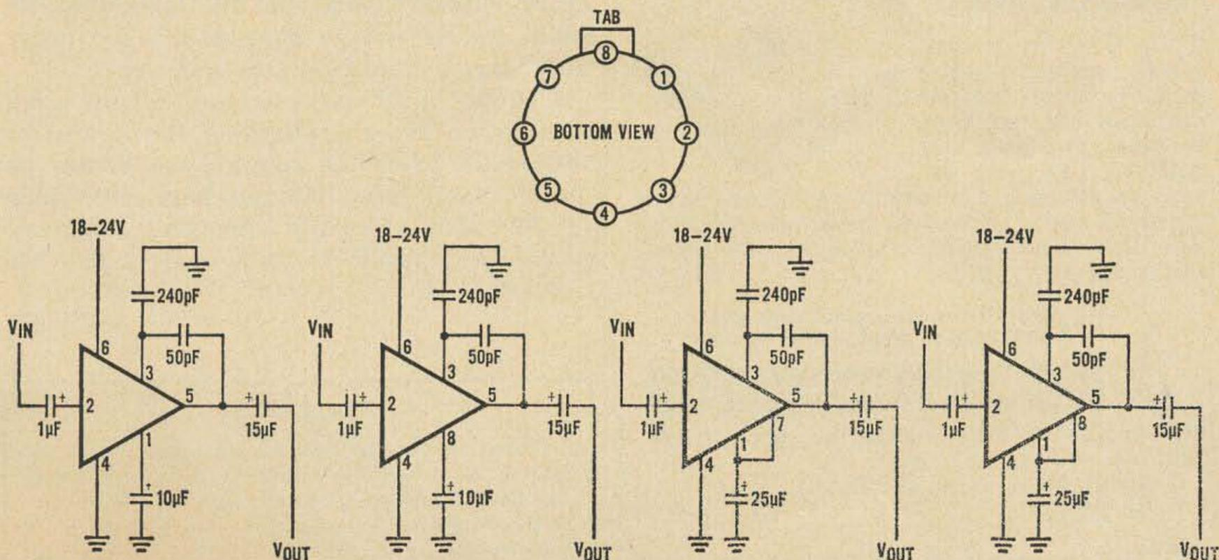
Fig. 4. Diagram showing connections for the  $\mu A716C$ .
