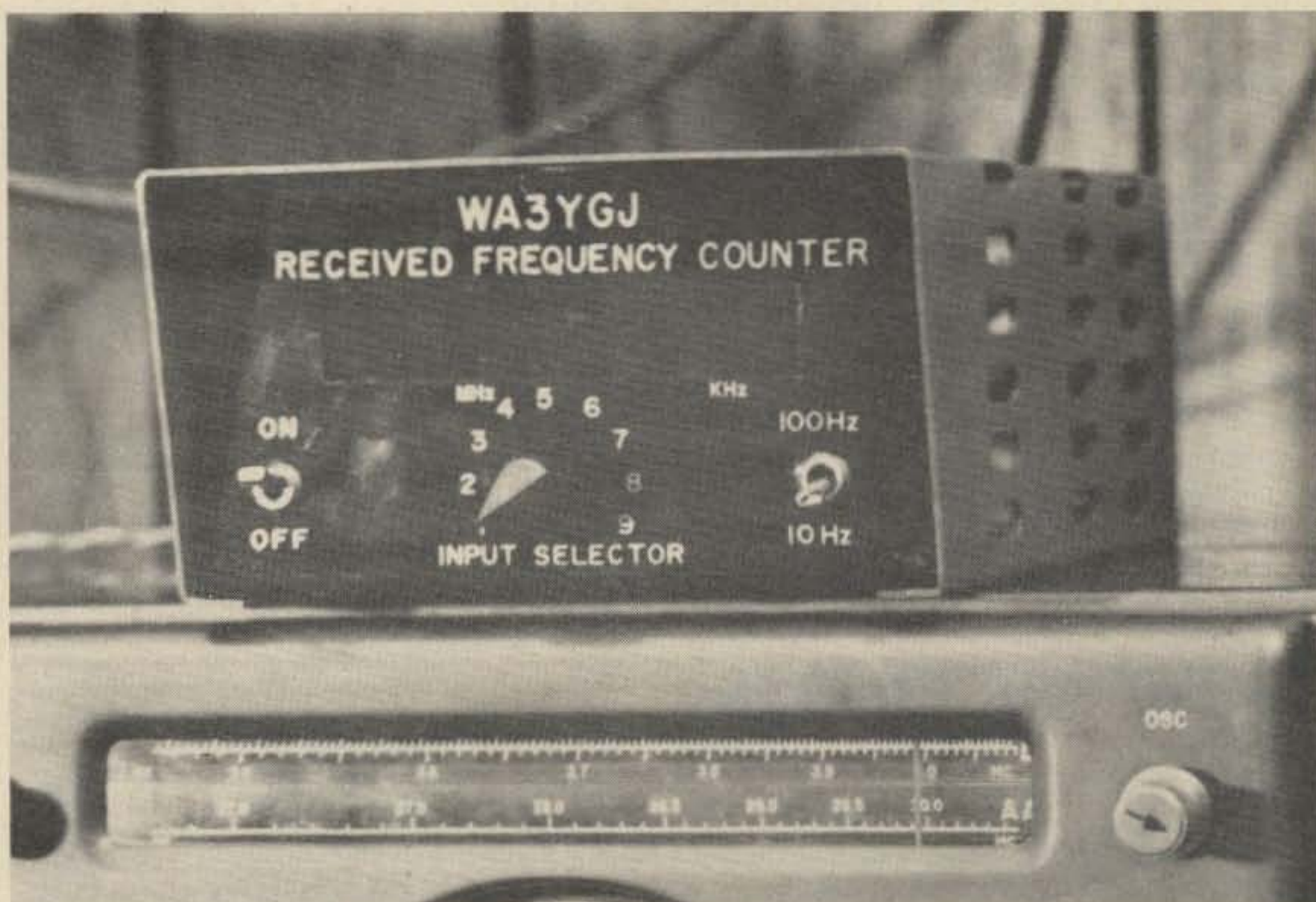
The received frequency counter shown in place on top of my HRO-50T receiver. This chassis contains all of the circuitry described in the article except the crystal oscillator, power supply, and multiple radio interface. These are still in breadboard form and are not shown for aesthetic reasons.
