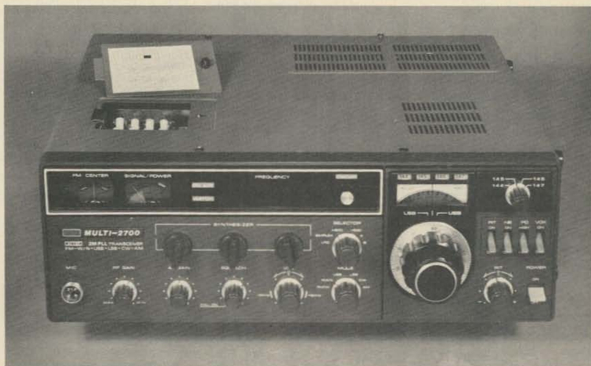
A clean layout — with VOX, AGC and gain controls accessible through top port.
