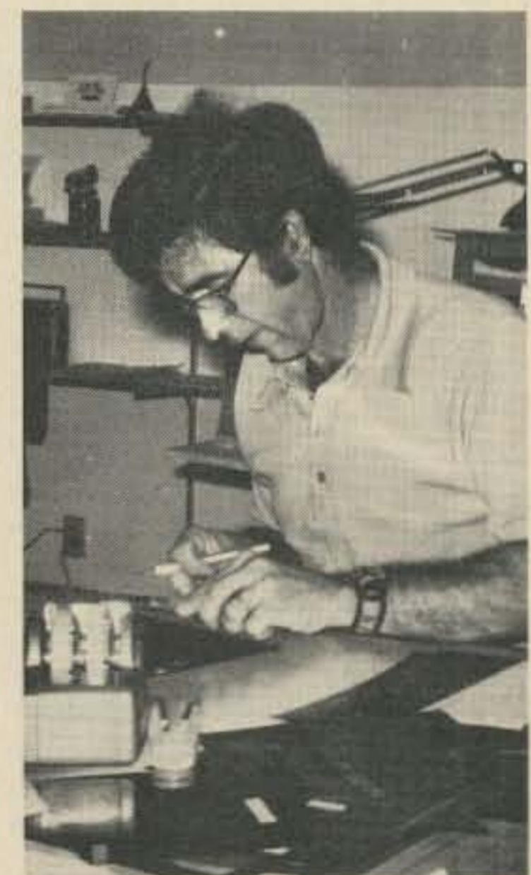
Noel Ray Self is working on negatives for 73 Magazine and for the latest 73 books. Photographs have to be made separately and glued onto the negative of the type and drawings ... a job requiring great precision. Negatives are never perfect, so Ray has to find all pin holes and go over them with paint to opaque them. Where ads are placed on pages, negatives have to be spliced together. Duplicates are then made on single sheets of film. Ray does the splicing ... also adding the page numbers at the bottom ... etc.
