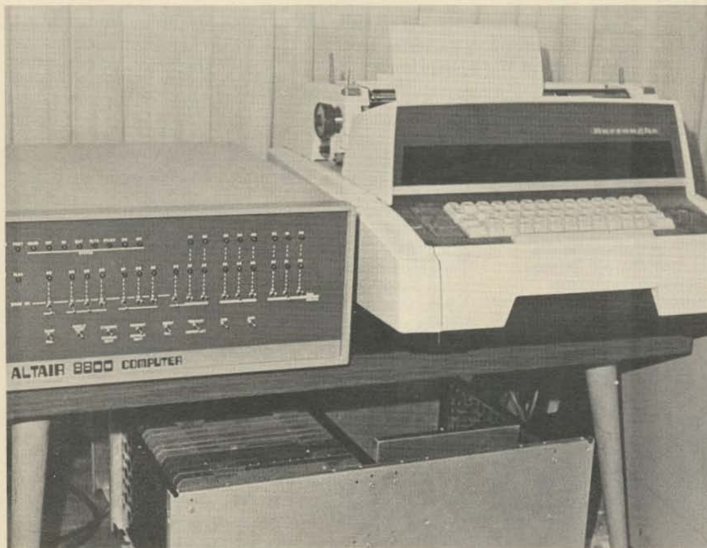
The Altair/Friden system. The 8800 is sitting next to the Friden TM 20K714 keyboard-printer. The TM 20K715 controller (without its cover) is visible under the table.
