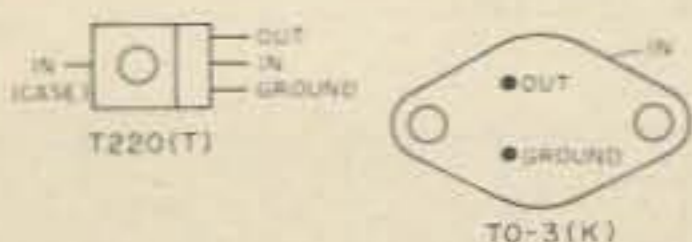
Fig. 5. LM320T(K) negative voltage regulator. LM320T(K) (5.0, 5.2, 6.0, 8.0, 12, 15, 18 or 24).
