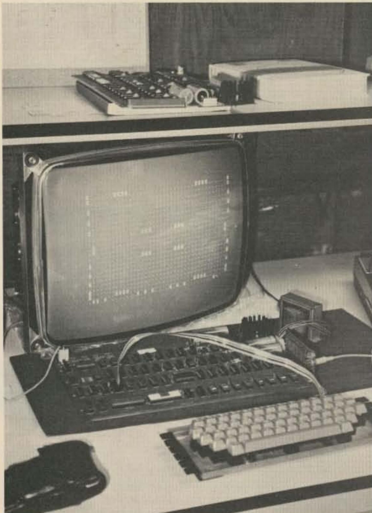
Here's the Apple computer system up and running a game of Life. Note the tiny cassette I/O board at the right! This is a complete computer and video generator, all on one board. Any wonder there was a lot of interest in this system at PC-76?
