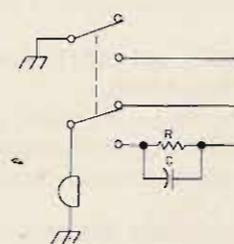
Fig. 3. A better filter for transmitting . . .
