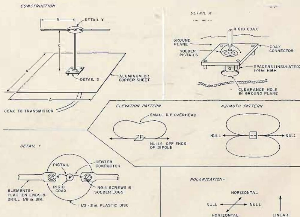
*Fig. 2. Dipole over ground plane.*
