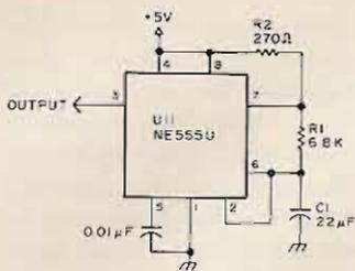
Fig. 2. Basic clock circuit.
