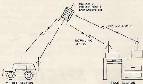
Fig. 1. Mobile to base station operation via satellite.
