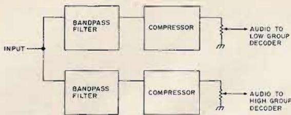
Fig. 4. Block diagram of input conditioning scheme.
