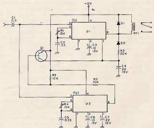
Fig. 2. Complete schematic of the two tone latching decoder.
