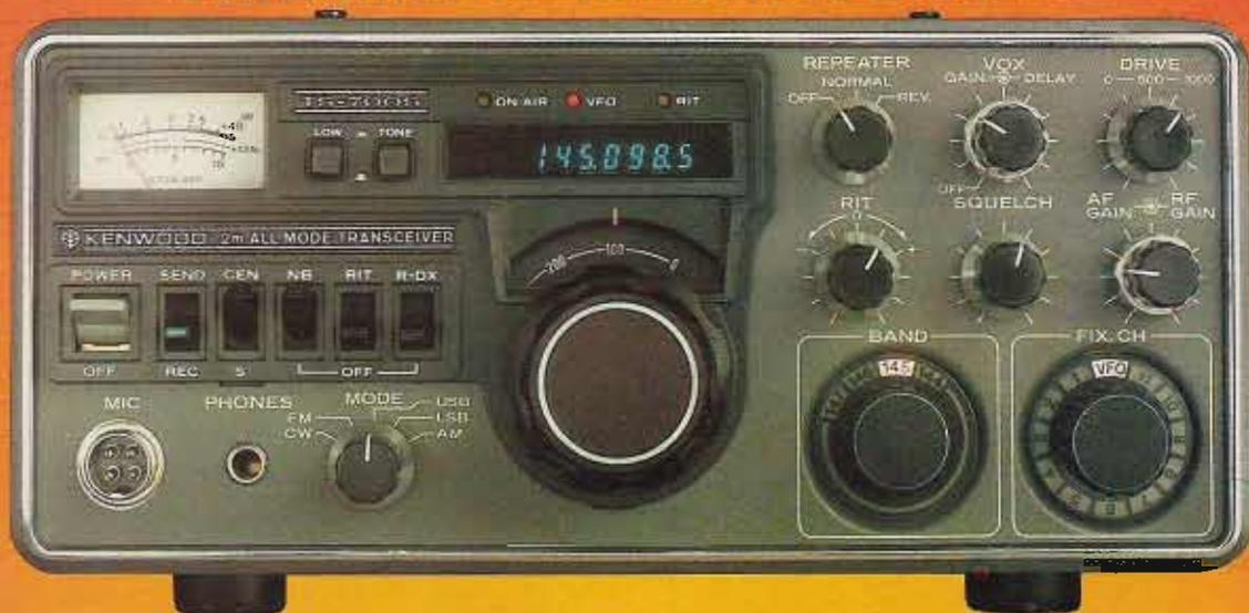
Kenwood has done it again! We've combined the fine, time-proven characteristics of the original TS-700A together with many of the ideas and comments for improvement from amateurs worldwide. Check out the new "built-ins": digital readout, receiver pre-amp, VOX, semi-break in, and CW sidetone! Of course, it's still all mode, 144-148 MHz and VFO controlled.
