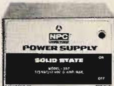
Functions silently in converting 115 volts AC to 12 volts DC. 4 amps continuous, 6 amps max. Enables anyone to enjoy CB radio, car 8-track cartridge, cassette player or car radio in a home or office.
