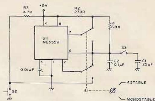
Fig. 3. Modified clock circuit.
