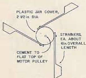
Fig. 1. Advanced design wind vane assembly.
