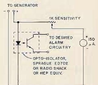
Fig. 2. Remote indicator. Alarm circuitry might be a 6 volt battery in series with a Mallory Sonalert, for example.
