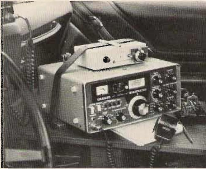
Transceiver as in Fig. 3 showing the tunable receive converter on top of the FT101.
