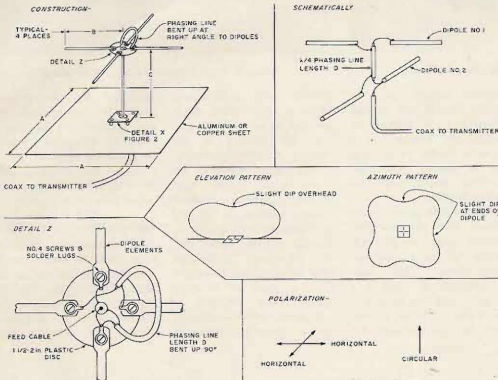
Fig. 3. Turnstile over ground plane.
