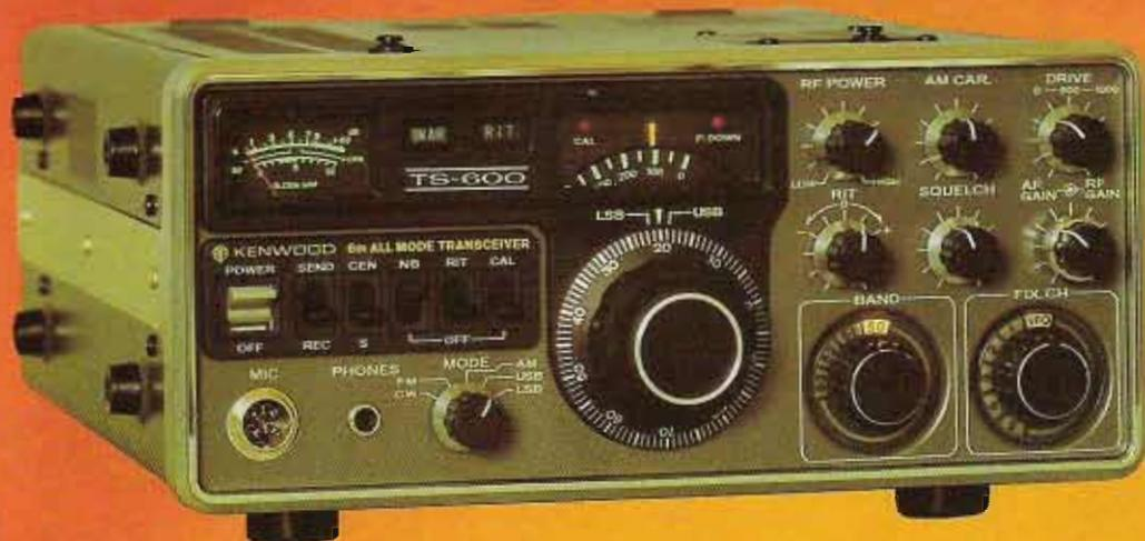
Experience the excitement of 6 meters. The TS-600 all mode transceiver lets you experience the fun of 6 meter band openings. This 10 watt, solid state rig covers 50.0-54.0 MHz. The VFO tunes the band in 1 MHz segments. It also
