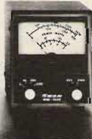
**WM1500** High-Accuracy In-Line Wattmeter. 10% full scale accuracy on 5, 50, 500 and 1500 watt scales, 2 to 30 MHz. Forward and reflected power. Use it for trouble-shooting, too. \$74.95
