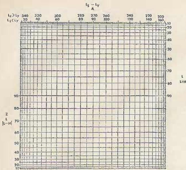
Fig. 3. Simplified d'Ocagne chart. All scales are expressed in degrees.  $L_s$  = satellite subpoint longitude;  $L_y$  = your longitude;  $A$  = azimuth angle;  $Z$  = zenith angle;  $L$  = your latitude; and  $H = 90^\circ - Z$ .
