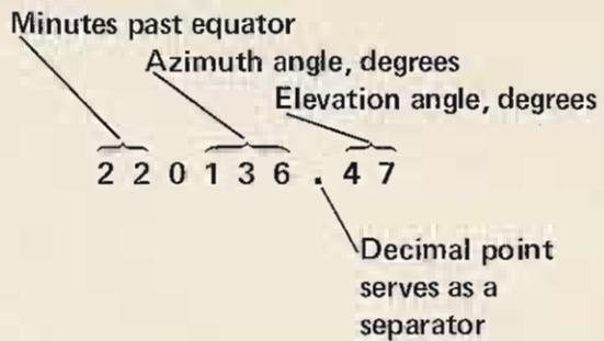
Fig. 1. Typical merged display.
