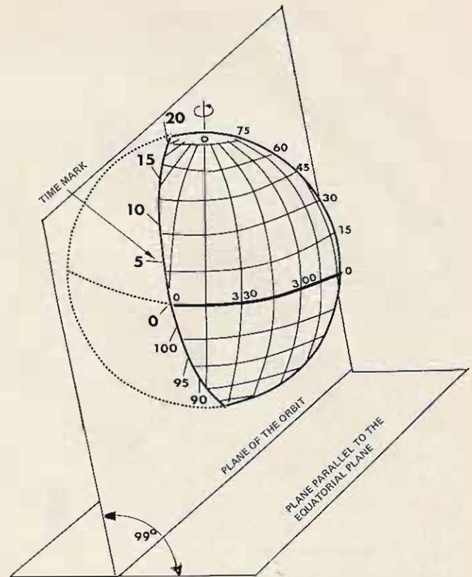
Fig. 3. Simulated Earth track on a plane inclined 99° from the equator (static Earth). Note that the orbital plane is fixed in space and the Earth rotates inside this plane from west to east (counterclockwise as viewed from a point above the North Pole).
