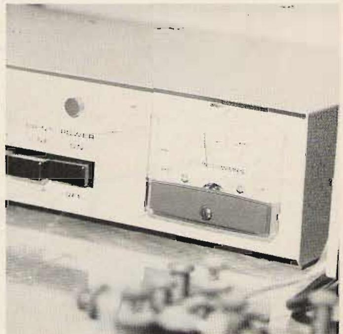
Many modern terminal units use a meter for tuning. A steady value indicates a properly tuned RTTY signal. Once the signal is tuned, the printer can be activated. The TU pictured is the HAL ST-5000.
