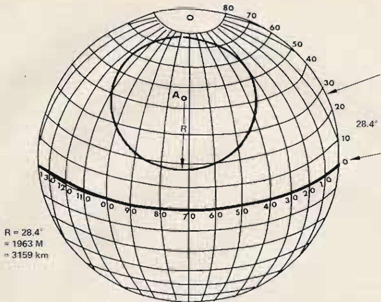
Fig. 9. Area of accessibility. The satellite will be available for communication when its subsatellite point is found inside the circle of accessibility.
