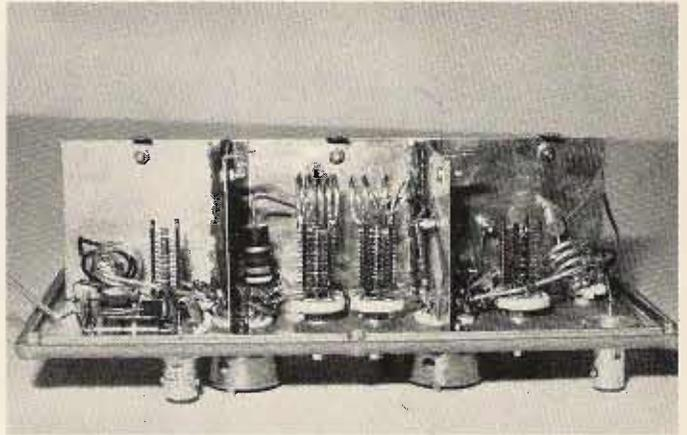
Transmitting converter amplifier and mixer. Note intercompartmental shielding utilized to insure stability.
