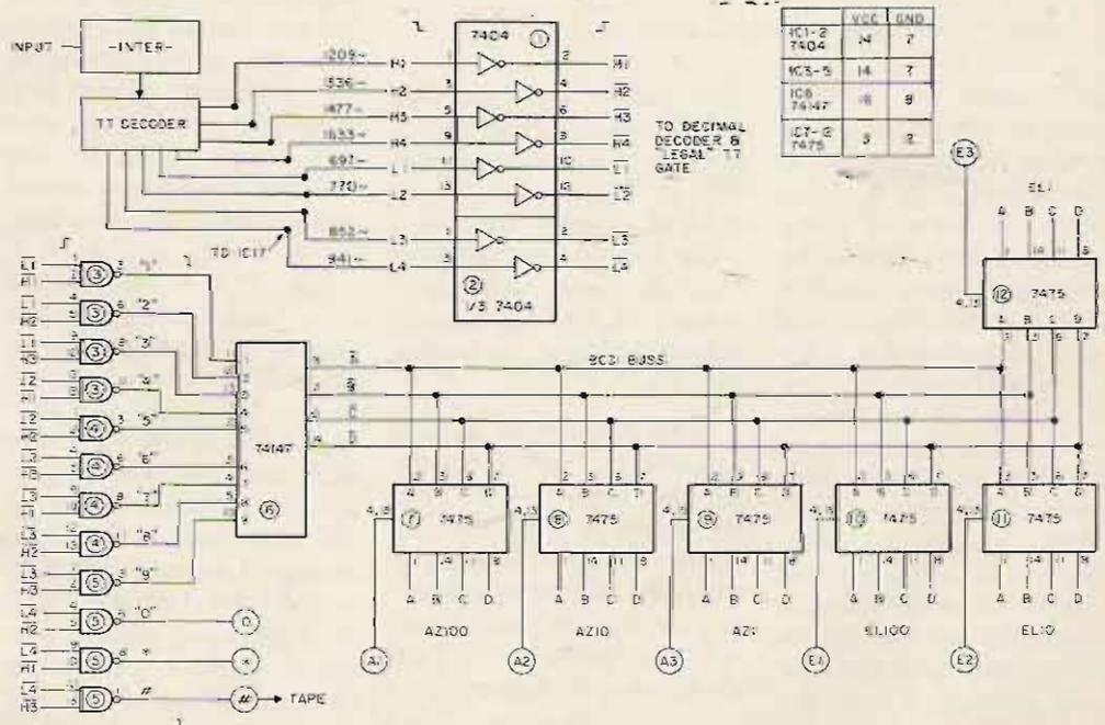
Fig. 2. Decode and store diagram.
