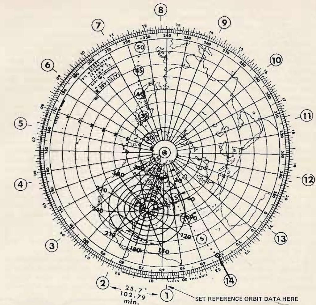
Fig. 13. Complete tracking system. Example: Reference orbit — 0032 GMT, longitude 57.2°. Set these values against index #1. We want to track AO-D during 14th orbit. Under index #14, we read EQX data: time 2247 GMT, longitude 31.8°. Tracking: satellite AOS (acquisition of signal) 10 minutes after EQX, 90° azimuth. 15 minutes after EQX — azimuth 45°, elevation ≈ 8°. LOS (loss of signal) 20 minutes after EQX, 10° azimuth.
