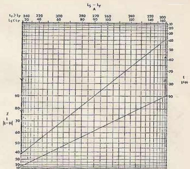
Fig. 5. ATS-3 worksheet. QTH is  $37^{\circ}$  N.,  $76^{\circ}$  W. Satellite is  $0^{\circ}$  N.,  $70^{\circ}$  W.  $L = 37^{\circ}$ ;  $L_S - L_Y = 70^{\circ} - 76^{\circ} = -6^{\circ} = 354^{\circ}$ ;  $Z \approx 37.5^{\circ}$ ;  $H = 90^{\circ} - Z = 52.5^{\circ}$ ;  $|L - H| = 15.5^{\circ}$ ;  $L + H = 89.5^{\circ}$ ;  $A \approx 167^{\circ}$  ( $168^{\circ}$  calculated);  $B$  (from table) =  $47.5^{\circ}$  ( $47.4^{\circ}$  calculated).
