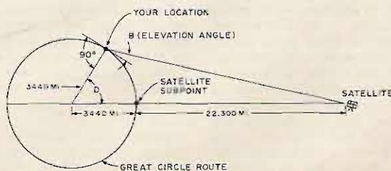
Fig. 2. Geometry used for calculating the elevation angle.
