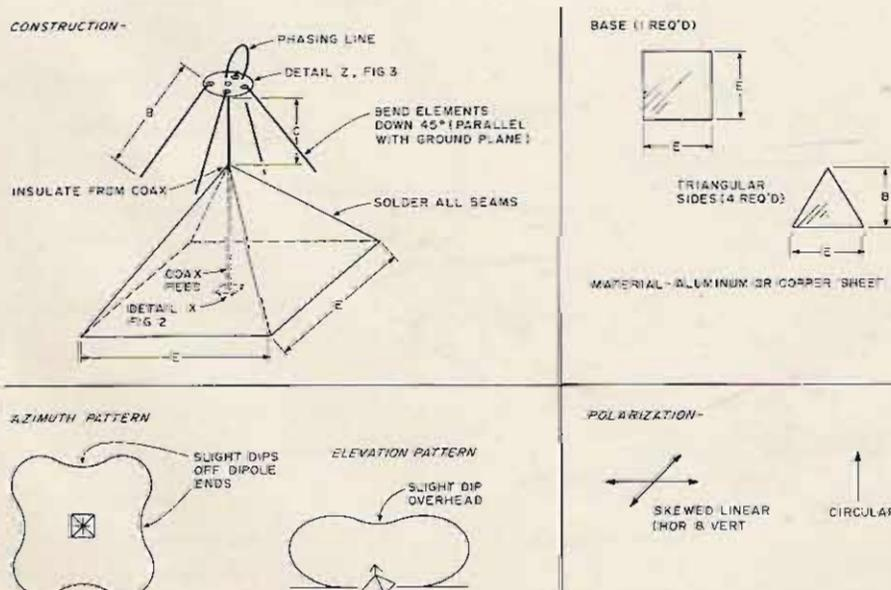
Fig. 4. Sloped turnstile over conformal ground plane.
