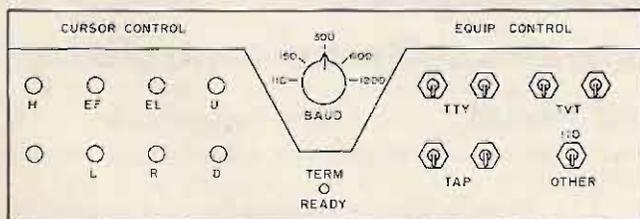
Fig. 1. Panel layout. H = home up cursor to start of page; EL = erase screen to end of line; EF = erase screen from cursor location on; U = move cursor up; D = move cursor down; L = move cursor left; and R = move cursor right.
