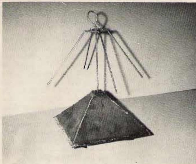
*Sloped turnstile over ground plane (432 MHz).*
