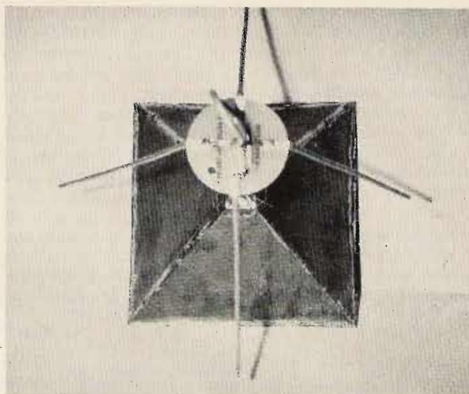
*Top view. Sloped turnstile over ground plane.*
