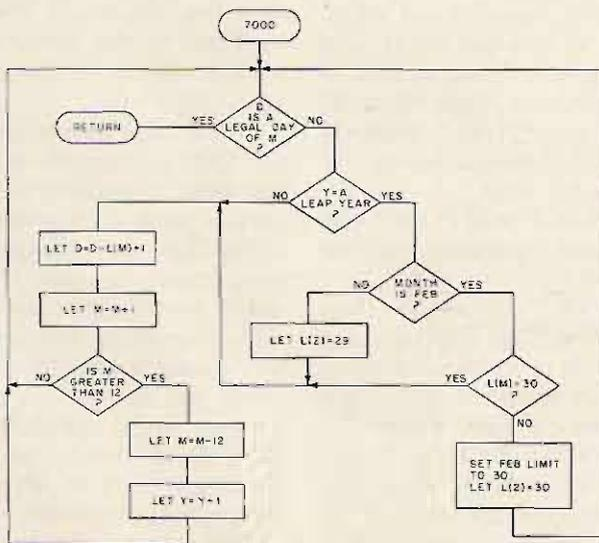
Fig. 6. Subroutine 7000, the calendar subroutine which takes care of advancing the month and year, when required. This subroutine also takes into account the possibility that the current year is a leap year and that, therefore, February must have 29 days instead of the usual 28.
