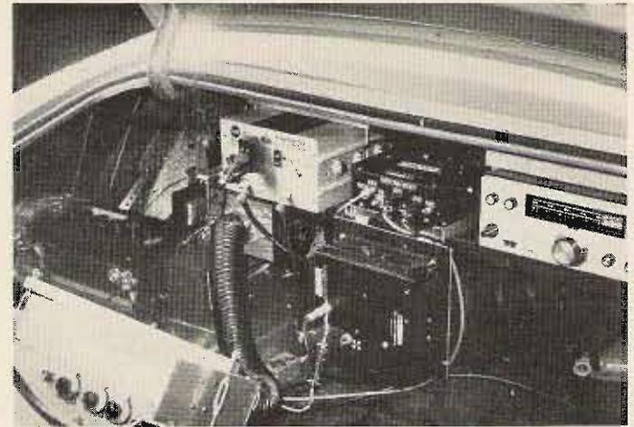
Power amp on 432 as in Fig. 3. There are 2 power supplies — 12 V dc to 300 V dc and 12 V dc to 1600 V dc — and a 12 V to 115 V ac converter. That's a lot of equipment to generate a 100 Watt plus SSB signal on 432.150.
