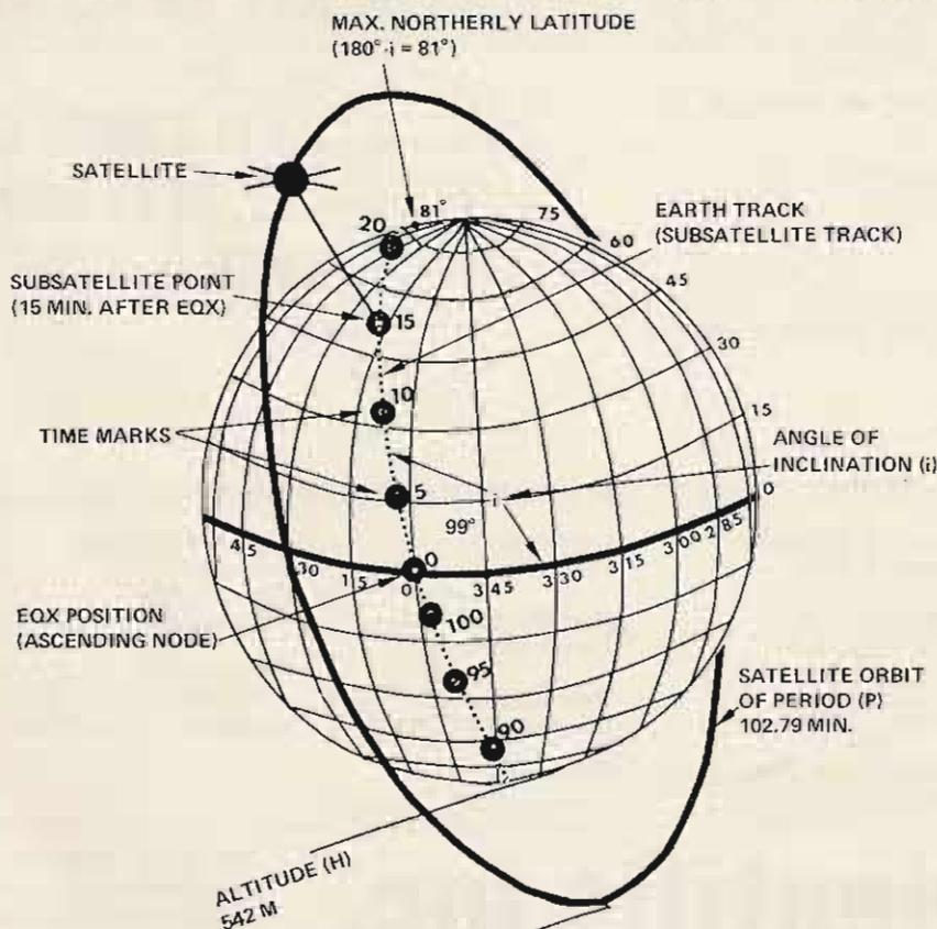
Fig. 2. Model of orbiting satellite (static Earth).
