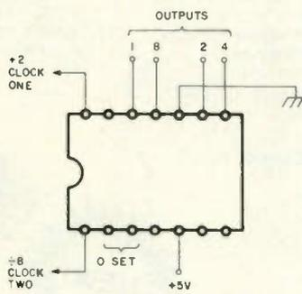
Fig. 3. 7493 binary counter pinout.
