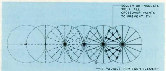
Fig. 8. Radial system shown in full for first two elements on the right. The other six are identical.
