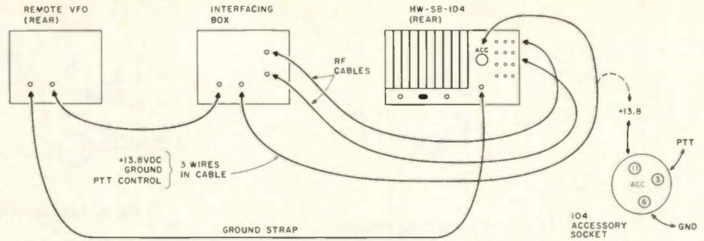
Fig. 2. Interfacing cable layout.
