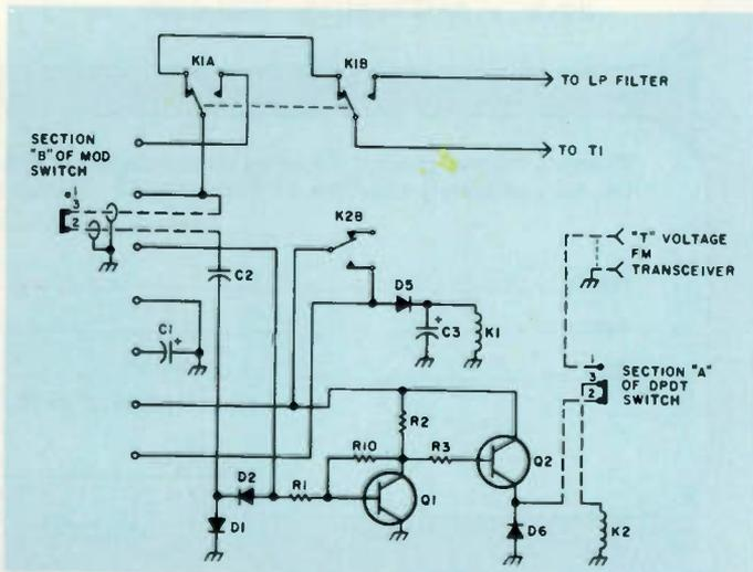
Fig. 1. Schematic of COR circuit showing modification for PTT switch. Leads from B section of DPDT switch are miniature 50-Ohm coax with shield grounded at switch end only.
