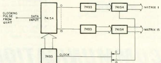
Fig. 8. Banking matrix using a 74154.
