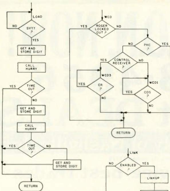
Fig. 4. Load, wait for carrier drop, link, tape, and selective call routines.
