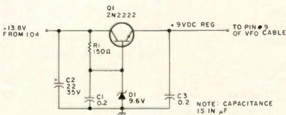
Fig. 3. 9 V dc regulated power supply.
