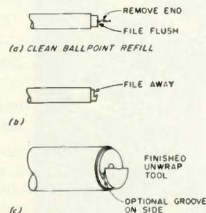
Fig. 2. Unwrap tool construction.
