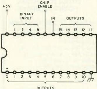
Fig. 2. 74154 data distributor pinout.
