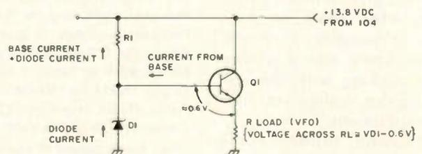
Fig. 4. Power supply simplified circuit.
