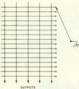
Fig. 1. Mechanical matrix selection.
