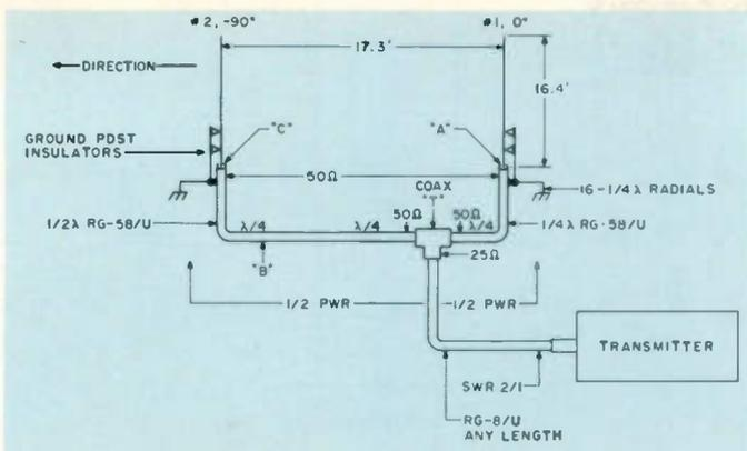
Fig. 1. Method of feed for the 2-element phased array.
