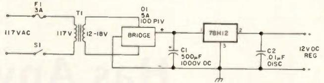
Fig. 1. Power supply schematic.
