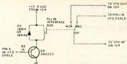
Fig. 6. Interface relay switching circuit.
