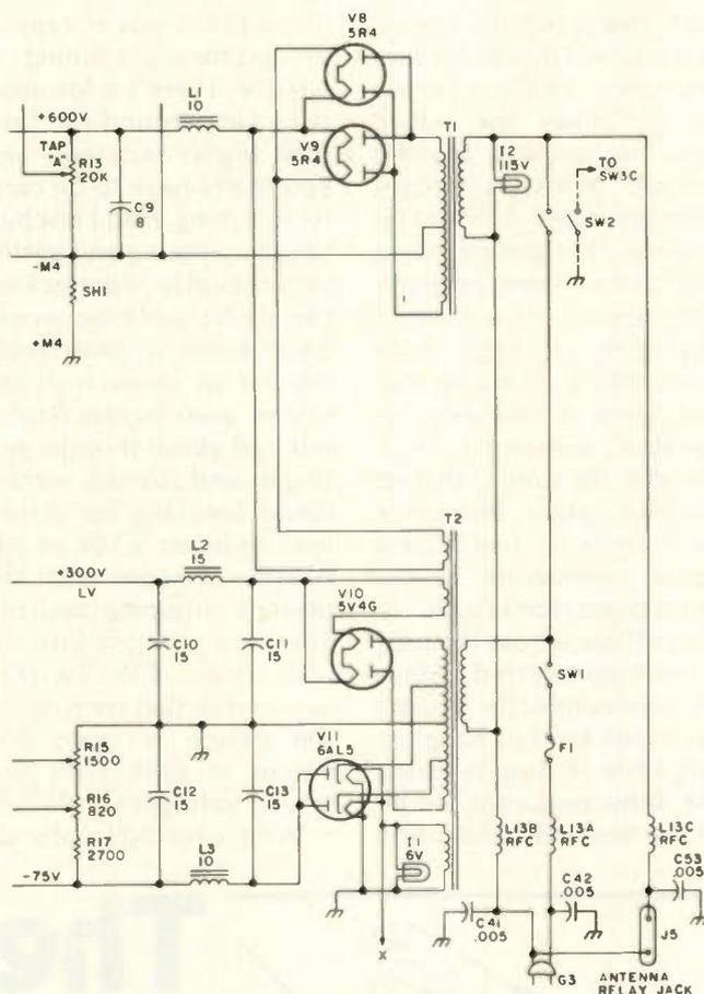
Fig. 1. Original Viking power supply diagram.
