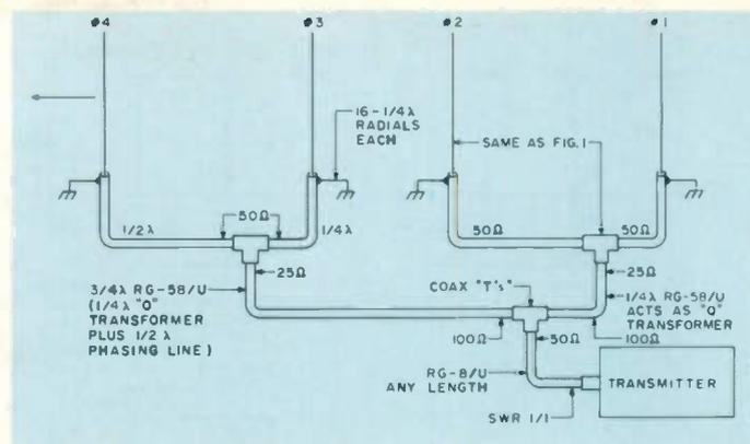
Fig. 2. Method of phasing and power division for the 4-element array.
