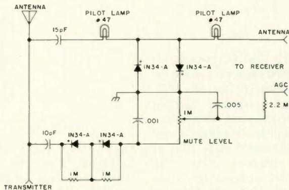
Fig. 1. Poor man's T-R switch schematic diagram.
