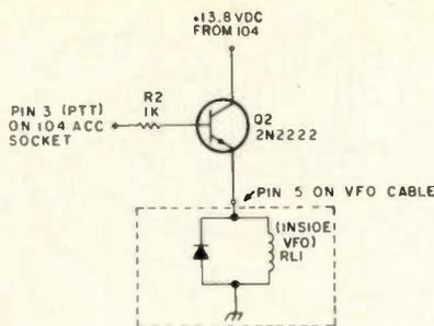
Fig. 5. Vfo relay switching circuit.
