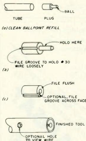
Fig. 1. Wire-wrap tool construction.
