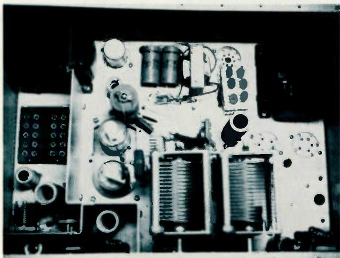
rent through an inductor causes a back electromotive force (emf). The back emf tends to oppose the change in voltage trying to take place, with the net effect that one tends to cancel the other, particularly when load demands change, as in modulation. So, instead of a changing voltage at the rectifier output (a ripple), you get a smoother dc voltage, which is why it's called a smoothing choke.
