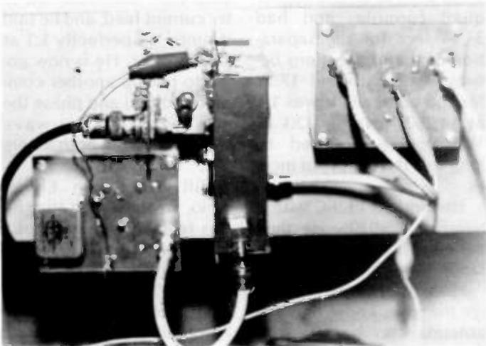
Photo C. From left to right: the oscillator, active mixer, and preamp.
