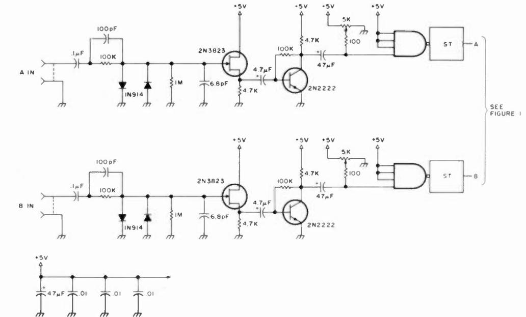
Fig. 2. Signal conditioner part of main board.
