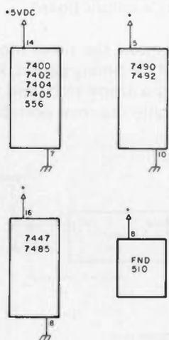
Fig. 4. Supply connections.
