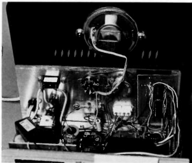
Interior view of the timer showing the speaker mounted on the top of the cabinet. The power supply components and 115 V ac connections are shown on the left side. The small board at the right was added after the project had been designed and the main circuit board etched. With better planning, the 2 ICs could have been mounted on the main board.
