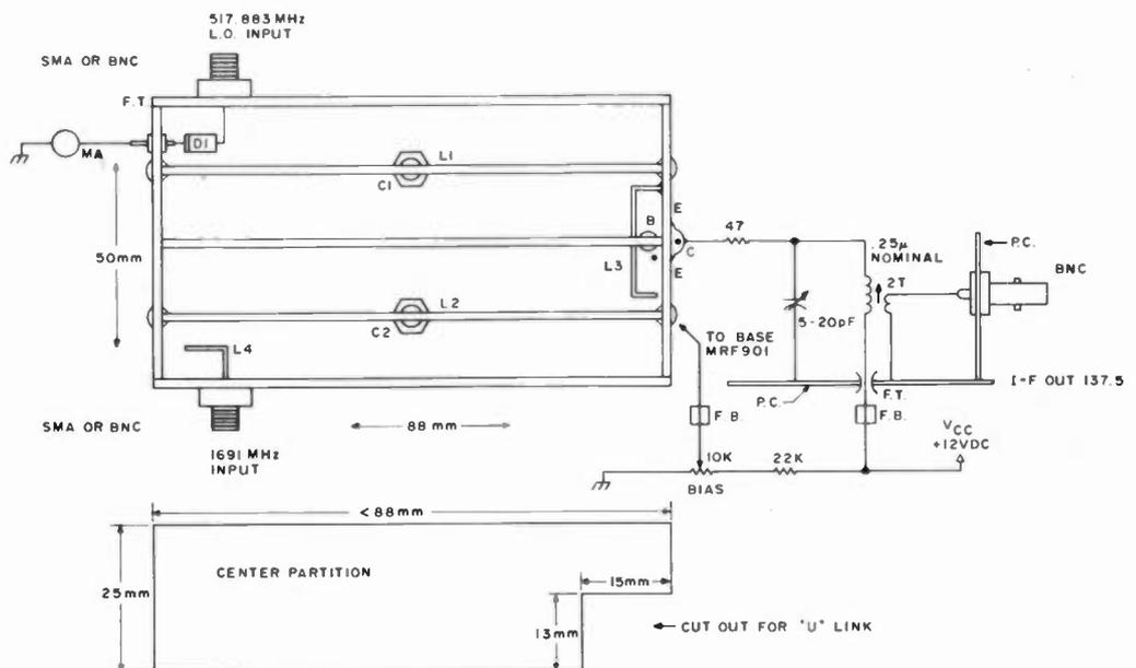
Fig. 2. Schematic of the active mixer. L1, L2—#10 wire; C1, C2—10-32 nuts and bolts; L3—20 mm x 14 mm U-shaped link, #14 wire; L4—12 mm x 7 mm x 2 mm tab.
