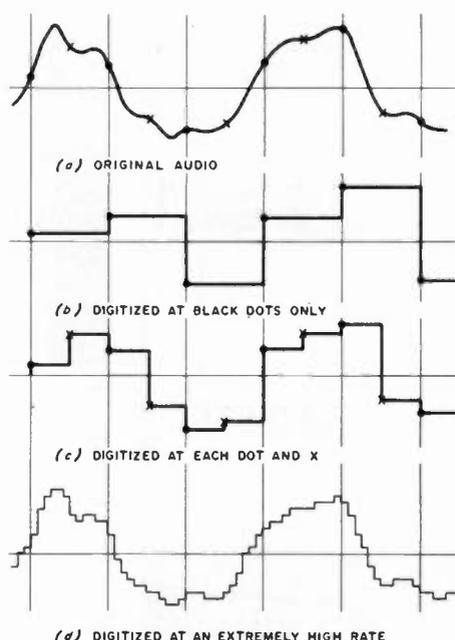
Fig. 1. Digitizing audio at various sampling rates.
