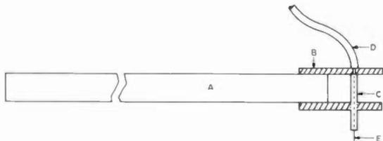
Fig. 4. Stylus holder details. (A) 3-1/4" piece of 1/4" steel rod stock (left over after the drum shaft has been cut to size). (B) 3/4" piece of 3/8" o.d. plastic tube stock. (C) 1/2" piece of 1/16" tube stock (stylus holder). (D) length of hookup wire soldered to one end of (C). (E) Wire stylus inserted into (C).
