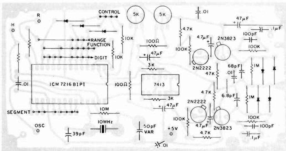
Fig. 6(b). Component layout, main counter board.
