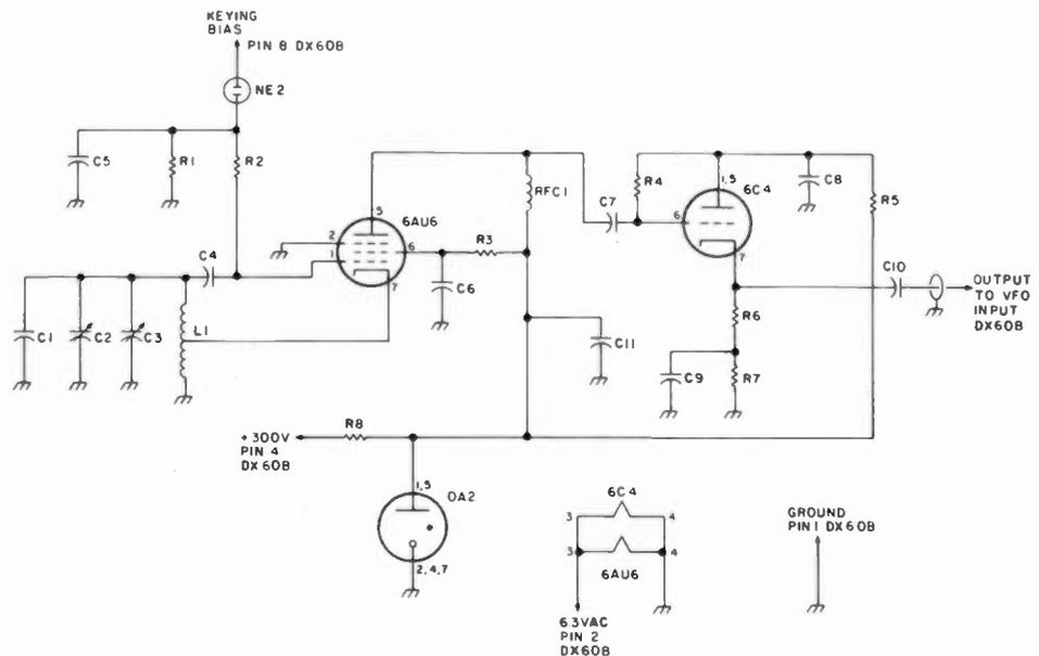
Fig. 1. Vfo schematic.
