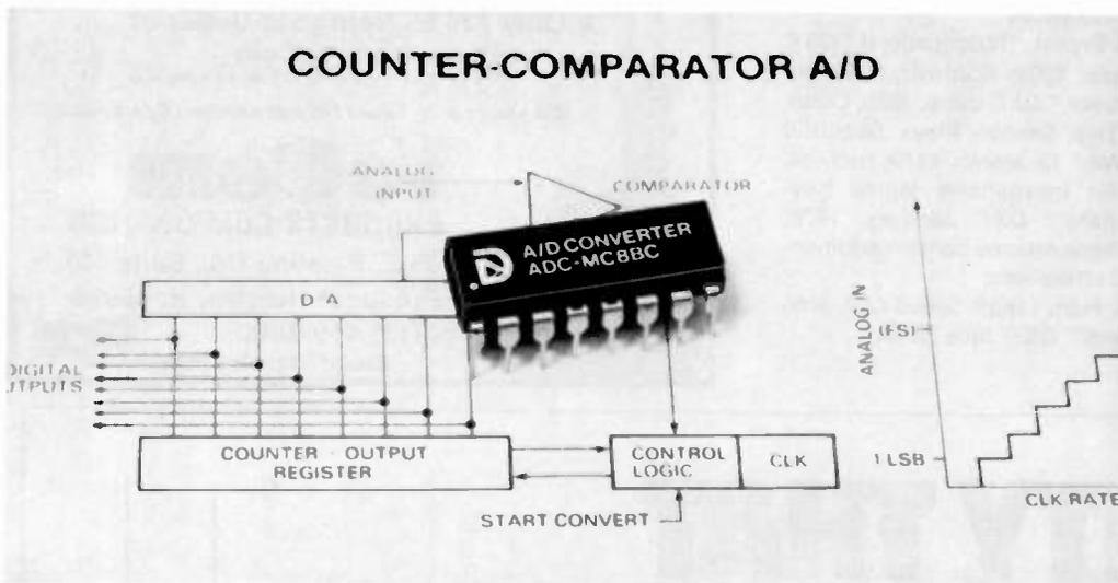
Photo A. A good, low-cost 8-bit A/D made by Datal. Its output coding is in binary, it runs off 5 volts, and it has a conversion time of only 500  $\mu$ s. Its current selling price is about \$8.00. (Photo courtesy of Datal)
