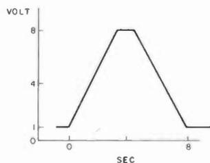
Fig. 2. Waveform from square-wave generator and R1C1 integrator.
