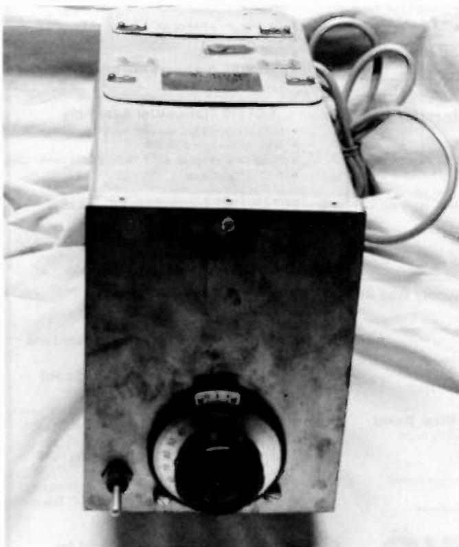
Photo A. Front view of the vfo showing use of the ARC-5 cabinet. The front is covered by a copperclad plate for appearance's sake and for dial mounting.
