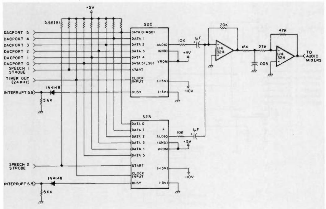
Fig. 1. Speech synthesizer hardware interface to microcomputer.
