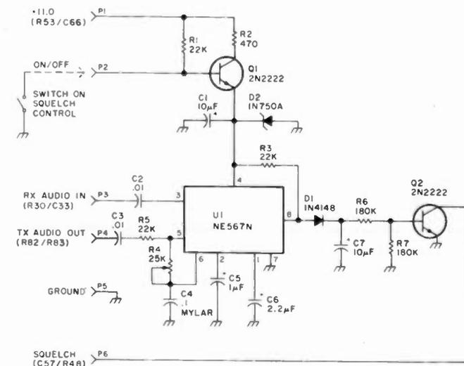
Fig. 1. Single-tone encoder-decoder for the Wilson MK II/IV.
