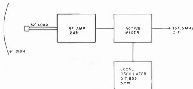
Fig. 1. System configuration for the active-mixer converter.
