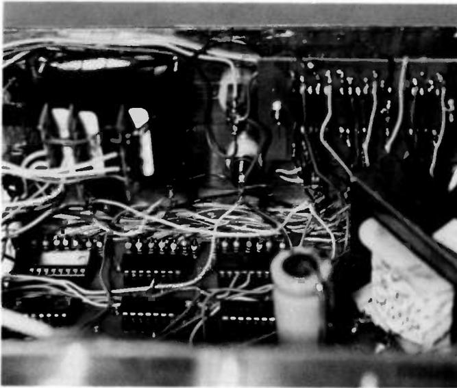
Interior view showing the inside of the front panel and part of the main circuit board. Displays are upper right; thumb-wheel switches are at the left. The 7447 display drivers and segment current-limiting resistors are in the lower center. Below them are the 7490 and 7492 decoders. The unorthodox wire connections to two of the drivers were added to correct errors on the circuit board. Because of omitted foil connections, wires were forced into the sockets beside IC pins.
