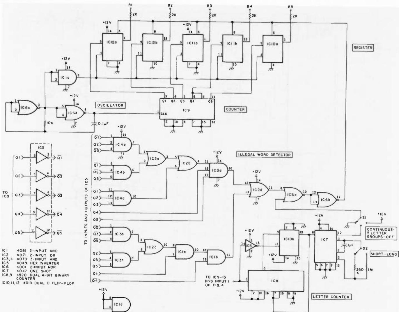
Fig. 3. The electronics of the Instructor. Not all connections are shown to avoid confusion in the diagram. All points labeled Q1 to Q5 are connected together. Similarly, all those labeled Q1 to Q5 are connected together. All unused CMOS gates are tied to 12 volts.
