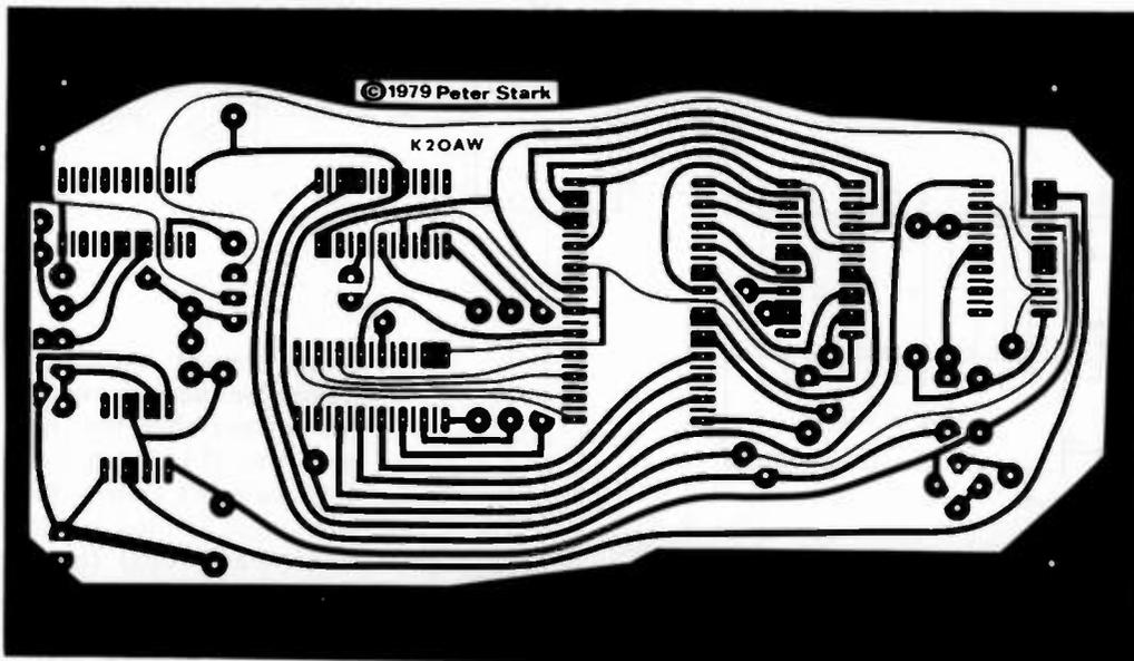
Fig. 4. PC board, copper side.
