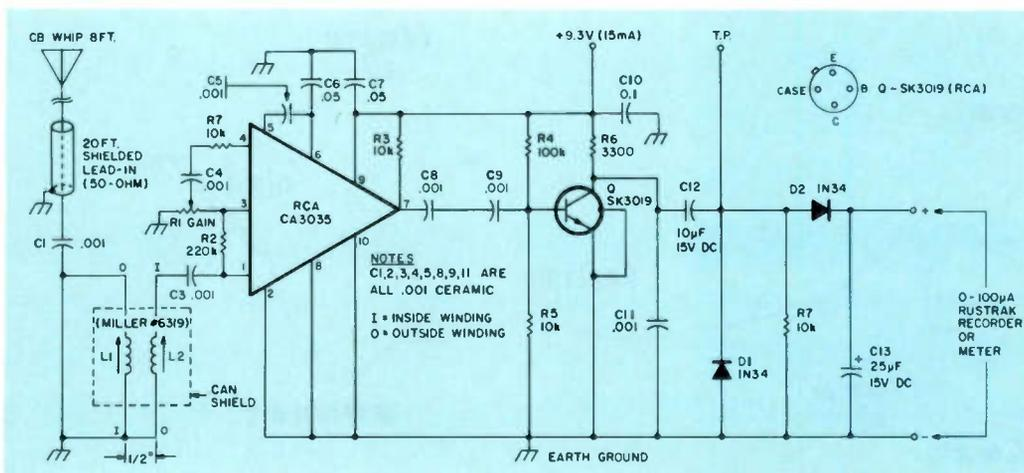
Fig. 2. Circuit for a tunable SES receiver.
