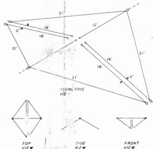
Fig. 2. Final configuration of the attic antenna.
