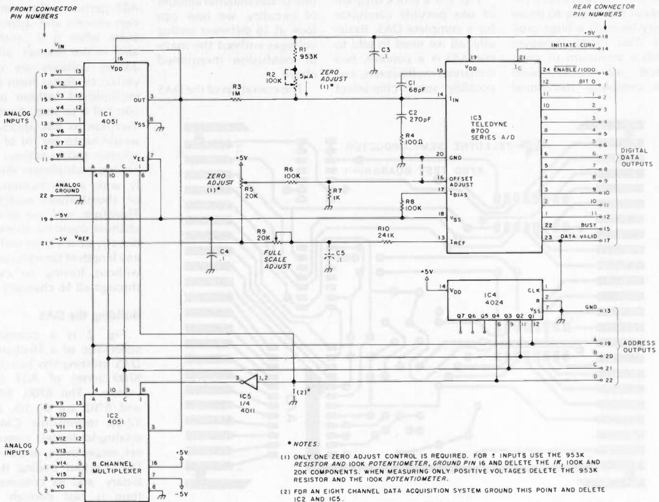
Fig. 2. The complete schematic for the 16-channel DAS utilizing the Teledyne 8700 series of A/D converters.
