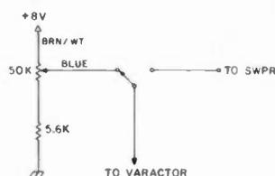
Fig. 4. Hookup using toggle switch.
