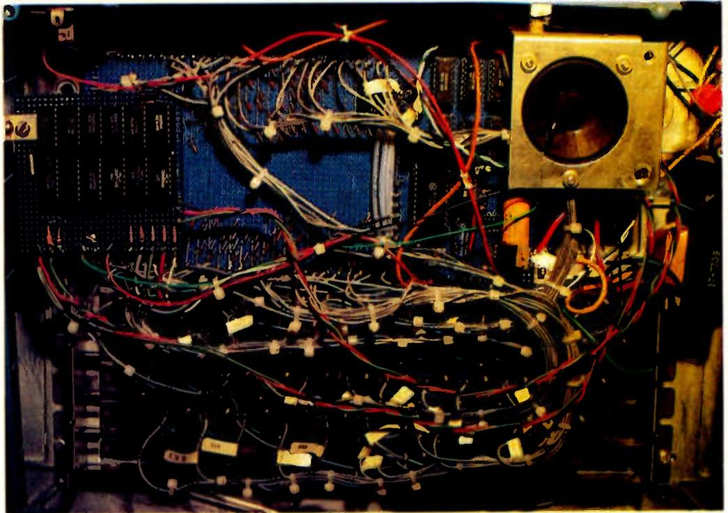
*Photo B. Perfboard and wire-wrap sockets are used for the two electronic boards. The diode matrix and keyer are on the lower board. The Instructor electronics are on the smaller board on the left, partially obscuring the diode matrix.*
