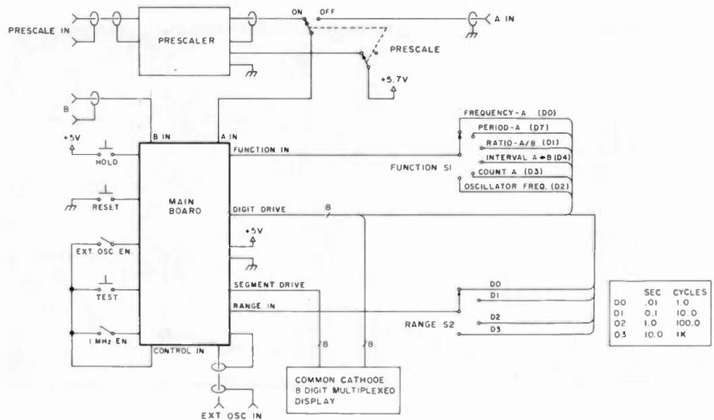
Fig. 3. External connections.
