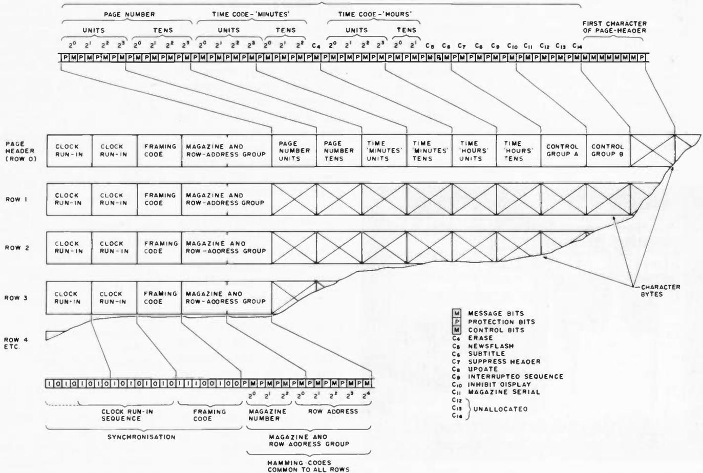
Fig. 1. Transmission format for British teletext.
