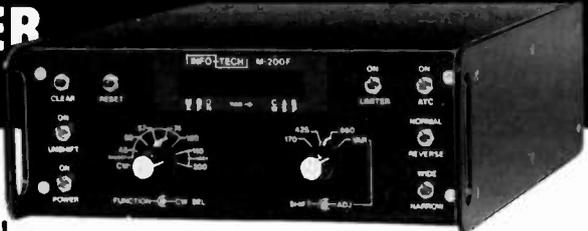
Converts Morse & RTTY (Baudot & ASCII) to video, and serial Baudot or ASCII for hard copy
