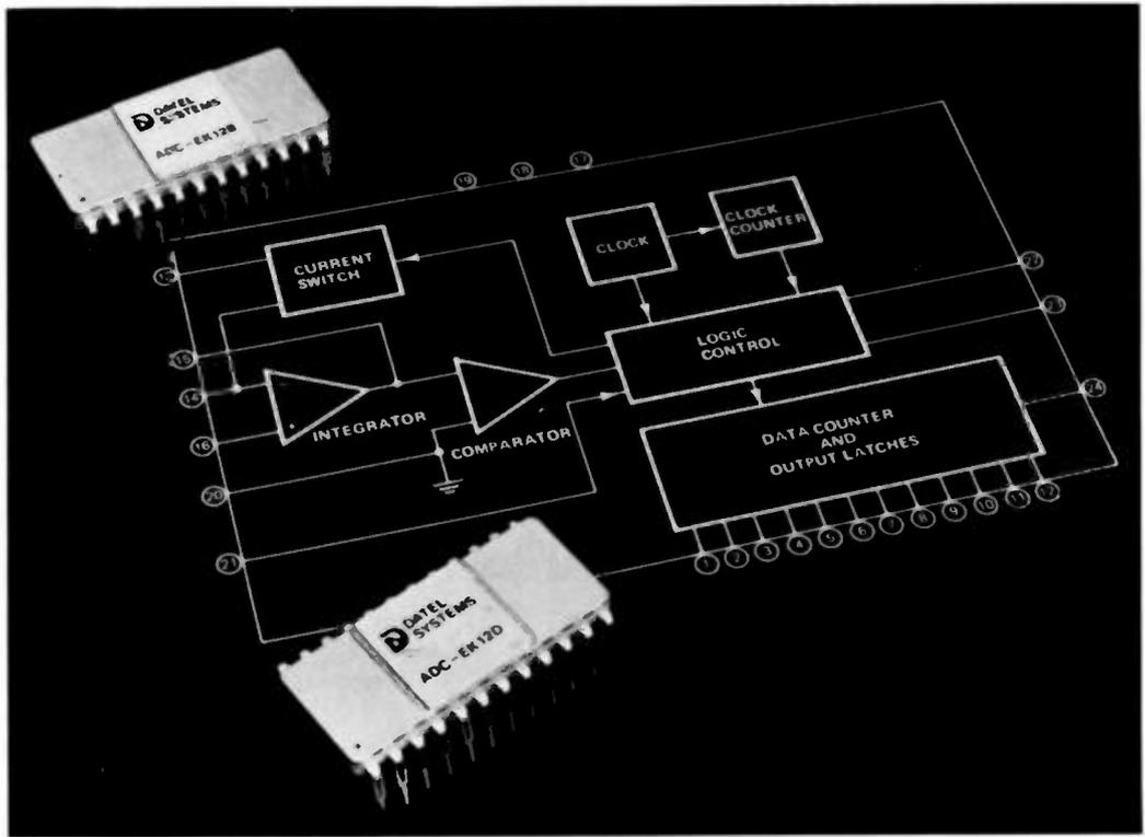
Photo B. Another Datel device which is a bit more expensive (\$34.00). It is a 12-bit binary or 3½-digit BCD coded A/D converter, and it runs off ±5 volts and has a 20-ms conversion time. (Photo courtesy of Datel)
