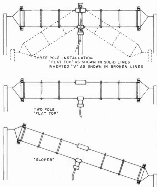
Fig. 1. Typical installations for B&W's 370-15 allband folded dipole.
