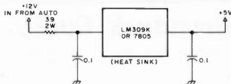
Fig. 6. Voltage regulator for mobile use.
