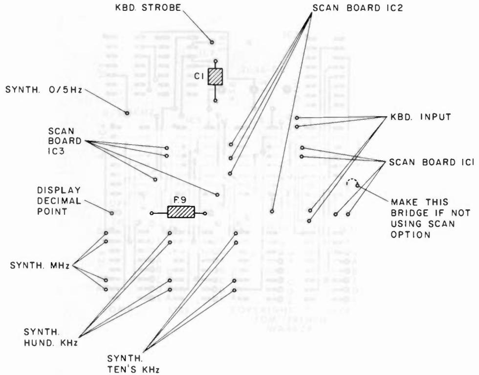
Fig. 2. 2036 Display Board connections.
