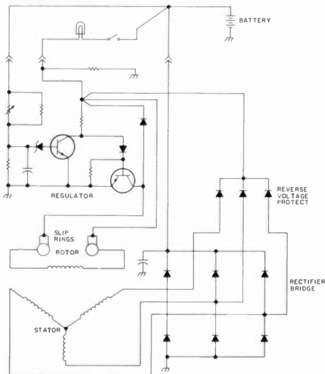
Fig. 1. The charging system for late-model GM cars.
