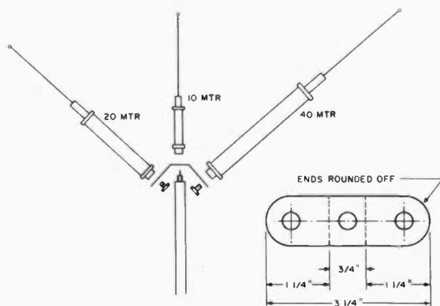
Fig. 1. Four-band mobile antenna construction details.
