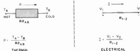
Fig. 1. The electrical analog of heat transfer.
