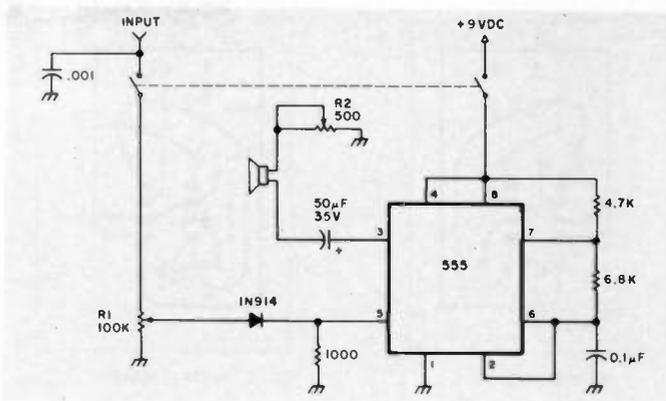
Fig. 2. Voltage-to-frequency converter schematic.
