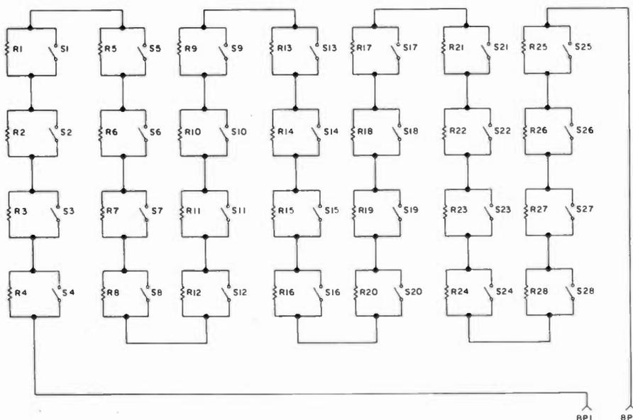
Fig. 1. Schematic for resistor substitution box.
