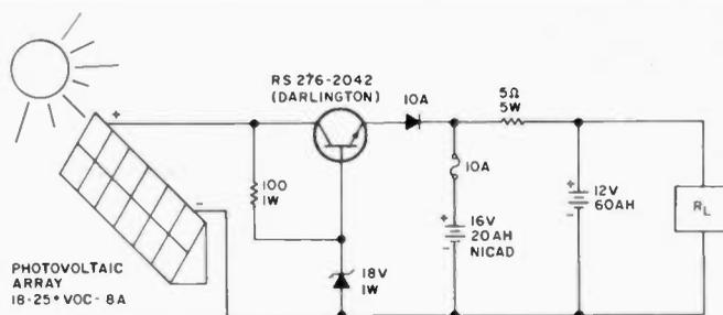
Fig. 2. Power conditioning and storage circuit.
