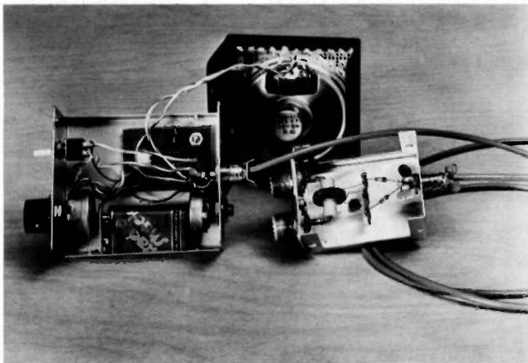
Photo B. Assembly details. Voltage-to-frequency converter is on left, rf coupler is on right.
