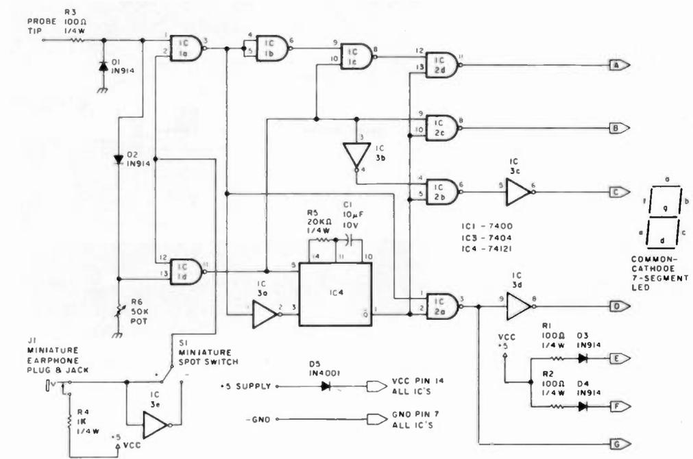
Fig. 1. Schematic diagram of the Synchronized Logic Probe.
