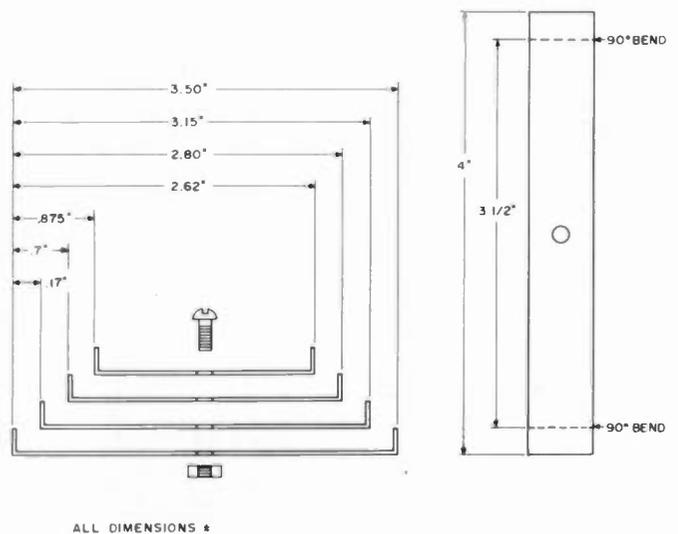
Fig. 2. Heat sink construction details.
