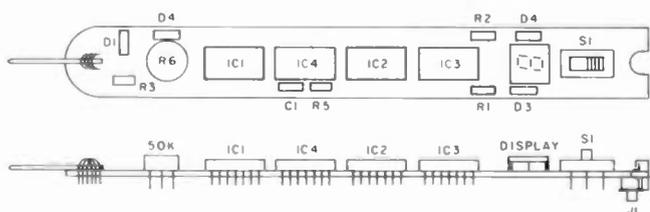
Fig. 3. Synchronized Logic Probe component mounting.
