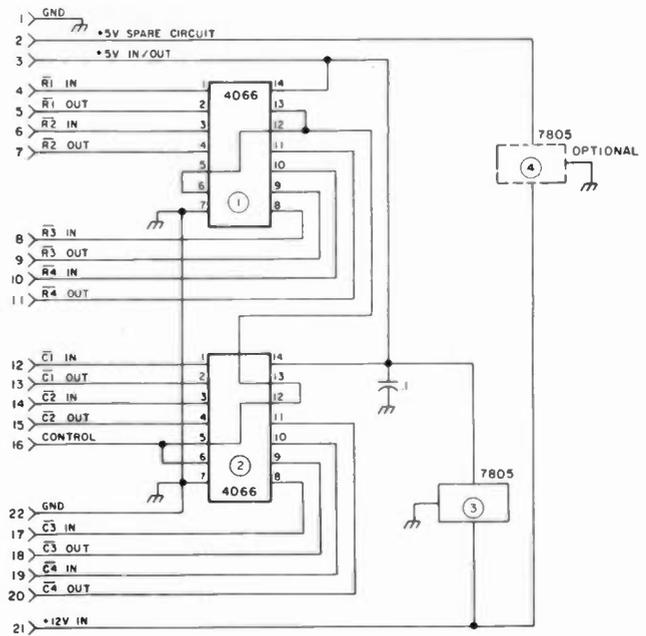
Fig. 6. Row/column switch and regulator board.
