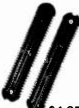
Rugged, lightweight, injection molded of top quality material, with high dielectric qualities and excellent weatherability. End insulators are constructed in a spiral unending fashion to permit winding of loading coils or partial winding for tuned traps.
