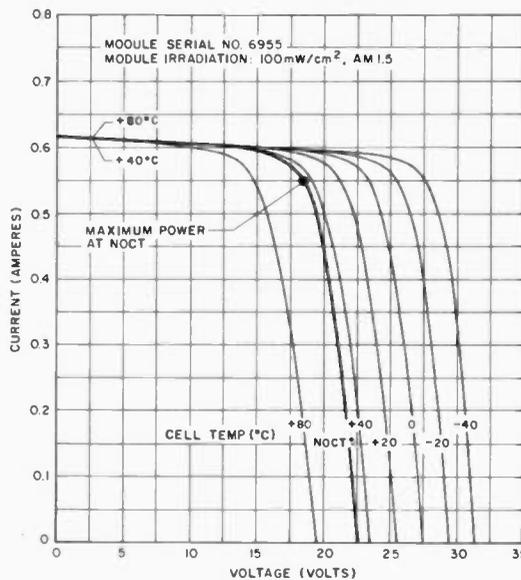
Fig. 3. Specifications of photovoltaic array.
