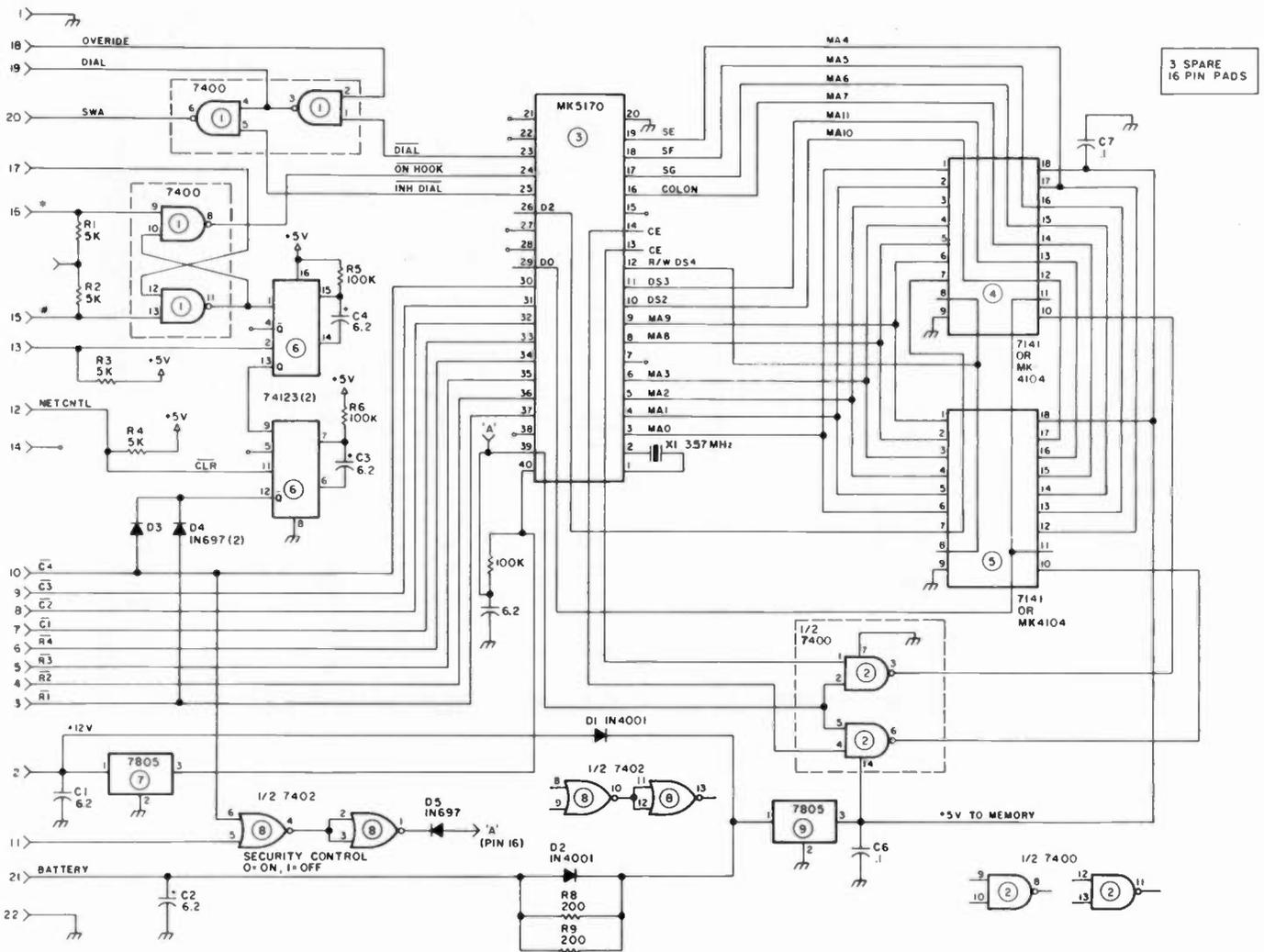
Fig. 2. Circuit diagram for the 100-number system.
