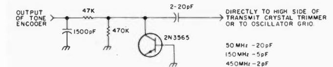
Fig. 2. Schematic of a typical varactor assembly. The collector-base junction of an NPN transistor is used as the varactor. The output of the assembly is connected to the high side of the transmit crystal trimmer. In a tube-type transmitter, the output is often connected to the grid of the oscillator tube. The value of the coupling capacitor changes, depending on the frequency range used. The values shown are approximate and may require adjustment to obtain the proper deviation level.
