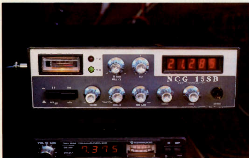
The NCG-15 15-meter monoband transceiver.
