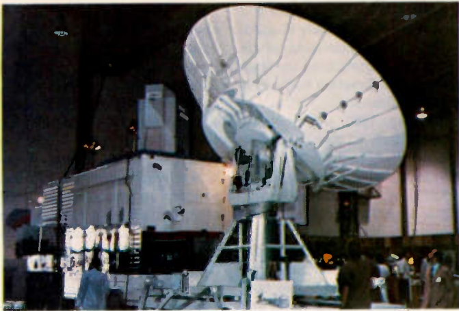
This is a complete mobile television studio capable of directly feeding a satellite from any location.
