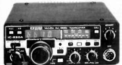
**IC-290A** All Mode 2m mobile. 143.8-148.199 Mhz, 1 or 10 watts. RIT, prog. offsets, 5 memories, 2 VFOs, 2 scanning systems, SSB squelch, priority channel, sidetone, blanker, memory retention provision, T/T microphone. 6 3/4" w x 2 1/2" h x 8 3/4" d. Regular \$549.00
