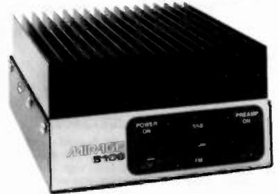
**MIRAGE B-108** Solid State VHF Power Amplifier with built-in switchable 10db gain/2.5db N.F. receive preamplifier. For 144-148 MHz, 5-15w in/80w out @ 10w. Operates with as little as 1w; 1-2w in gives 15-30w out. Linear, for FM, CW and SSB with external or automatic internal relay keying with adjustable delay. Size: 5 $\frac{1}{2}$ "w x 3"h x 8"d. Wt. 3 lbs. Requires 13.6 Vdc @ 10-12 Amps.
