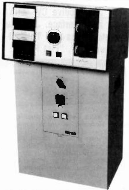
**HENRY 2K Classic** 80-15m Linear Amplifier. 2000 watts PEP SSB - 1000 watts CW, RTTY & AM. Two Eimac 3-500Zs, 80-150 watts drive, tuned input. ALC circuit, heavy duty power supply, fully metered, air cooled, built-in antenna relay. Size: 32 $\frac{3}{4}$ "h x 16 $\frac{1}{2}$ "w x 15"d. Wt. 125 lbs.
