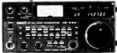
**IC-720A** Solid state, digital HF Transceiver. 9 HF Ham bands, receives .1 to 30 Mhz. 100w output, cont. LED readout, 2 VFO's, AM, CW, SSB & RTTY filters. PBT, RIT, VOX, semi break-in, blanker & processor. 13.5v/20A 4 1/2" h x 9" w x 12 1/2" d, 17 lbs. Regular \$1349.00
