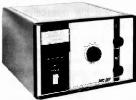
**HENRY 1KD-5** 80-15m Linear Amplifier 1200w PEP input, 700w PEP nominal output. Single Eimac 3-500Z, tuned input. ALC, conservative rated power supply, built-in antenna relay. Size: 8 $\frac{3}{4}$ "h x 14"w x 15"d, 48 lbs.
