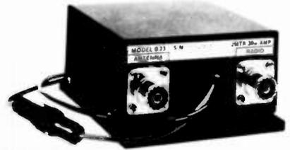
**MIRAGE B-23** All mode Solid State VHF Power Amplifier for Hand-helds & low power FM/SSB transceivers. For 144 to 148 MHz, 100mw to 5w in/30w out @ 2w, RF relay. Size: 4 $\frac{1}{4}$ "w x 2 $\frac{1}{4}$ "h x 2 $\frac{1}{4}$ "d. Wt. 1 $\frac{1}{4}$  lbs. 13.6 Vdc @ 5 Amps.
