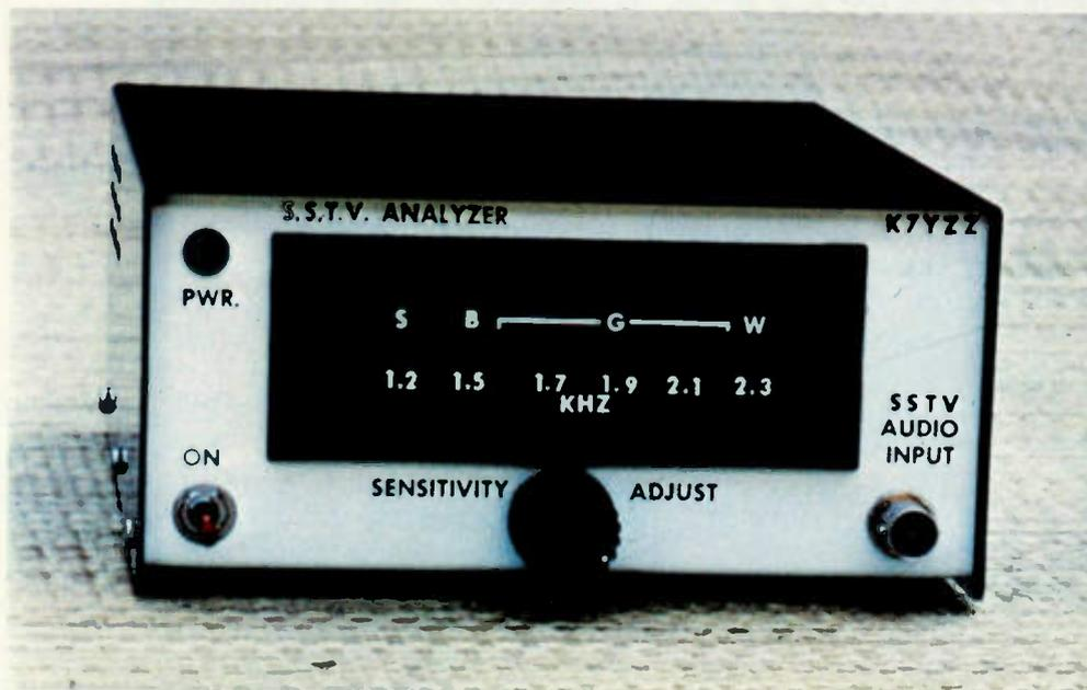
*The completed SSTV audio signal analyzer.*
