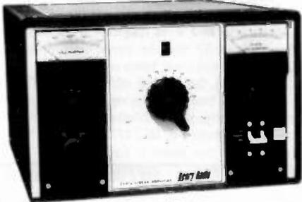
**HENRY 2KD-5** 80-15m Linear Amplifier. 2000 watts PEP input, 1200w PEP nominal output on SSB, 1000 watts CW, RTTY & AM. Two Eimac 3-500Zs, 100 watts drive, tuned input. ALC, heavy-duty power supply, full metering, built-in antenna relay. Size: 10 $\frac{1}{2}$ "h x 15"w x 17 $\frac{1}{2}$ "d. Wt. 62 lbs.
